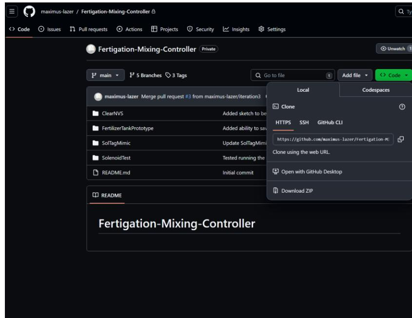
4. In the “Fertilizer-Mixing-Controller-main” folder, open the “FertilizerTankPrototype” subfolder. The file FertilizerTank.ino is the code that is running on the Arduino Nano ESP 32. Open this file in the Arduino IDE.
