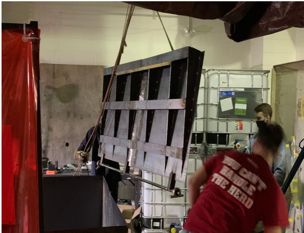
Figure 20: Paddle after assembly, being hoisted by a gantry into the tank
