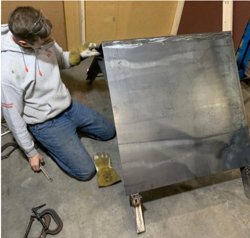
Figure 15: Sawhorse style jig to ensure right angle joints between panels.
