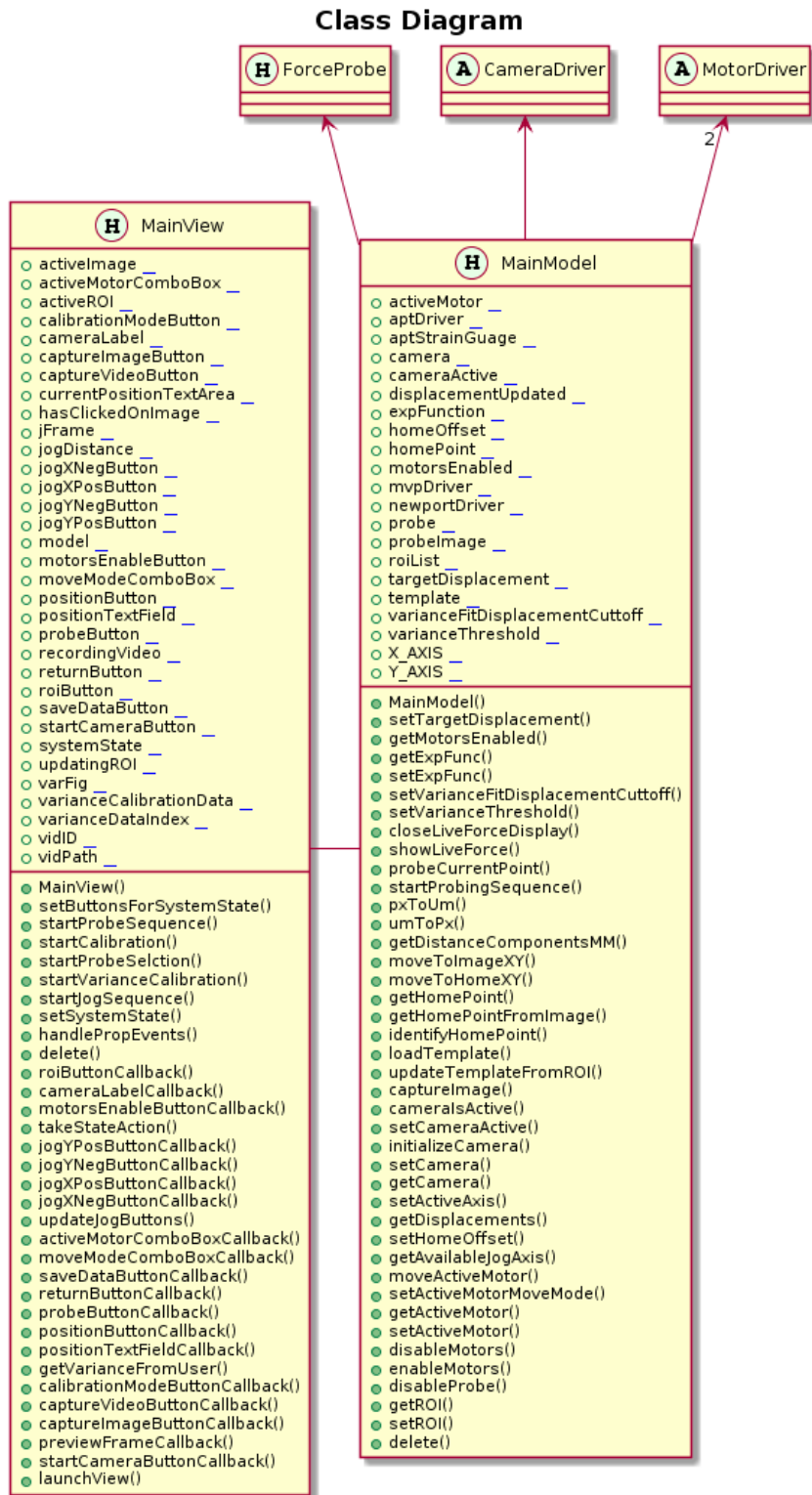
Figure 41. Part 2 of a UML class diagram for the MATLAB software. Shows the primary control and display classes
