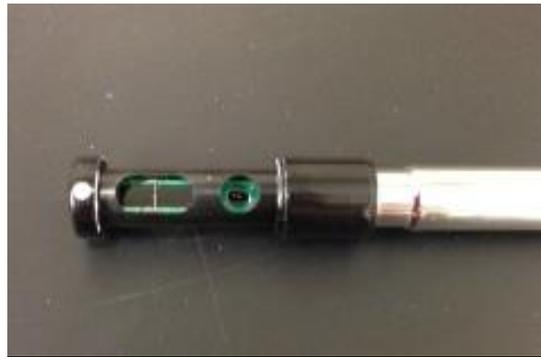
*Figure 27: Close up of Anemometer Measuring Element*
