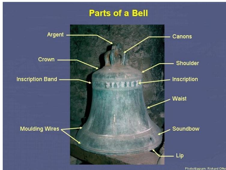
**Figure 8** Parts of a Bell
