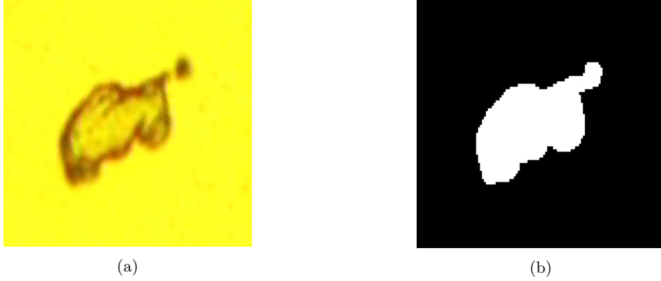
Figure 21: (a) Instance of porosity from labeled sample (b) Generated binary mask from instance.
