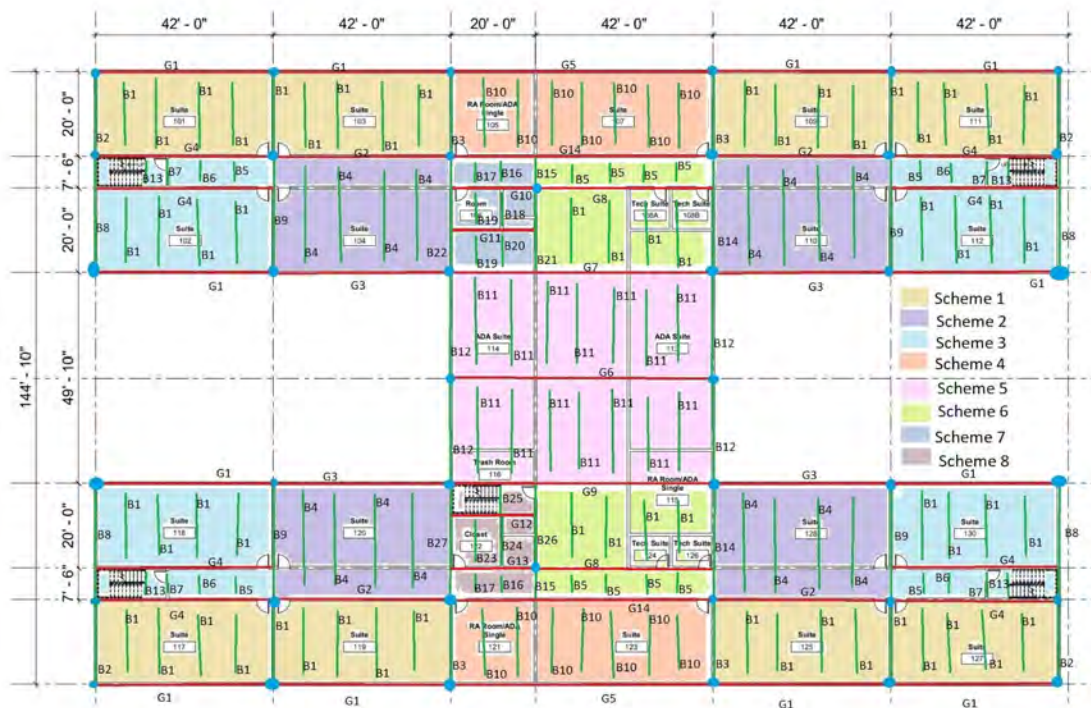
Figure 5: Basic Framing Scheme Layouts
