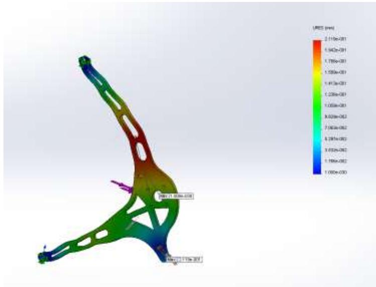
Figure 22: Maximum Deflection under Acceleration Load
