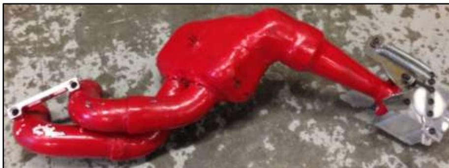
Figure 5 - 2012 FSAE Intake & Throttle Body
