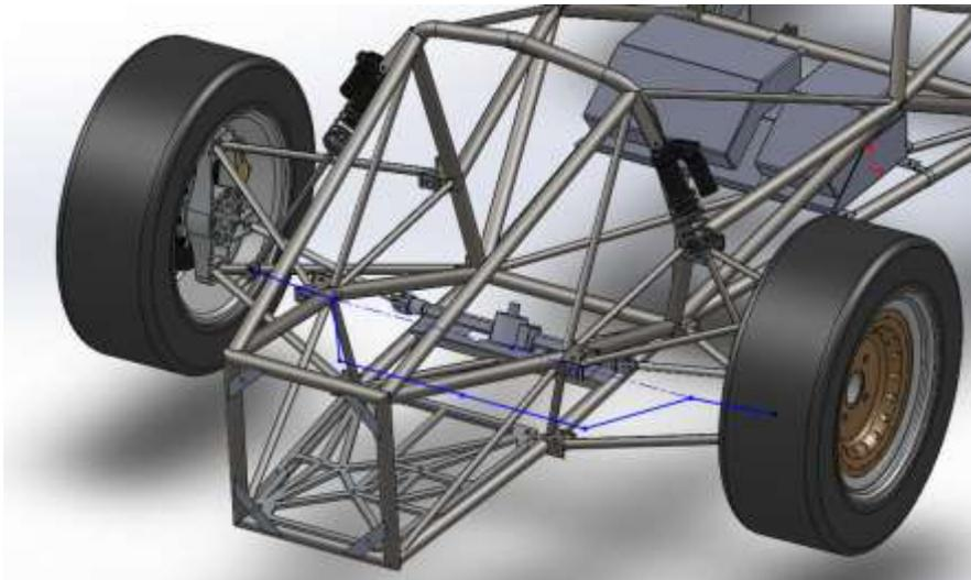
Figure 50 Initial Sketch for Sway Bar Positioning With Front Suspension
