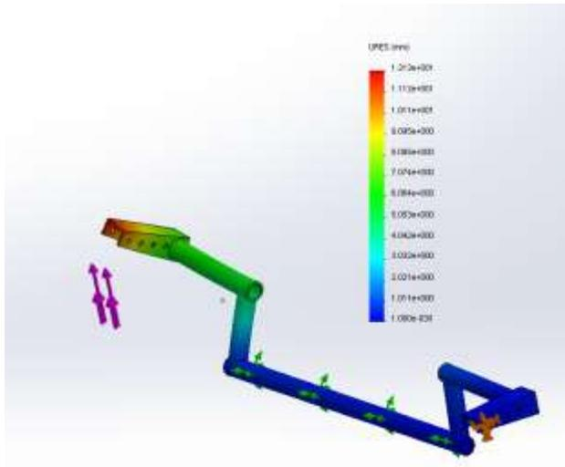
Figure 52 1.0" Sway Bar Displacement Analysis
