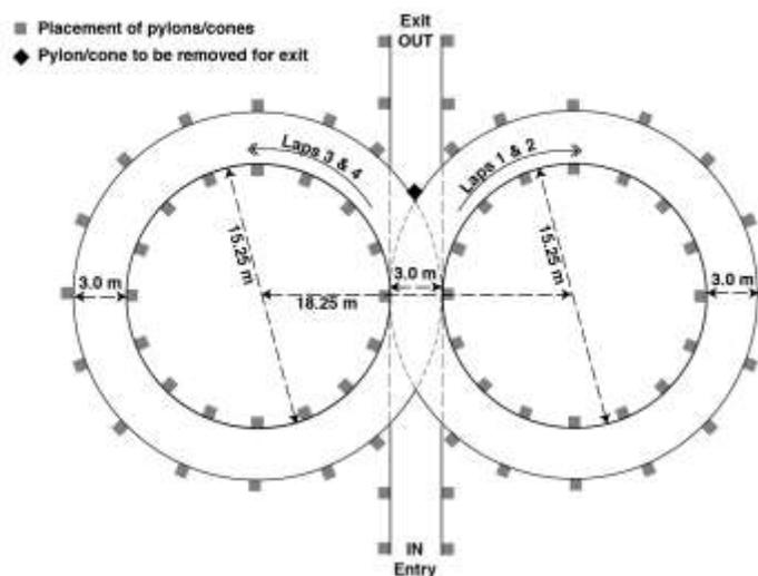
Figure 1: FSAE Skid-Pad Layout (2013 Formula SAE Rules)
