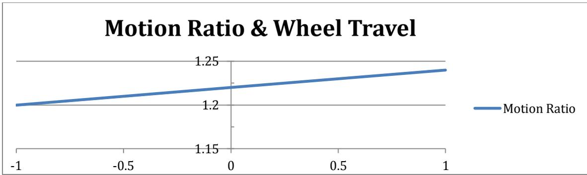
Figure 36: Motion Ratio Over Wheel Travel – Progressive & Approximately Linear
