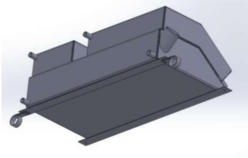
Figure 45: View of tank assembly showing mounting rails & clips
