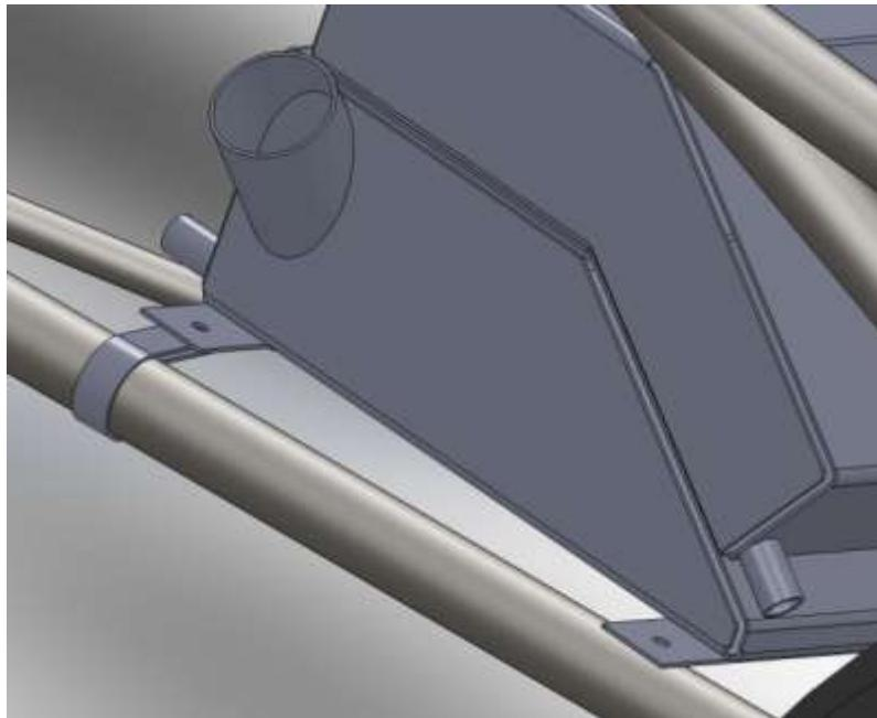
Figure 46: Tank assembly mounted to chassis members
