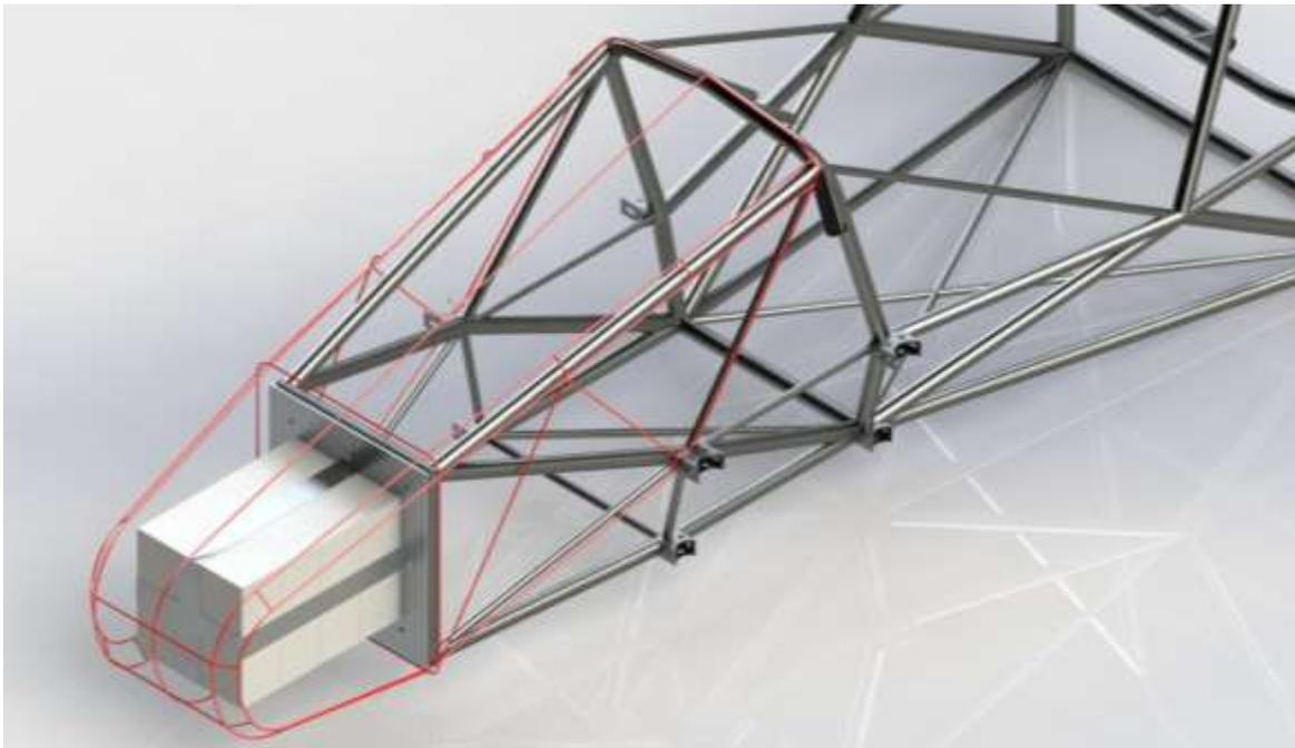
The other holes in the chassis frame not covered by this nose cone are separate from it for two reasons. First, their removal is not necessary during judging at competition. Therefore, they can be attached to the chassis separately. The convenient part about this is the fact that these connections can then be essentially be permanent ones, which are easier to accomplish.
