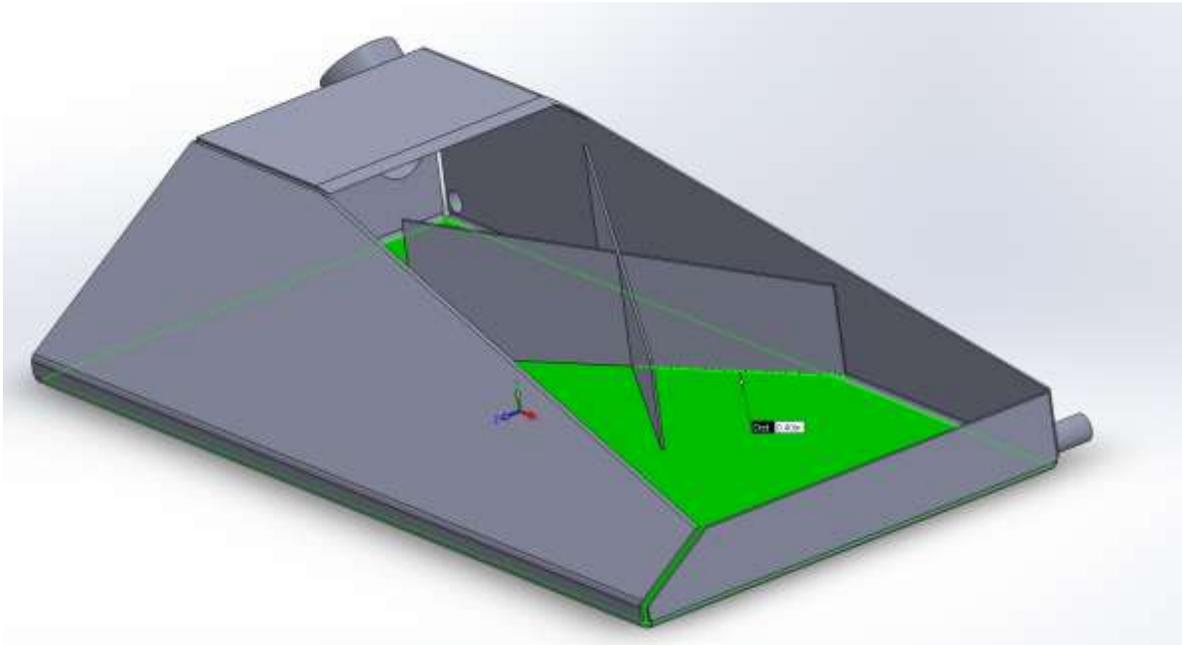
**Figure 43: Final Fuel Tank Design Sectioned to show baffling and clearance**
