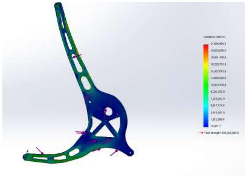
Figure 25: Max Stress under Torque Load
