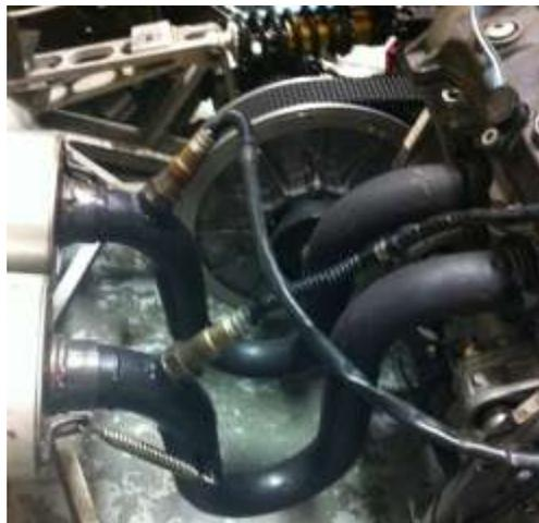
**Figure 9: Primary Exhausts on the 2012 FSAE Car**
