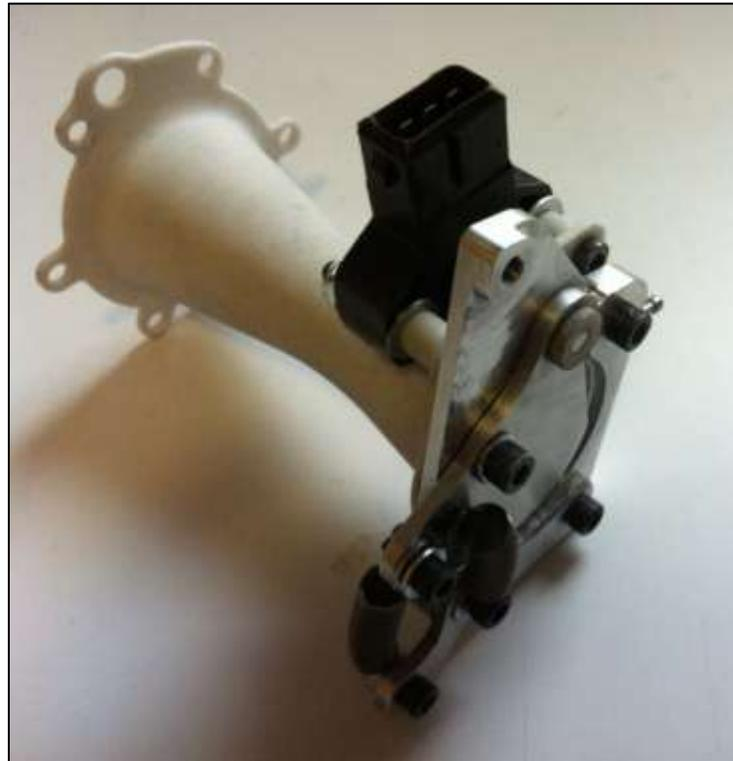
**Figure 7 - 2013 Throttle Body and Restrictor**
