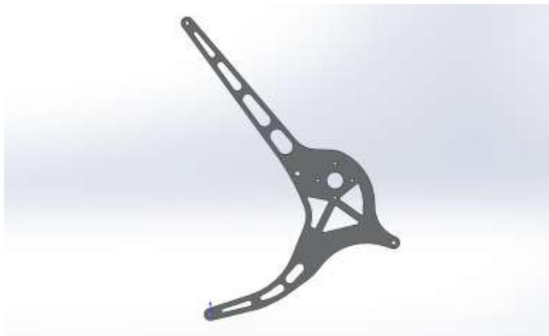
**Figure 16: Left Engine Mount**
