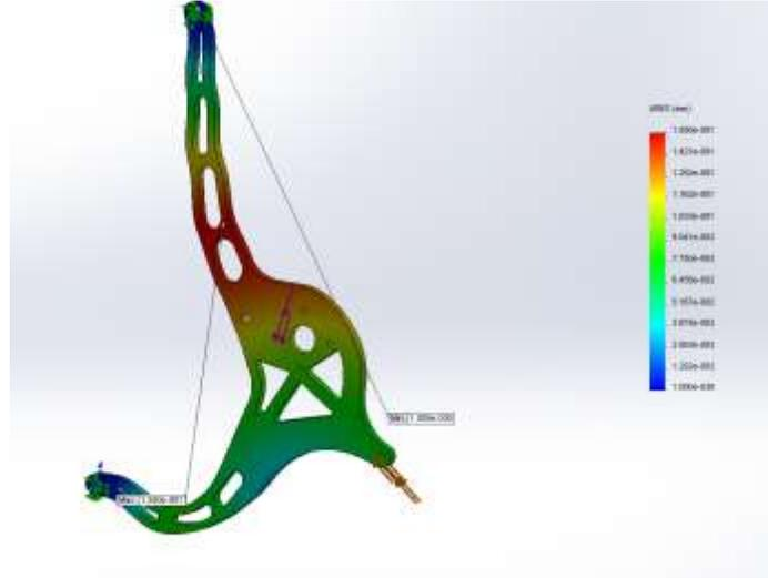
Figure 24: Deflection under Downward Load
