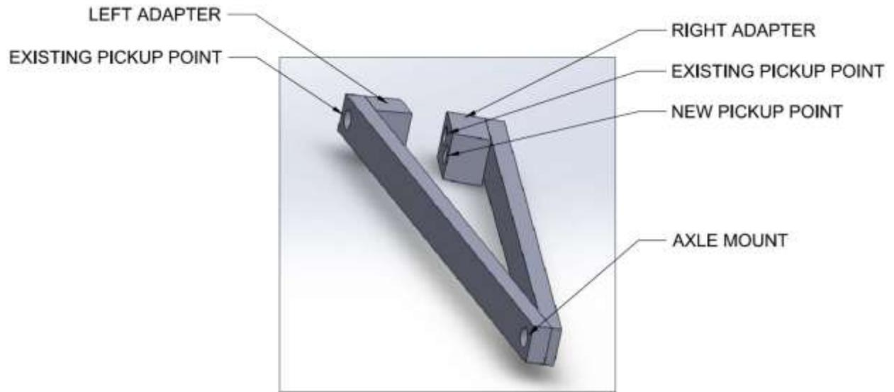
Figure 28: Semi-Trailing Arm Mounting Points (Material Between Points for Visual Purposes Only)
