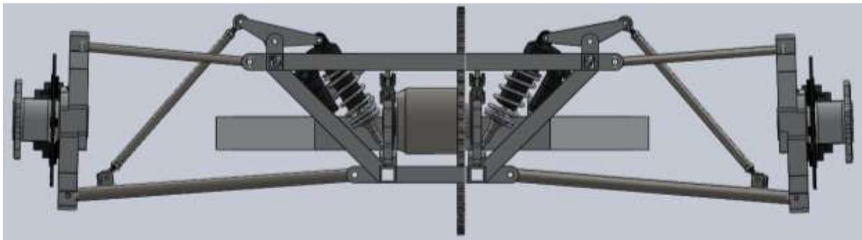
Figure 34: Pushrod Actuated Shocks Mounted Within Rear Sub-Frame
