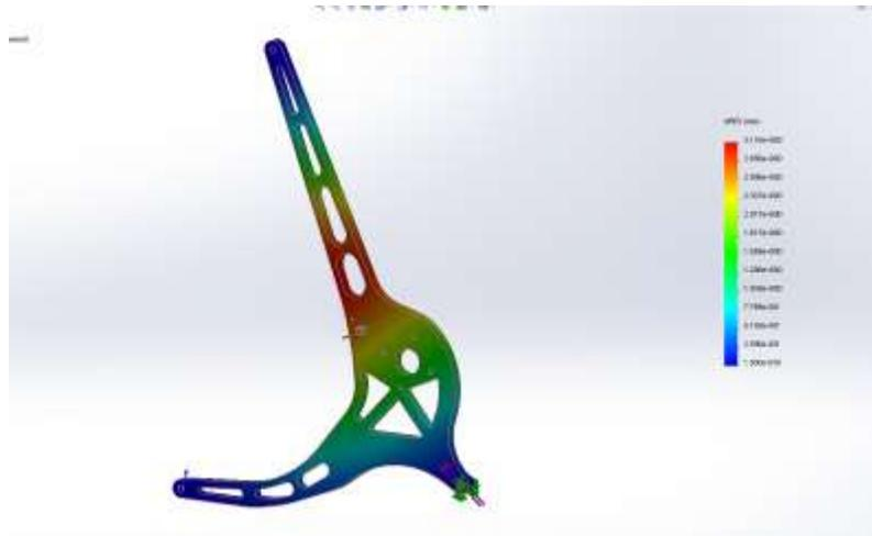
Figure 20: Deflection under Lateral Load
