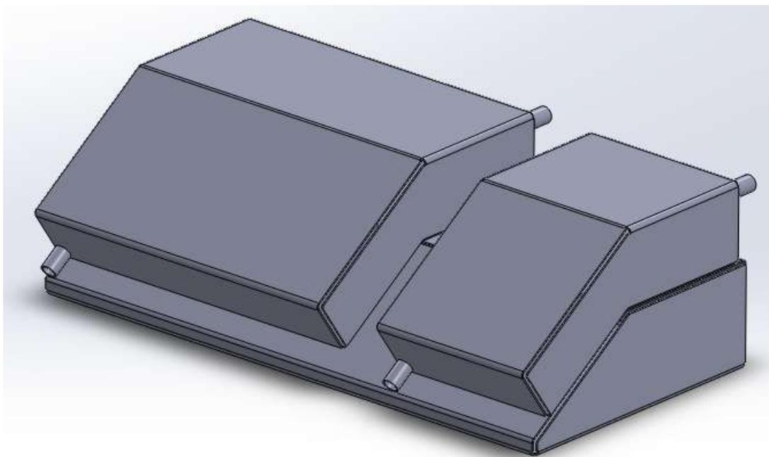
**Figure 44: Fuel, Oil, and Coolant tank assembly**
