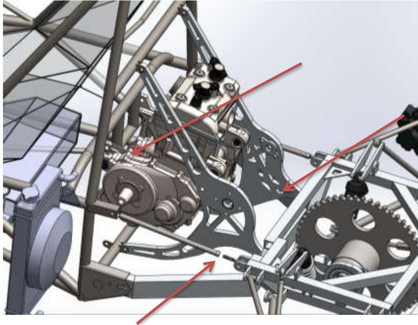
**Figure 17: Engine Mount Setup**
