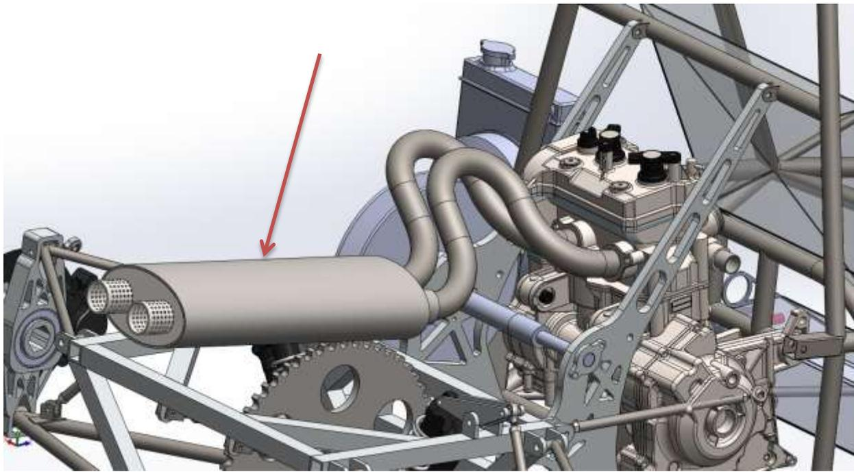
**Figure 12: Final Muffler Design**
