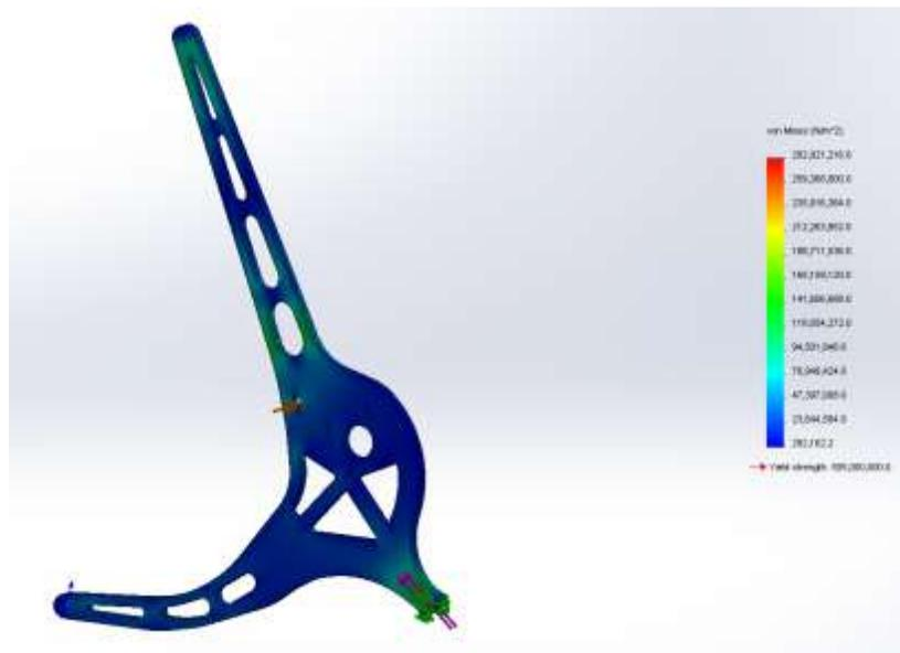
Figure 19: Stress under Lateral Load
