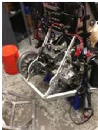
Figure 27: Water Jetted Engine Mount Components
