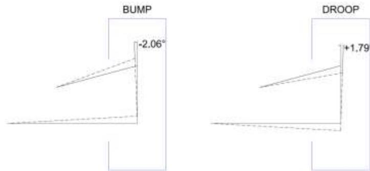
Figure 31: Camber Gain Under Bump and Droop
