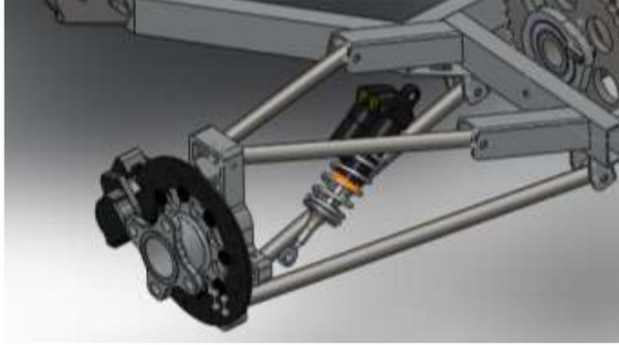
Figure 33: Final Rear Suspension Geometry
