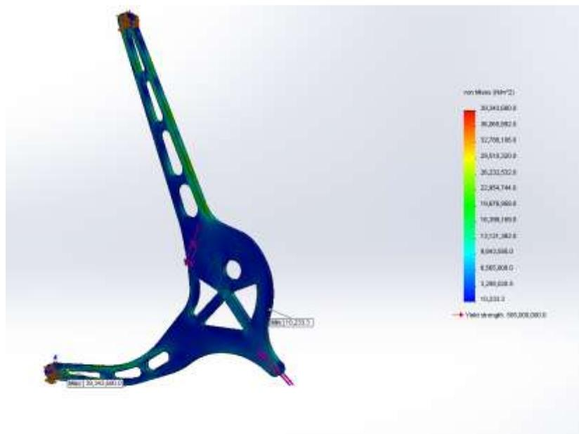
Figure 23: Stress under Downward Load
