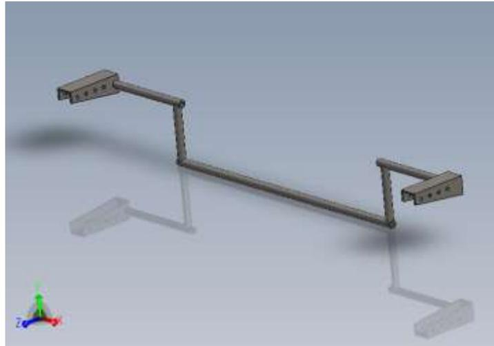
**Figure 51 Sway Bar Shape and End Hookup Design**
