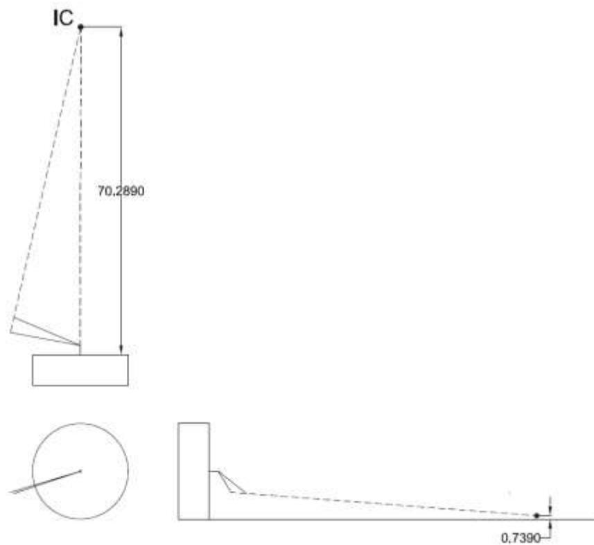
Figure 29: Determining Semi-Trailing Arm Instant Center Location
