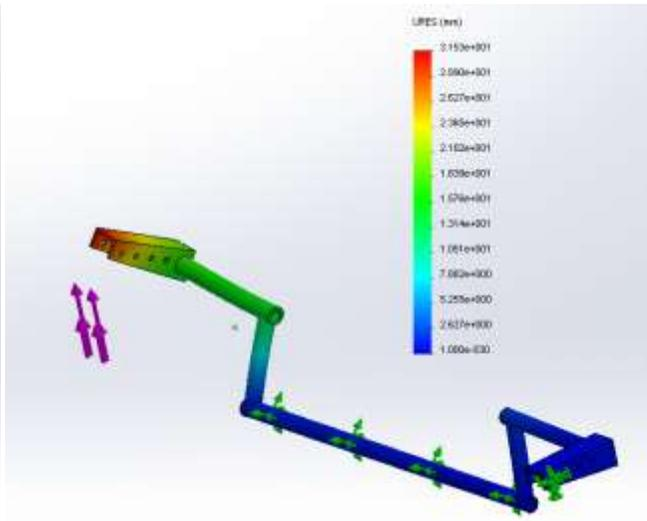
Figure 53 0.75" Sway Bar Displacement Analysis
