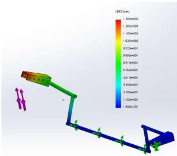
Figure 54 0.50" Sway Bar Displacement Analysis
