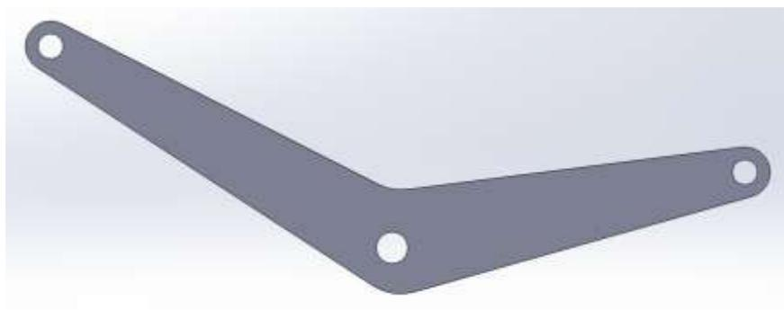
**Figure 35: Rocker Shape - (Left to Right) Pushrod Mount, Pivot, Shock Mount**
