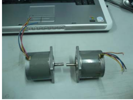
Figure 4.19 Step Motors used to drive the Knee Motion
