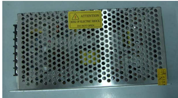
Figure 4.17 Electric Power Source for Control System
