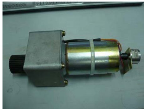
Figure 4.18 DC Motor used to drive the Hip Motion
