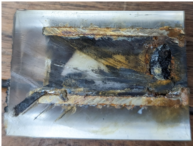
Image 13: Porous titanium cathode mesh sample from the second cathode test. The cathode was cut in half to reveal its cross section, as seen in the image.
