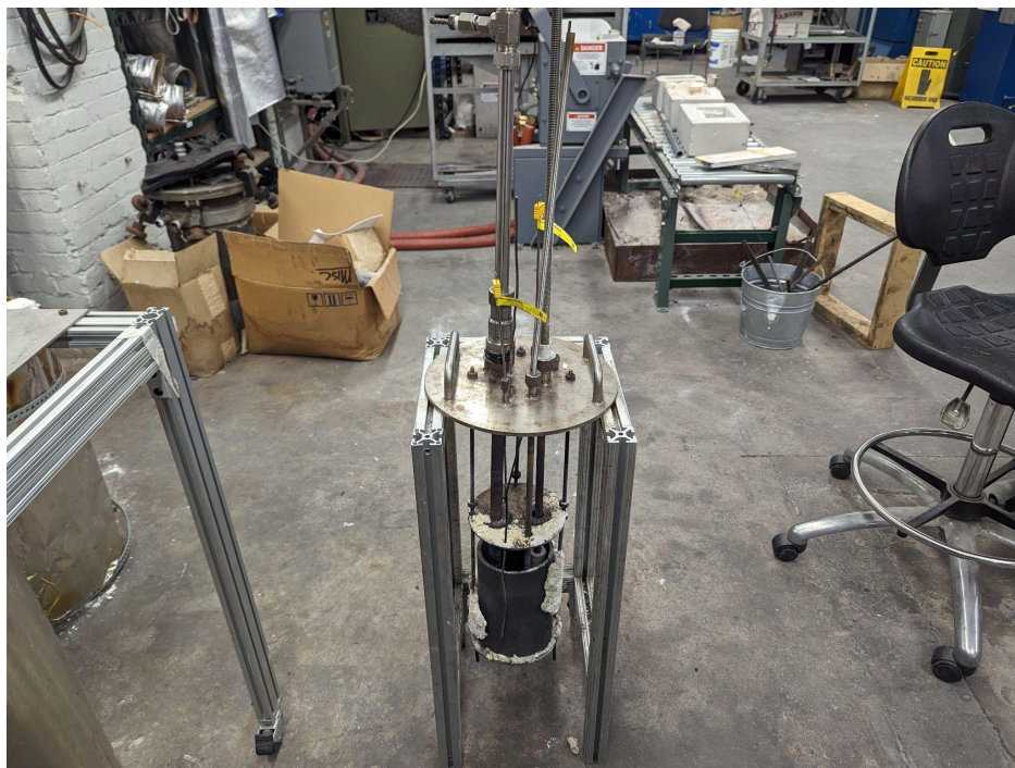
Image 1: Final setup of the Magnesium-Air Battery containment cage, including the cathode, anode, cold finger, and crucible.
