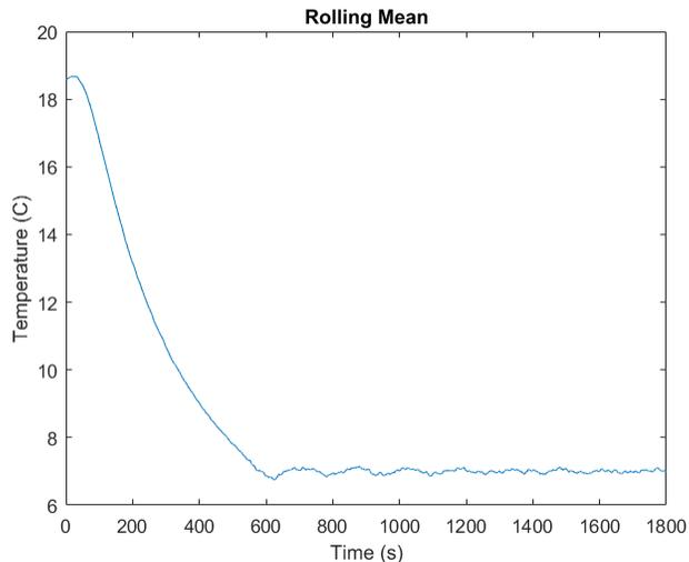
Figure 40: PID control of temperature with a target of 7 degrees Celsius
