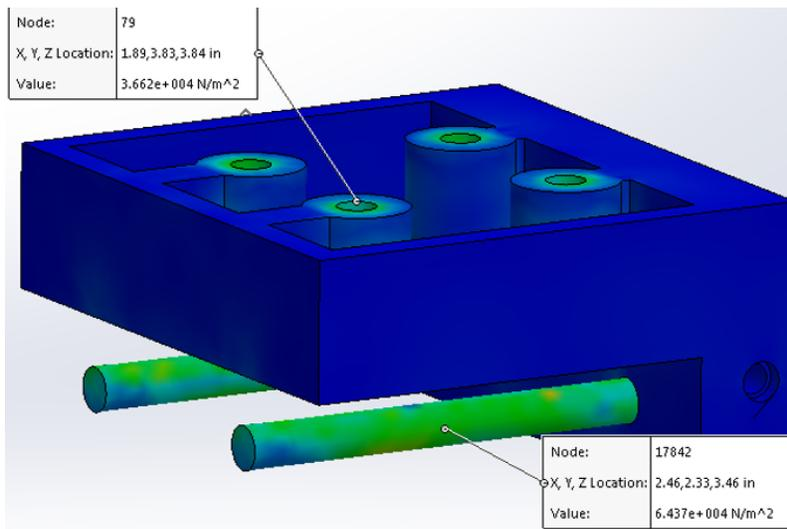
Figure 27: Solidworks Simulation of Von Mises Stress on the Drone Mount
