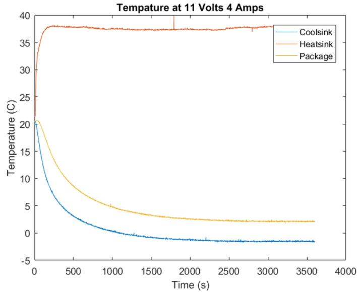
Figure 29: Measured temperature of package with 1.0in insulation thickness
