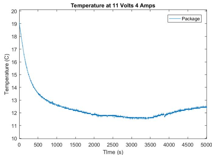
Figure 28: Measured temperature of package with 0.5in insulation thickness
