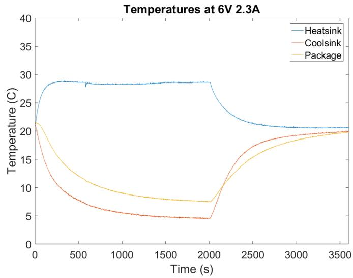
Figure 49: Test 1" insulation with shutoff (6V)
