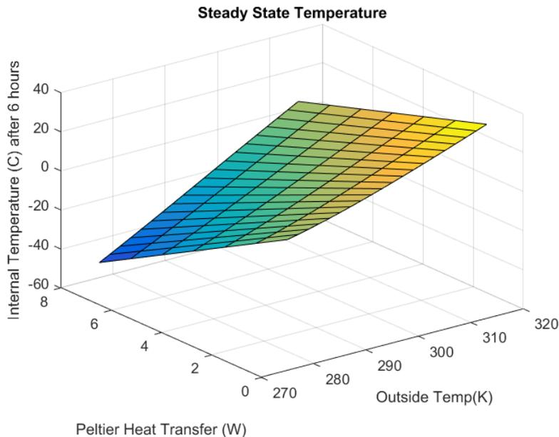
Figure 23: Steady state internal temperature at different TEC wattages and external temperatures
