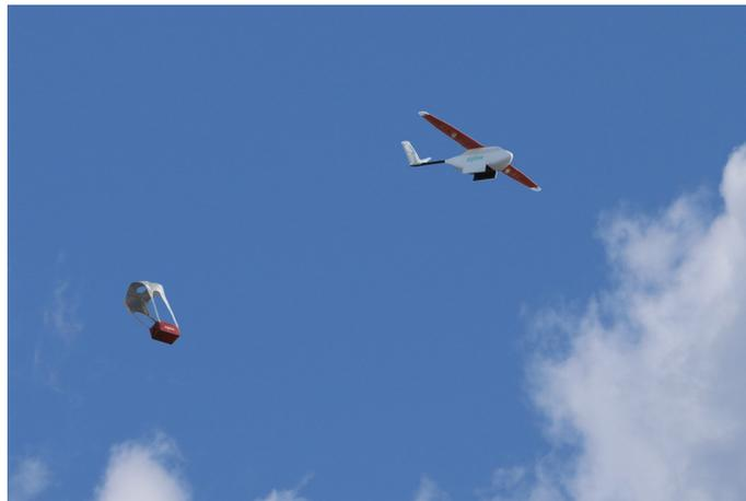
Figure 5: A Zipline "Zip" delivering supplies via paper box and parachute.
