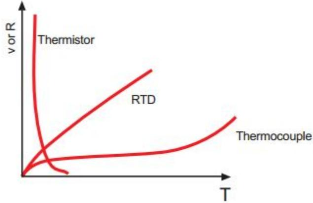
Figure 12: Generic graph of thermistor resistance changes
