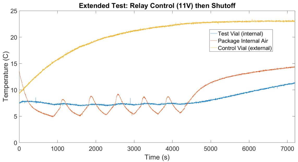
Figure 57: 3.0 Test full load relay control with extended off period
