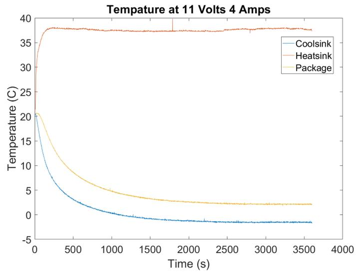
Figure 52: Test full power (11V)
