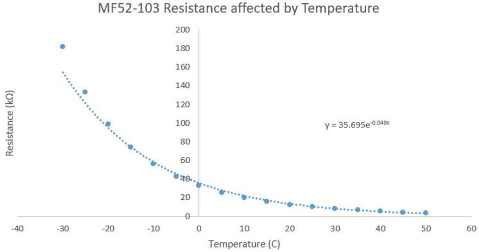
Figure 13: Determination of intermediate resistor values
