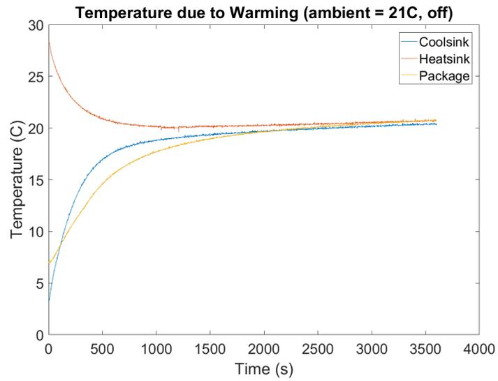
Figure 51: Test warming with no power
