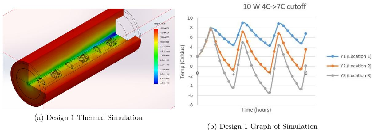
Figure 20: SolidWorks thermal model and resulting temperature plots for each vial location
