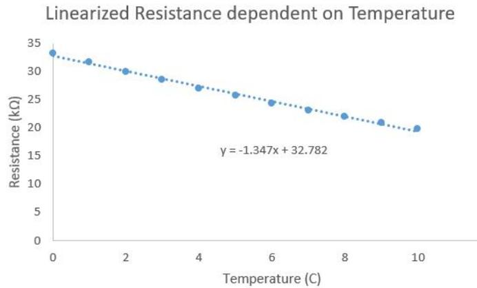
Figure 14: Determination of intermediate resistor values
