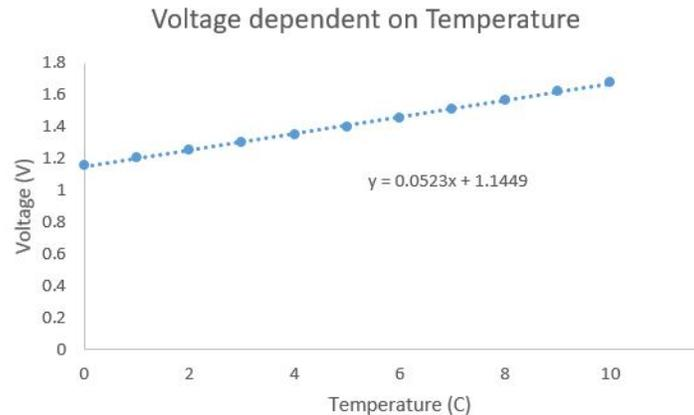
Figure 15: Voltage divider output dependent on temperature
