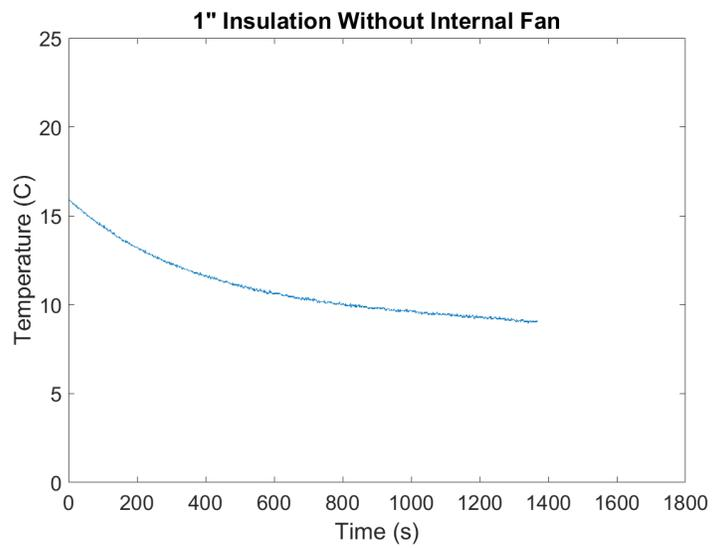
Figure 48: Initial test 1" insulation w/o fan (11V)
