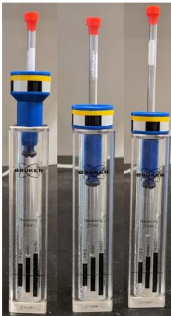
Figure 3: Visual aid for the proper use of the NMR leveling jig.
