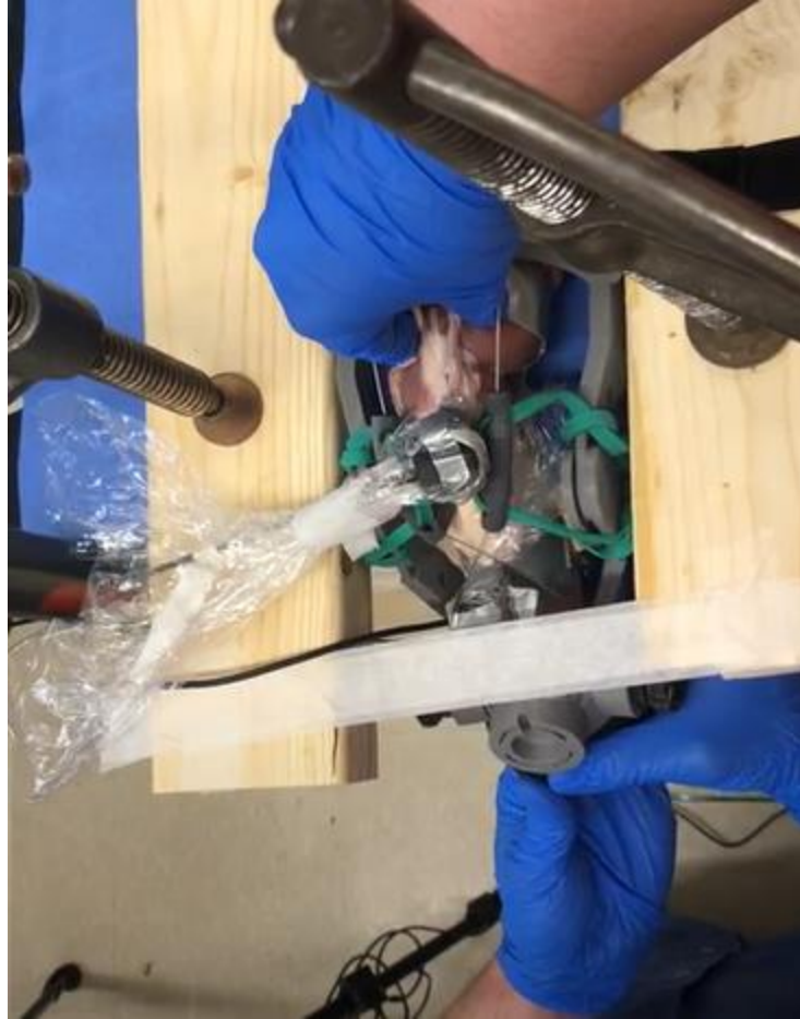
Figure 66: The brace and thigh region of the leg are fixed by clamps, and by a team member placing a force on the quadriceps region to hold the leg down
