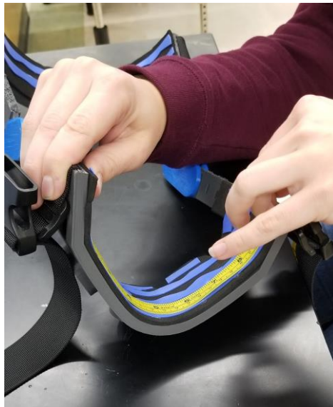
Figure 26: Measurement of the brace dimensions
