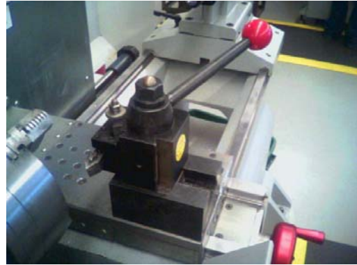
Figure 2.6 Lathe cutting tool and chuck
