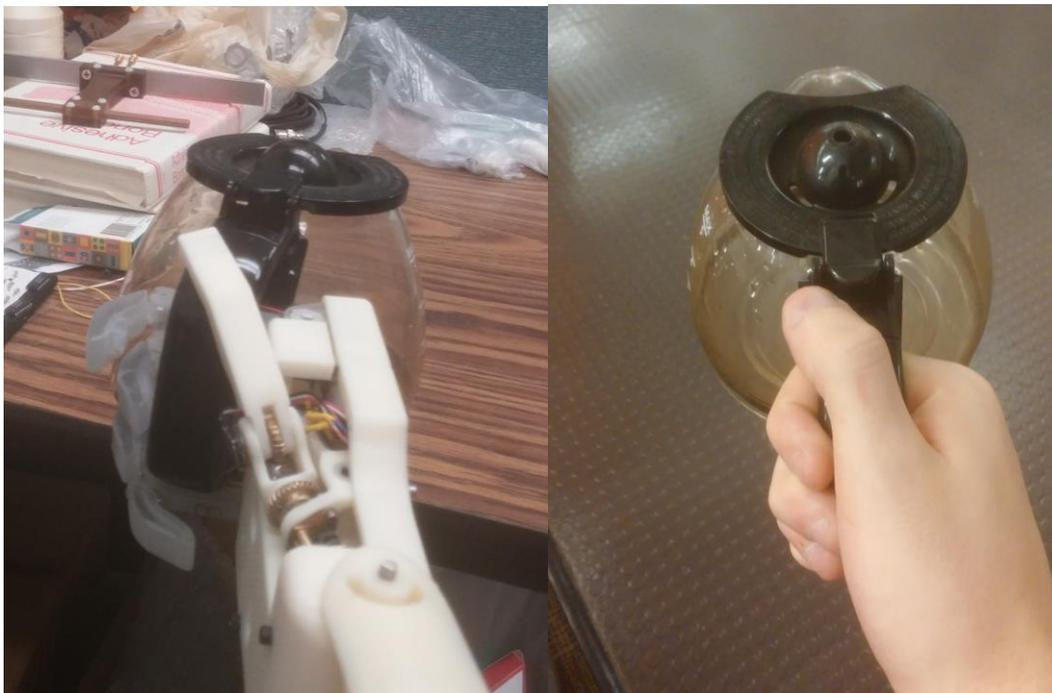
Figure 28: Robot vs Human Grip on the Coffee Pot
