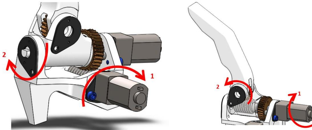
Figure 19: Rotational patterns of the Thumb
