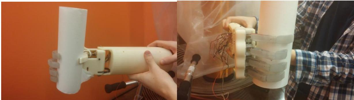
Figure 26: Holding the Heavier and Harder to Grip Paper Towel Roll
