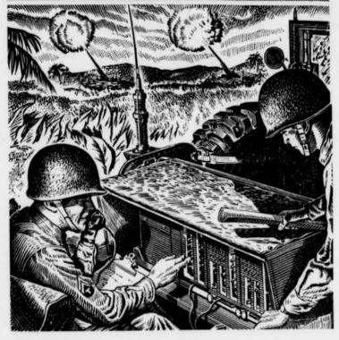
ONG TOMS - blasting unseen targets - are I directed by voices flashing through this artilleryman's radio telephone "switchboard." His FM set can operate on 120 crystal controlled channels, any ten selected instantly by push-buttons. Using its many channels, he connects the battalion commander with spotters up front and in planes; then with battery commanders who focus tremendous firepower. He's helping soften the hard road ahead.
