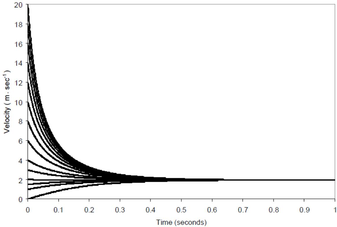
Figure 5: Initial Velocities vs. Terminal Velocity [1]
