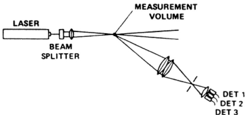
Figure 12: Phase Doppler Anemometer Diagram [14]
