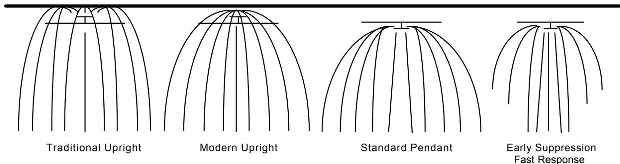
Figure 3: Sprinkler Spray Shapes [1]
