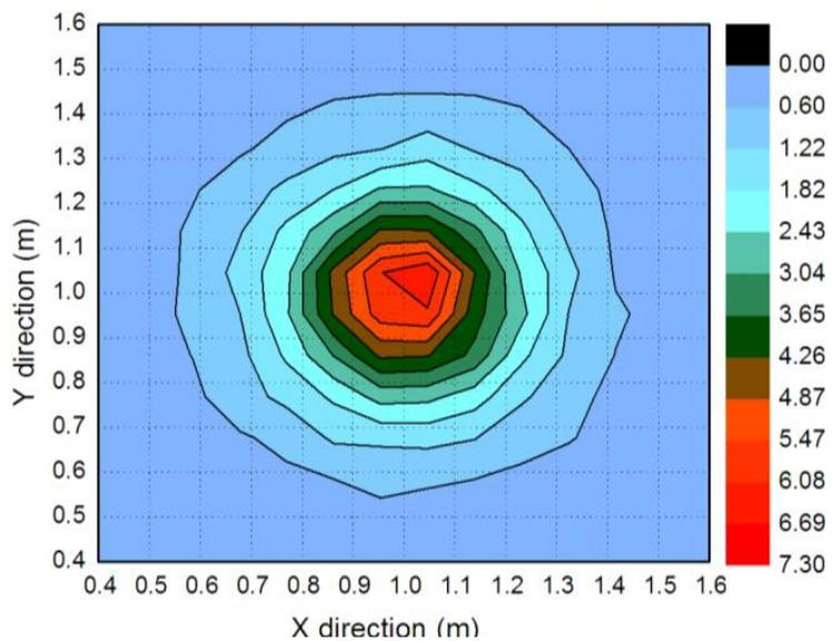
Figure 2: Contour map of FDS water flux density distribution in  $L/m^2$  [3]
