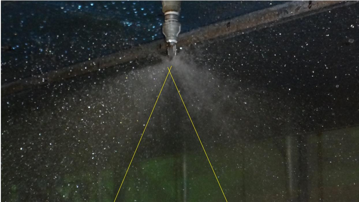
Figure 4: Inner Spray Angle
