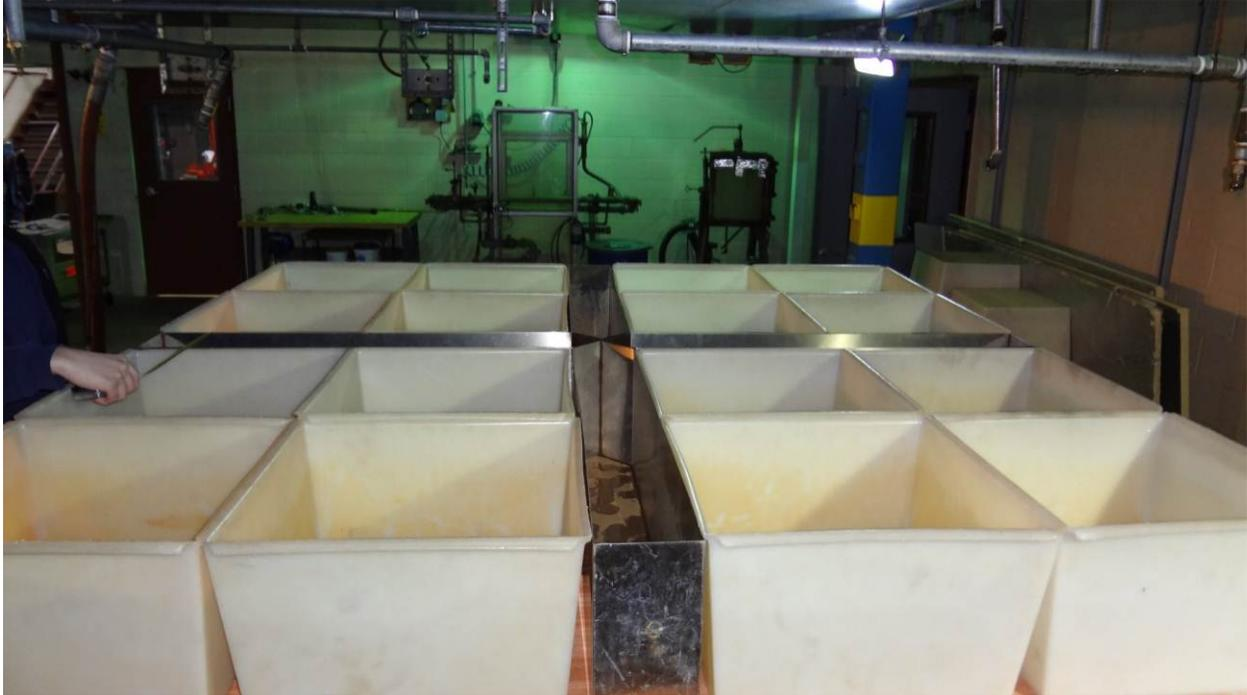
**Figure 20: Tyco Bucket Test Setup**
