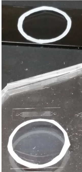
Figure 26: Fibrin Gels crosslinking in vellum rings on PDMS (microvascular layer) and Dacron (flat gel)
