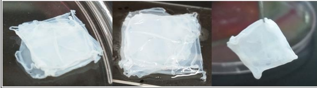
Figure 31: Preliminary Gel Stacking; Image on right shows gel out of solution holding a square shape
