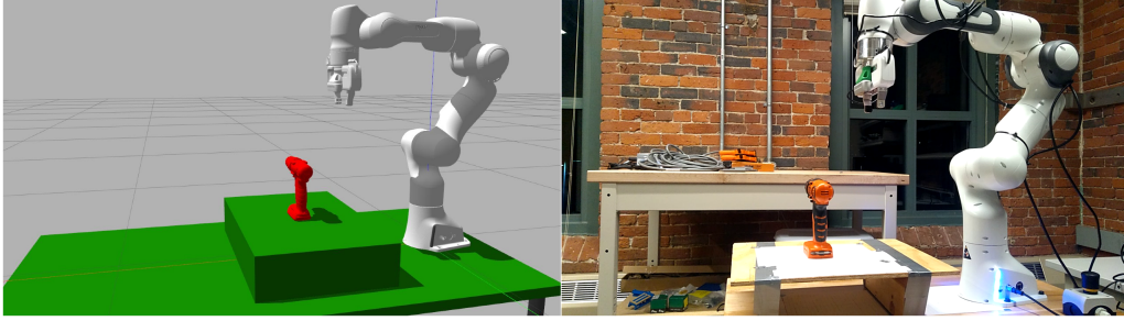
Figure 7.1: The setup as seen in simulation environment (left) and lab environment (right) with power drill in place
