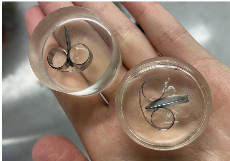
Figure 20: A photograph of pieces of the silicon wafer mounted using Epoxicure 2 and a metal stand to hold the wafer upright.
