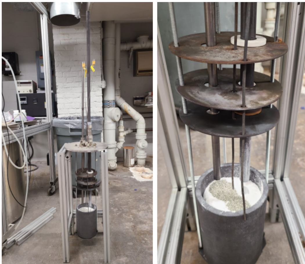
Figure 18. Photograph of electrolysis cage set up (Espinosa, Rutherford, Wallace, Powell, 2020).
