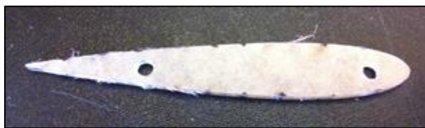
Figure 31. Acrylic NACA 0015 cross section
