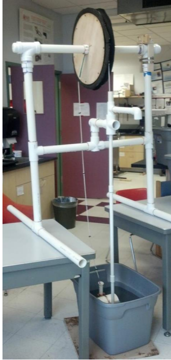
Figure 33: Final Constructed Rope Pump
