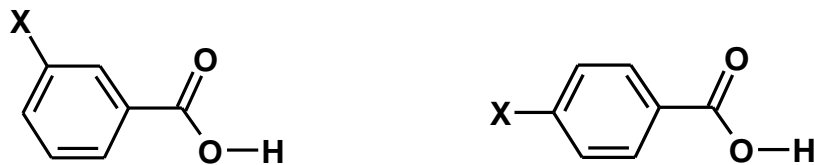
Figure 11. Benzoic acids substituted at the 3- and 4- positions with X groups. X = Cl, CH 3 , Br, or I.
