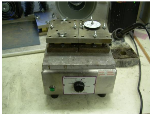
Figure 34: Fixture and hot plate for placing boards on heat sinks
