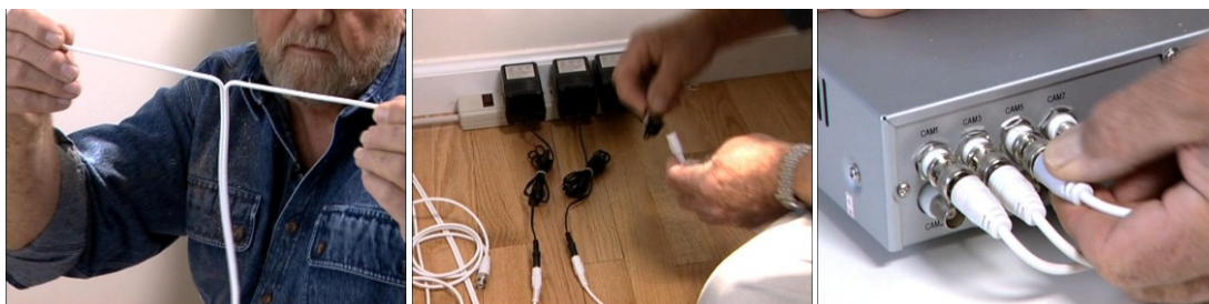
The power and video cords are pulled apart and attached to the power outlet and digital video recorder. The DVR is then connected to a TV or Computer monitor (Not Shown).
