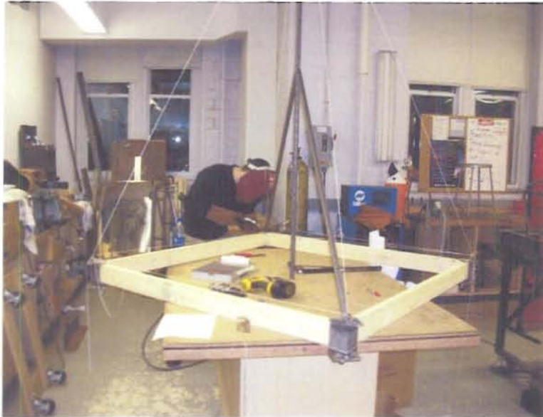
Figure 25: Wooden Jig Constructed, Corner Bracket Being Welded
