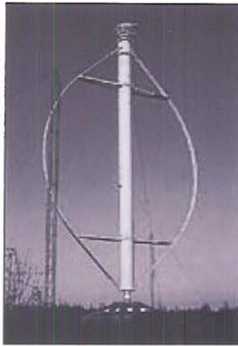
Figure 10: Vertical Axis Wind Turbine [12]
