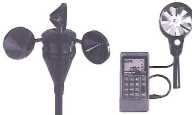
Figure 8: Mounted and Handheld Anemometers [10]
