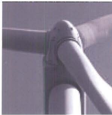
Figure 13: Hub and Blades of a Turbine Rotor [15]
