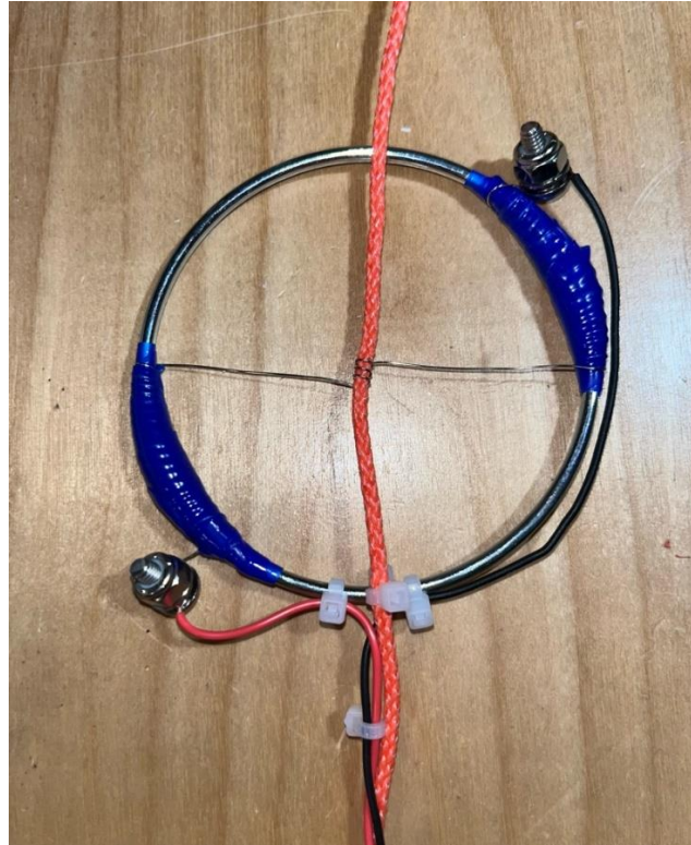
Figure 20: Final ETS Heating Element Configuration
