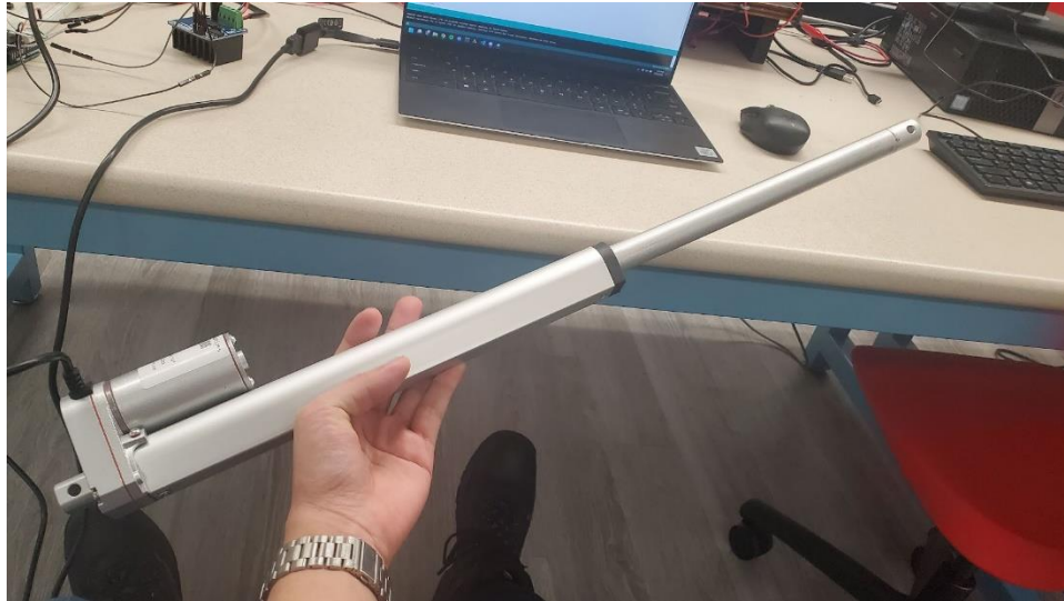
Figure 45: Linear Actuator Fully Extended using a Variable Supply
