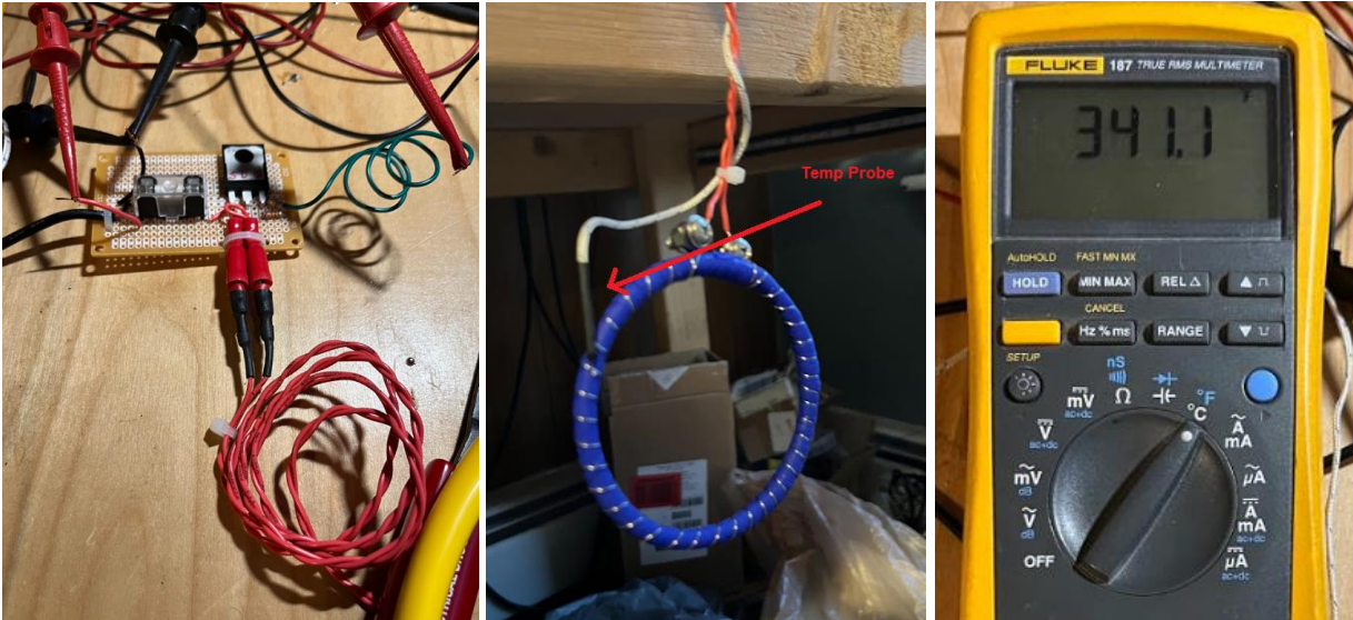
Figure 17: ETS Heating Element Temperature Test
