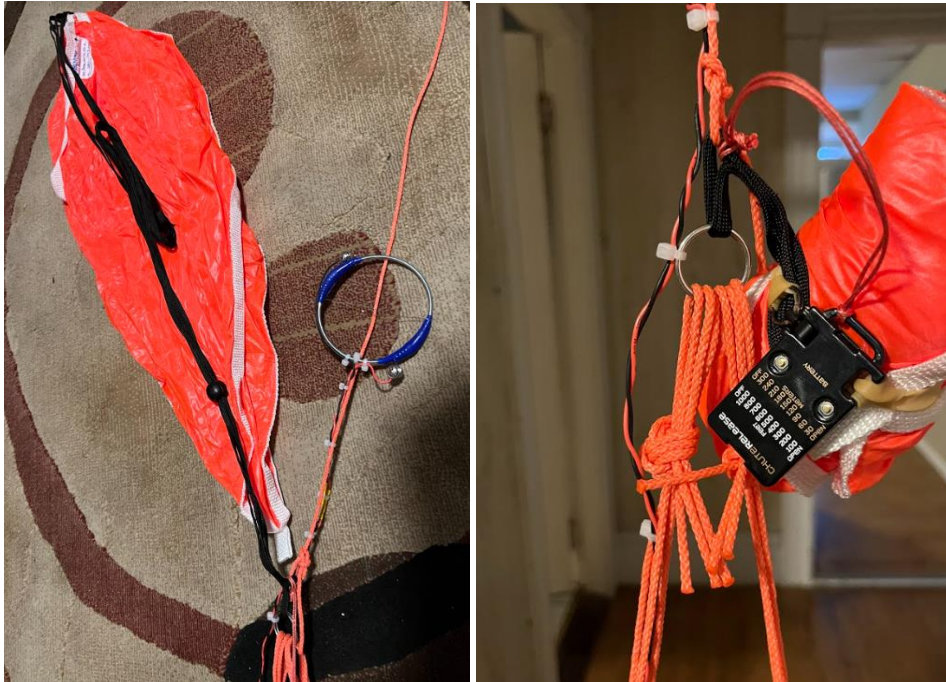
Figure 21: Payload Parachute Line Configuration
