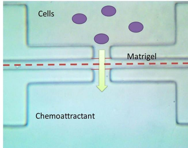
**Figure 5: Final Design Function Schematic**
