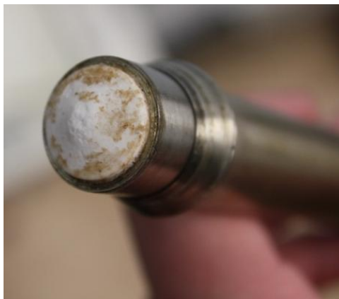
Figure 5-4: Solidified salt at bottom of reactor
