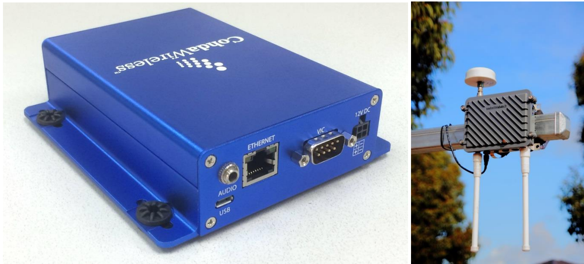
Figure 35 - Cohda Wireless Products, OBU left, RDU right
