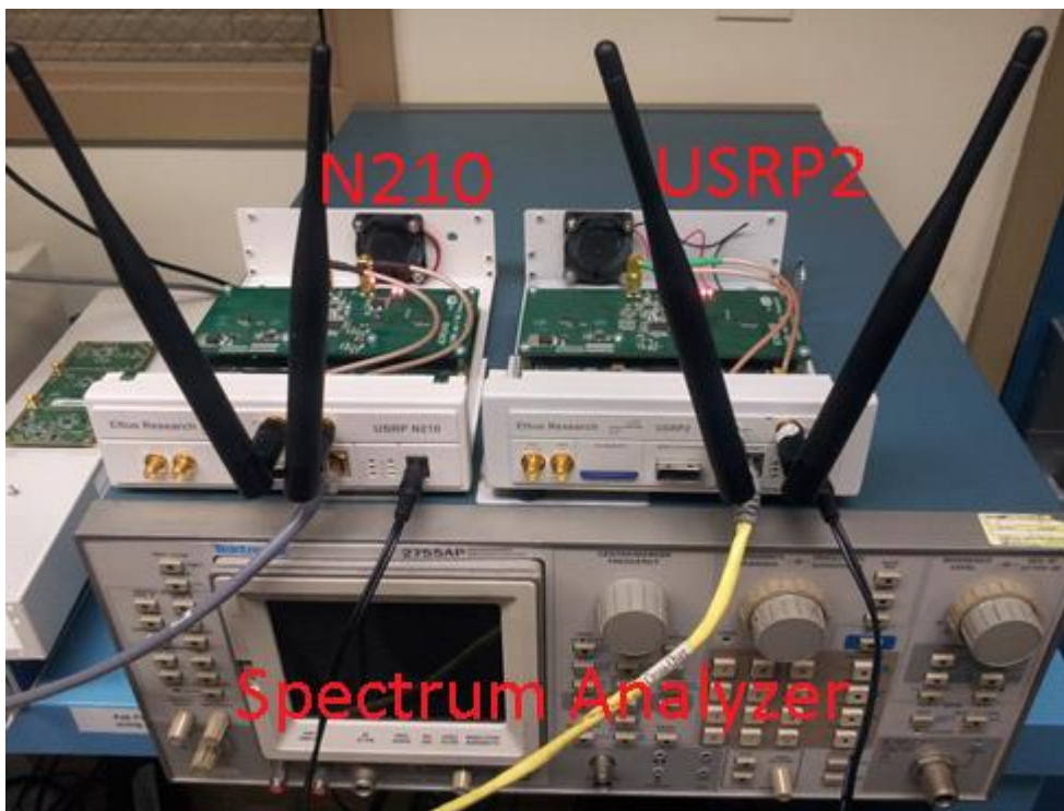
Figure 1 - Experiment Setup with N210 (left) and USRP2 (right). The only relevant difference between N210 and USRP2 is that FPGA image and ZPU firmware is loaded from SD card in case of USRP2 or from flash IC in case of N210. The box at the bottom is a spectrum analyzer used to confirm the presence of 802.11p carrier frequency.
