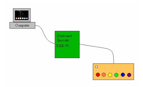
This prototype is a combination of a flash animation along with a button box that connects to the computer. The button box is connected to the keyboard port of the computer using a keyboard encoder. For purposes of our model we used a keyboard encoder loamed to us by Ken Chan. A similar board can be used or can be purchased through Auden Electronics, we suggest model KEP-629. The buttons are then hooked up to the board so that the characters shown on the following page are produced.
