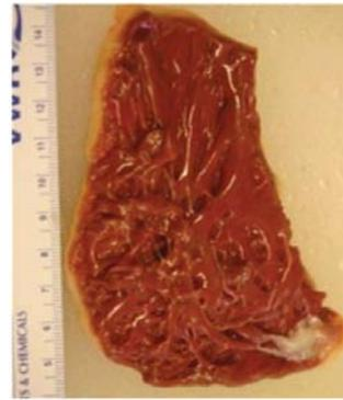
(c) Tissue sample mounted for biaxial test
