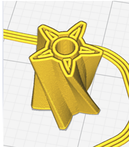
Figure 9-13: Sliced Layer view of Worm Gear
