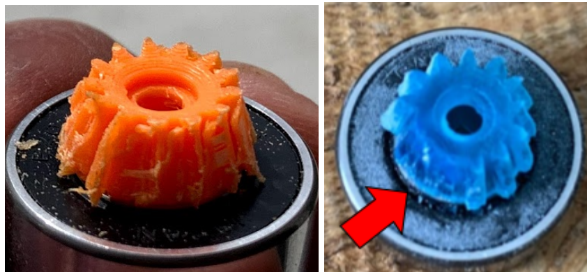
Figures 9-21: Example of Pinion Failure (Left Image: PLA, Right Image: Tough Resin)
