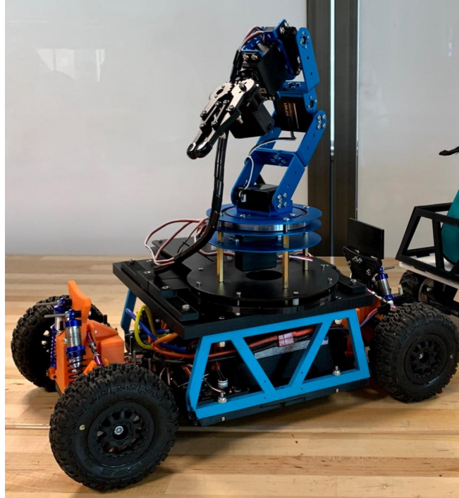
Figure 13-3: Robotic Arm Attached to PARV Using the Mounting Plate
