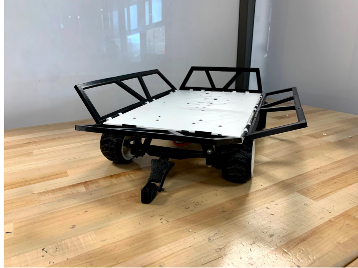
Figure 13-4: Trailer with its Sides Dropped Down
