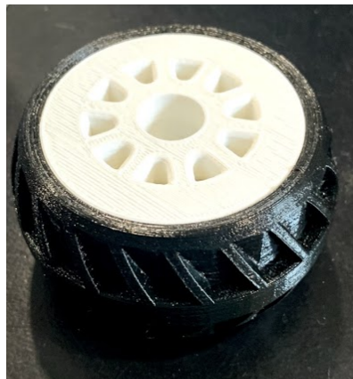
Figure 11-3: First Iteration of Printed Wheel
