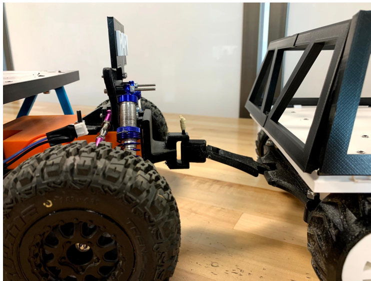
Figure 11-9: Trailer Hitch Assembly Attached to PARV
