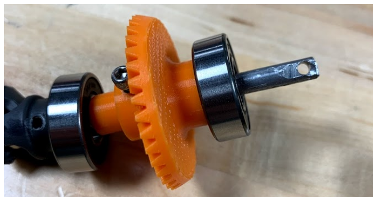
Figure 9-20: 3D Printed Ring Gear With Metal Shaft
