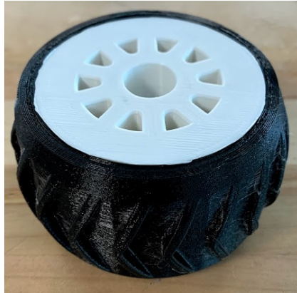
Figure 11-4: Final Iteration of Printed Wheel
