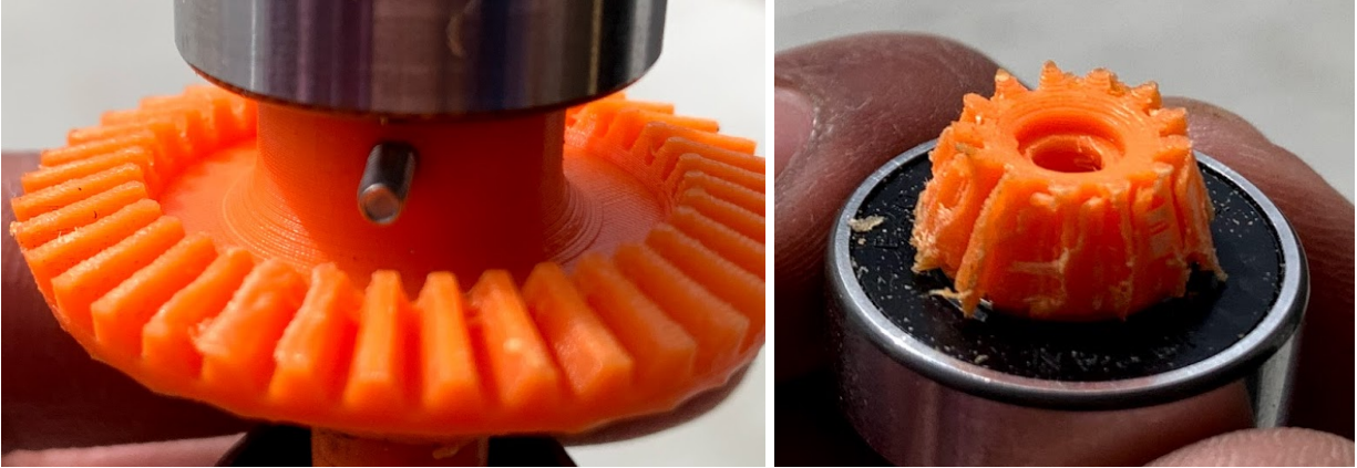
Figure 15-3: Damage On Direct Drive Ring and Pinion Gears
