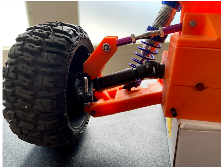
Figure 12-4: Picture of Front Left Suspension With Hobby Store Drive Shaft, Turnbuckles, and Shocks
