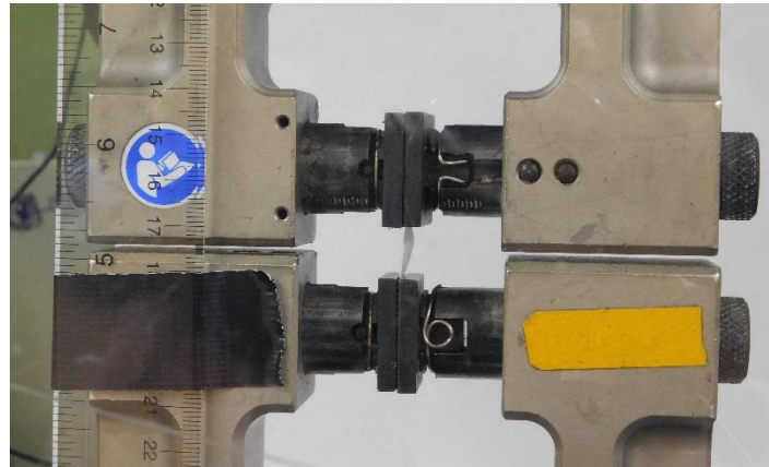
Figure 18: Tensile Strength Test Setup
