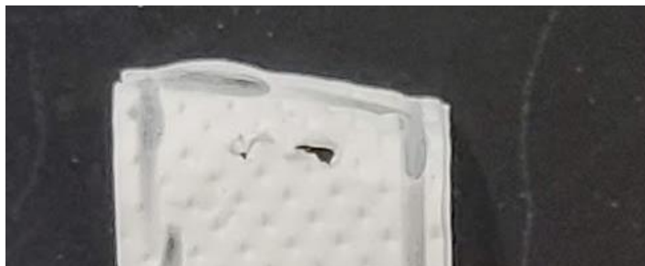
Figure 30: Suture Pullout Test Example
