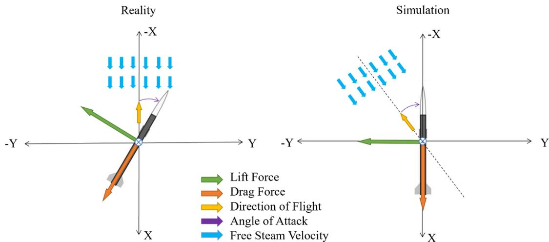
Figure 4-21 Orientation of Rocket and Free Stream Velocity
