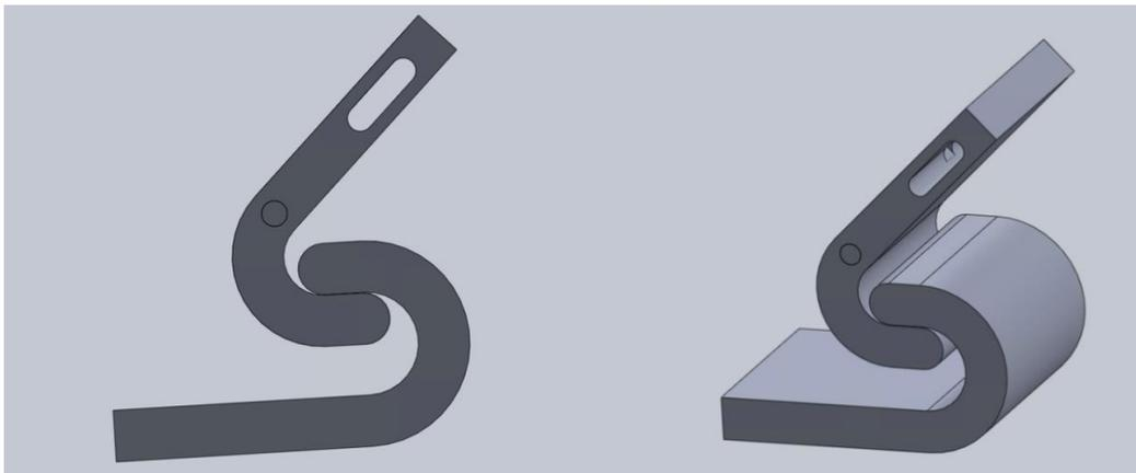
Figure 3-4 Left View and Trimetric View of Circular Clasp SOLIDWORKS Model
