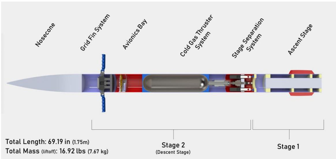
Figure 2-4 Cross Section, Project Andromeda Rocket
