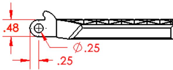
Figure 2-11 Grid Fin Dimensions in Inches, Side View
