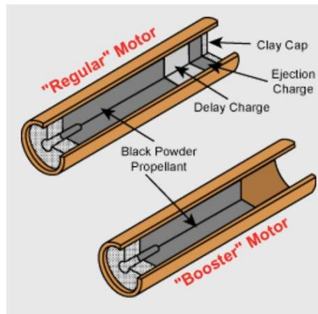
Figure 1-20 Black-powder Stage Separation Rocket Engine © Apogee Rockets 2019
