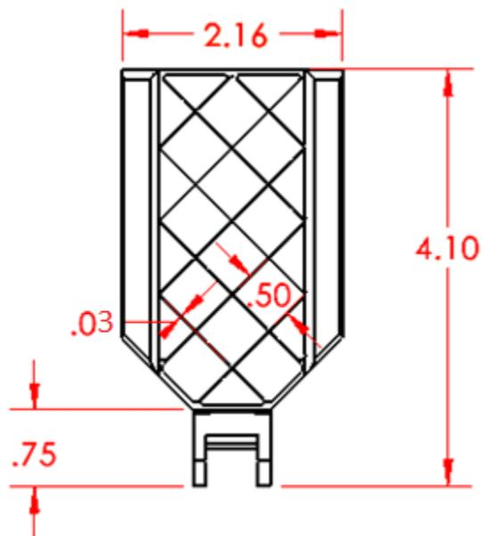
Figure 2-10 Grid Fin Dimensions in Inches, Bottom View
