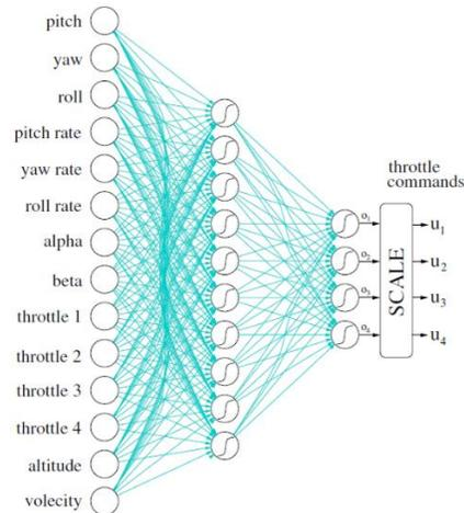
Figure 1-34 A Visualization of a Neural Network for Guidance of a Finless Rocket [48] © University of Texas, Austin 2003
