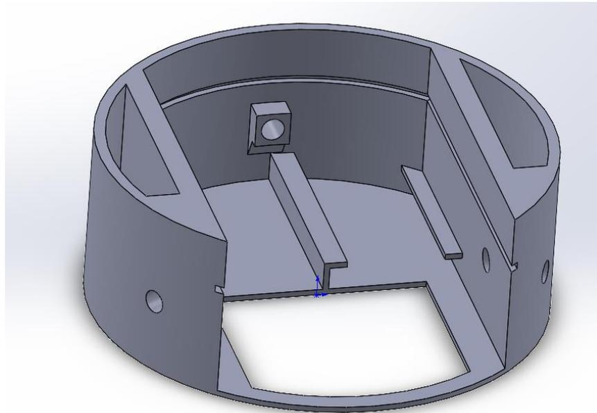
Figure 4-5 The Avionics Bay Structure.
