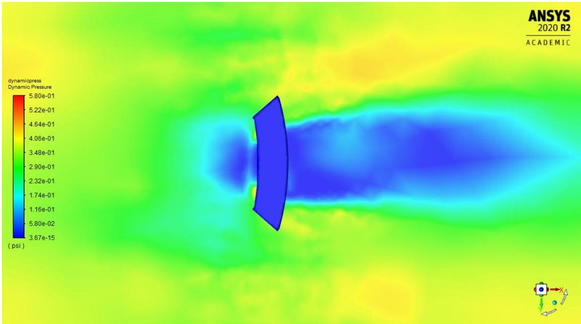
Figure 2-48 Dynamic Pressure Contour, Grid Fin  $\alpha = 0$  degrees at hinge ( $Z=0$ ) plane
