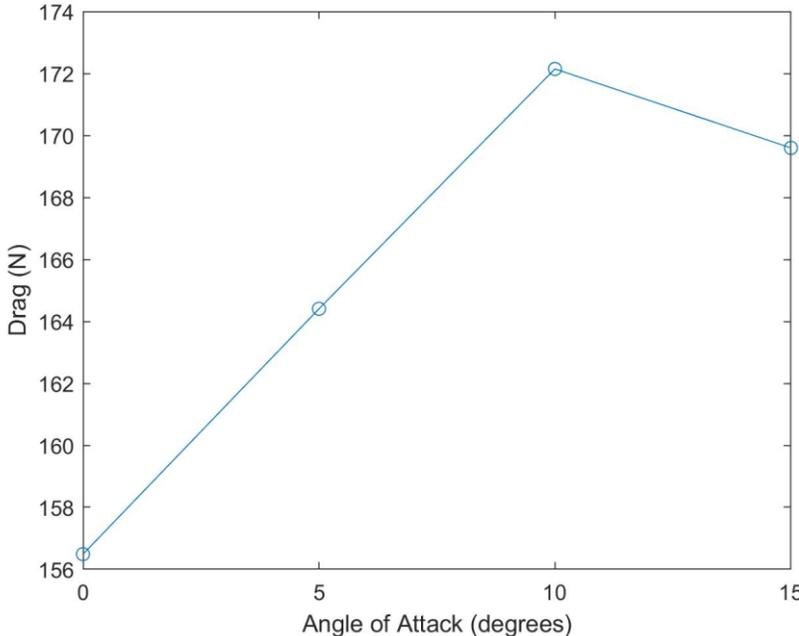
Figure 7-7 Plot of Drag as a Function of Angle of Attack
