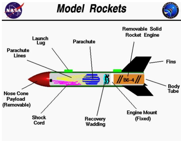
Figure 1-7 Model Rocket Cross Section © NASA 2014
