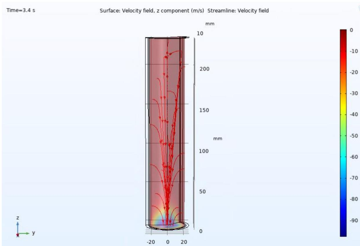
Figure 3-13 Velocity Streamlines for the Velocity Distribution in the Motor Case at  $t = 3.4$  s
