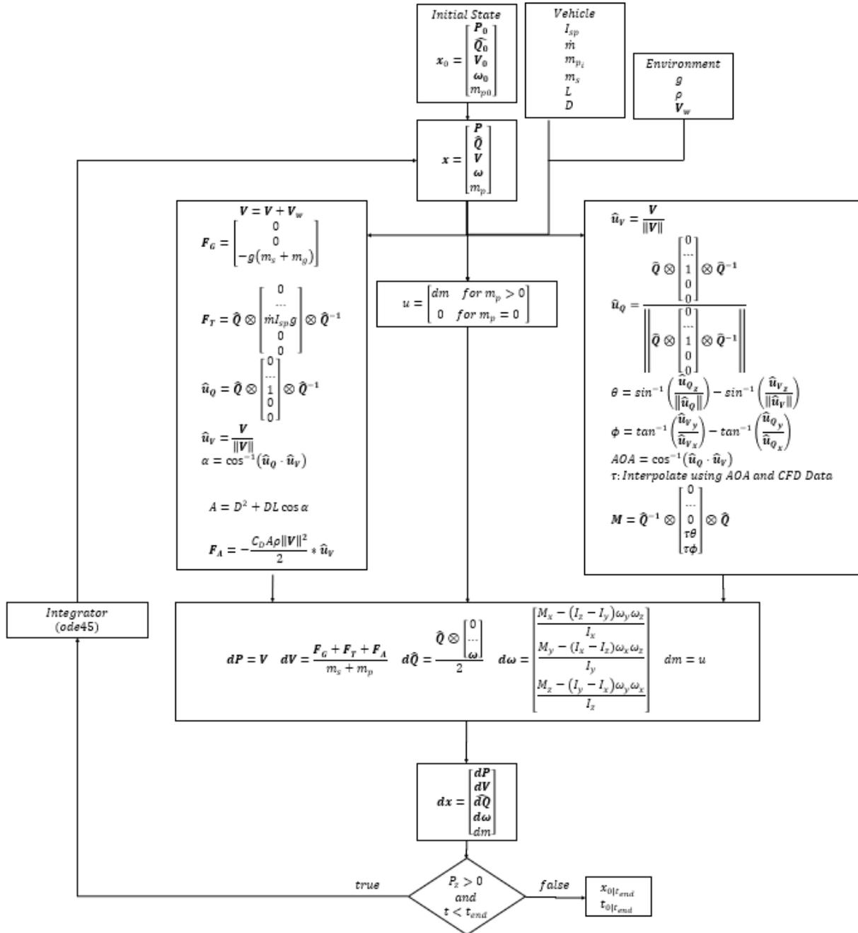
Figure 4-7 Integrated Simulation Flow Chart
