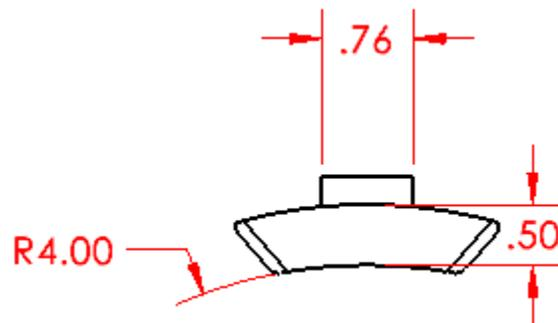
Figure 2-12 Grid Fin Dimensions in Inches, Front View
