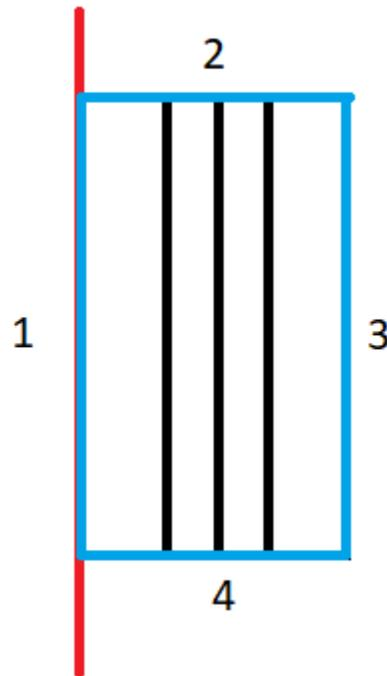
Figure 3-2 Boundary Conditions Defined in Heat Transfer Model. Domains are axisymmetric about the red centerline
