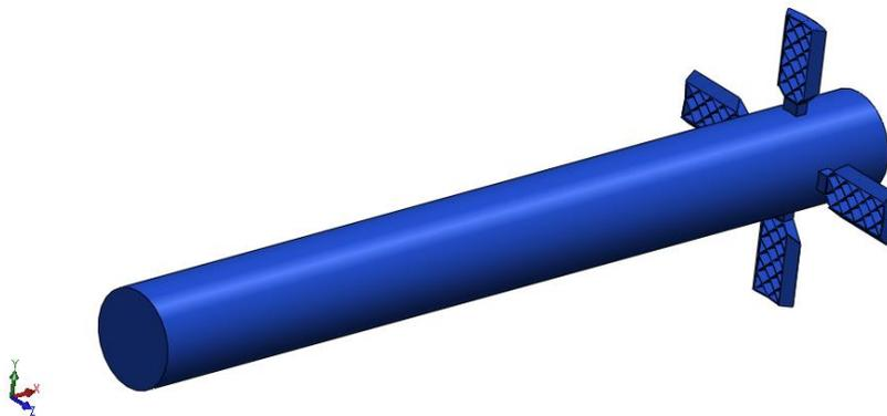
Figure 2-42 Simplified Descent Body Geometry
