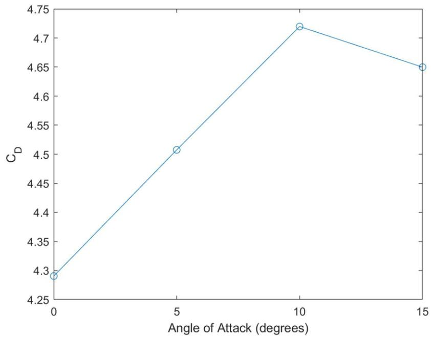
Figure 7-12 Plot of Drag Coefficient as a Function of Angle of Attack
