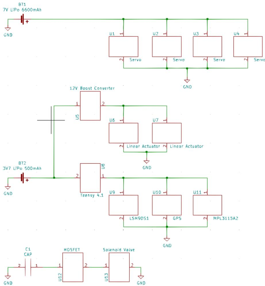
Figure 4-2 Avionics Bay Electrical Diagram
