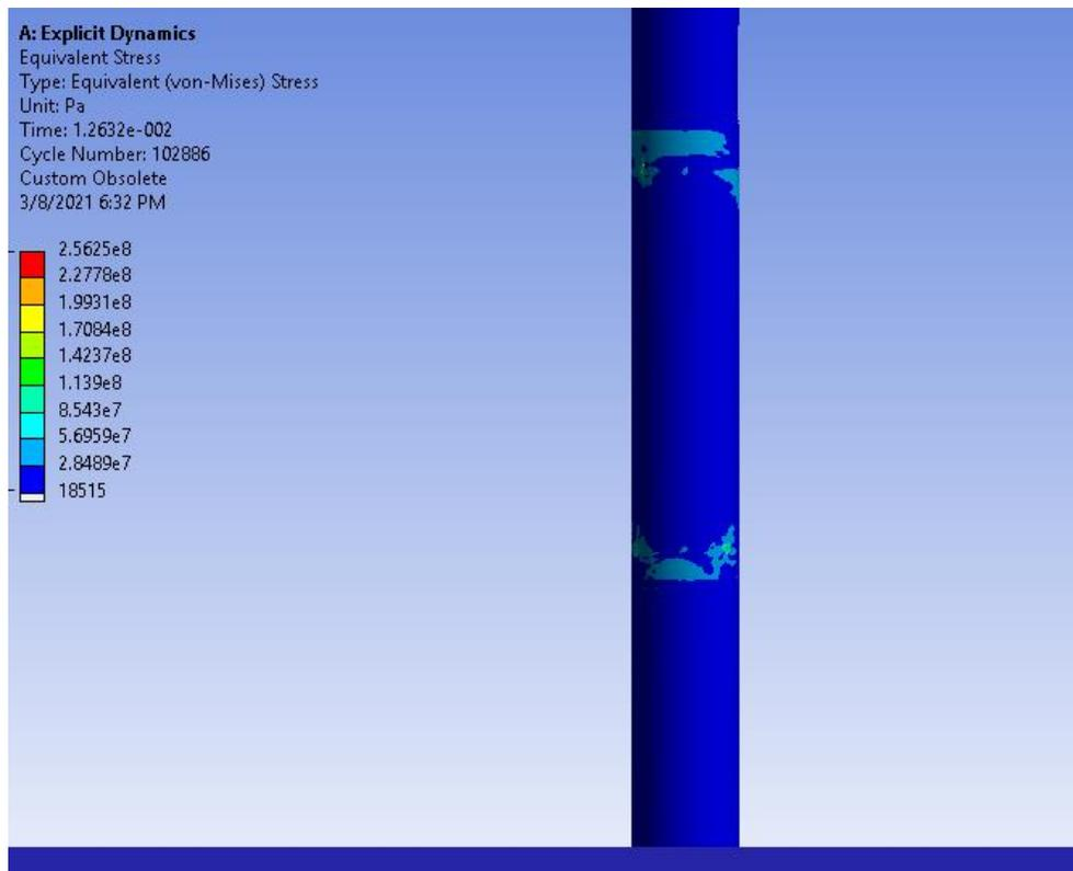
Figure 2-26 von-Mises Stress, 5m/s Impact Landing
