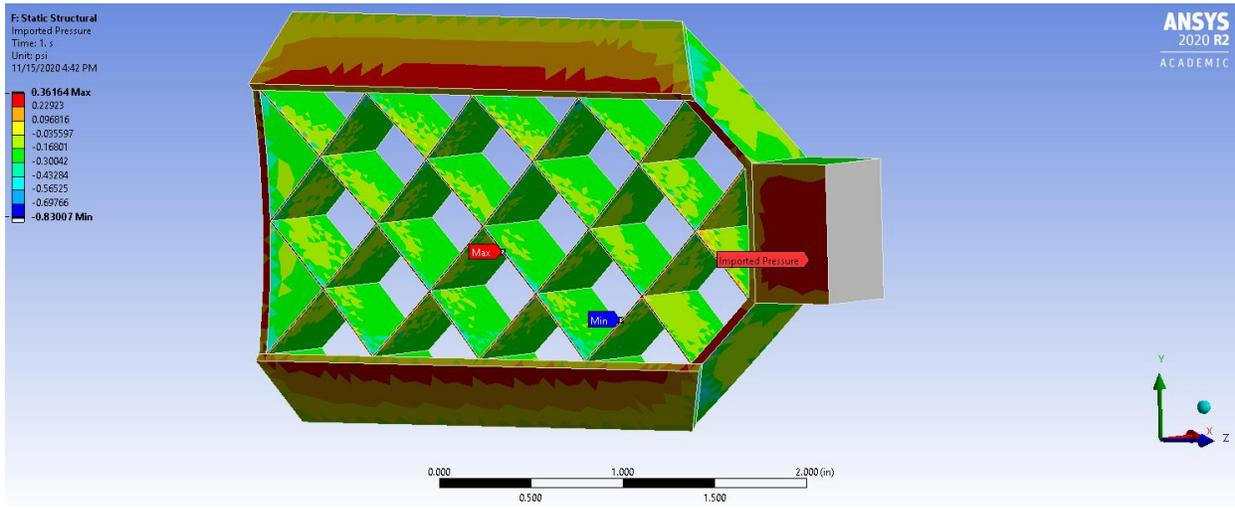
Figure 2-54 Fluent Grid Fin Imported Pressure Load
