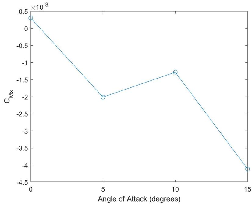
Figure 7-13 Plot of X Moment Coefficient as a Function of Angle of Attack
