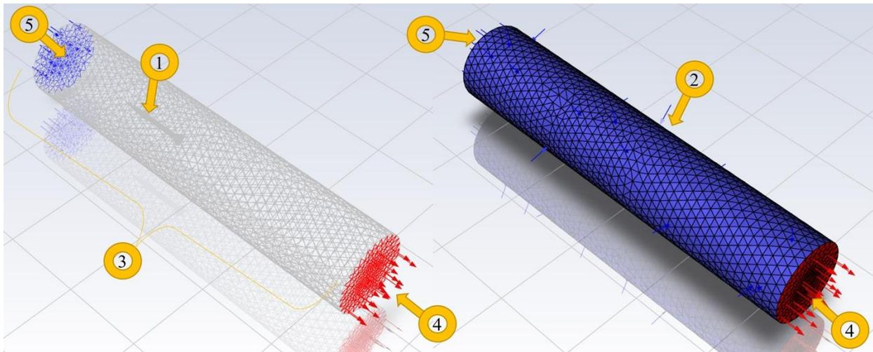
Figure 4-22 Rocket Ascent Set Up
