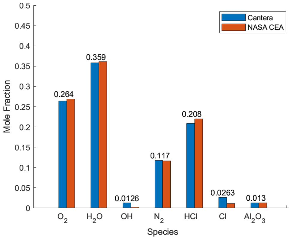
Figure 3-10 Mole Fractions of Combustion Products from each Model
