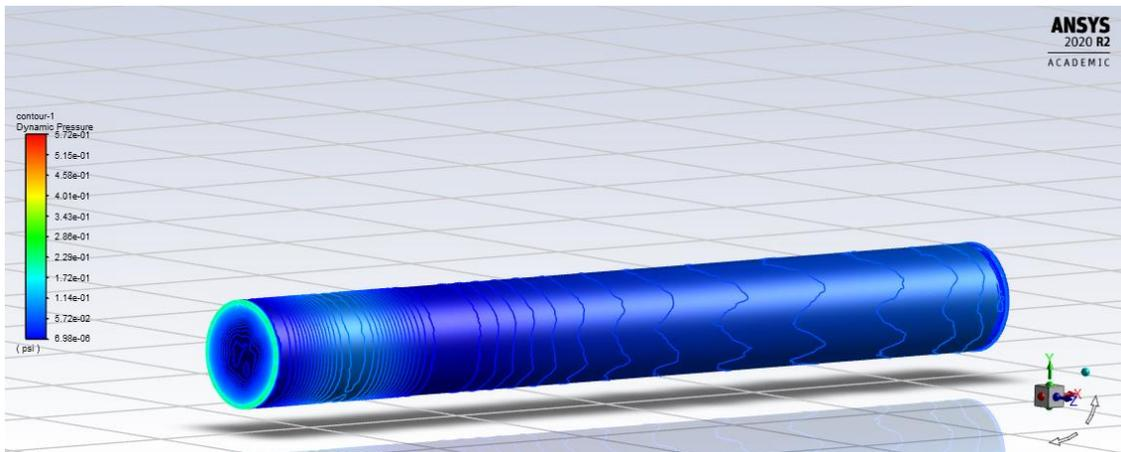
Figure 2-44 Descent Stage Simple Geometry Dynamic Pressure Contours
