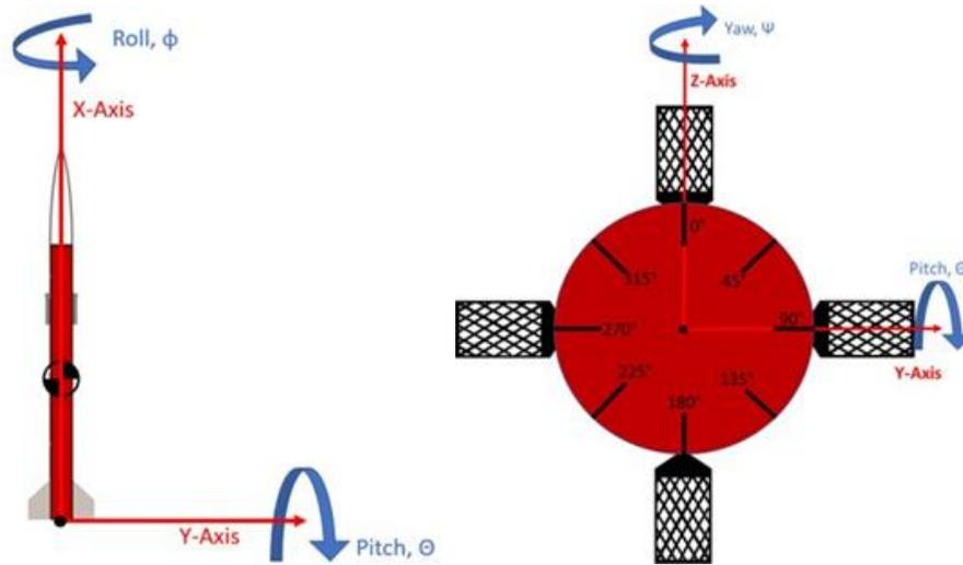
Figure 1-4 Rocket Coordinate System – Side View and Top View
