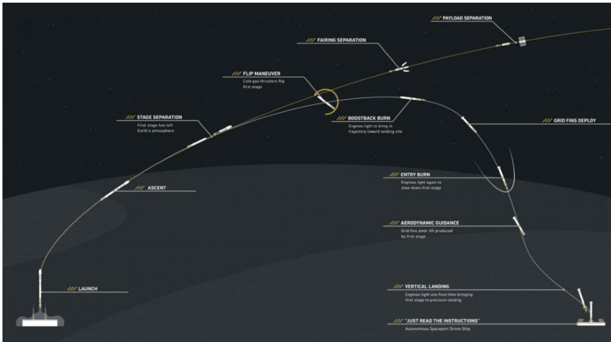
Figure 1-12 SpaceX Falcon 9 Sample Mission Profile, Falcon User Guide [7] © SpaceX 2020
