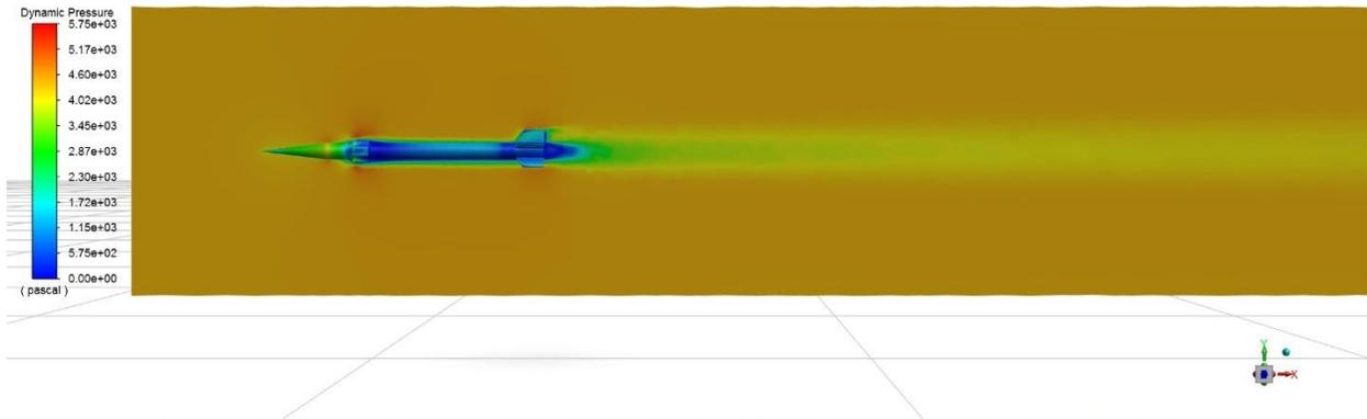
Figure 7-16 Dynamic Pressure Contour at AOA 0 deg
