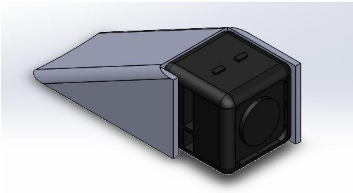
Figure 2-17 Camera and Fairing Assembly
