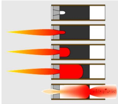
Figure 1-21 Burning Particles Produced from Black-powder Stage Separation © Apogee Rockets
