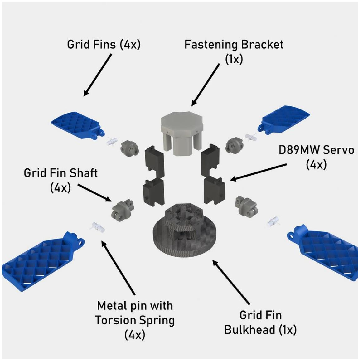
Figure 2-14 Exploded View, Grid Fin System
