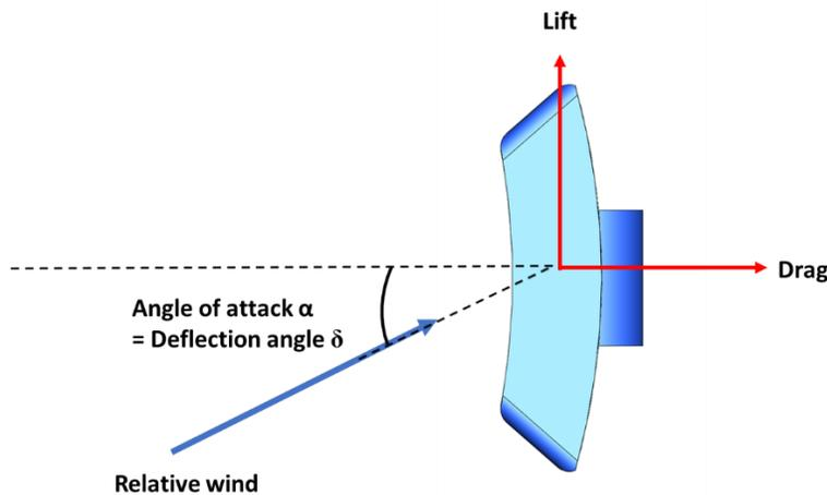
Figure 2-37 Grid Fin Fixed Geometry Approach
