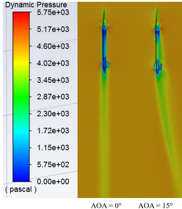
Figure 4-26 The Dynamic Pressure Contours at 280 ft/s
