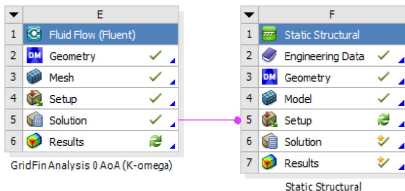
Figure 2-53 Fluent Aerodynamic Model Import to Ansys Structural
