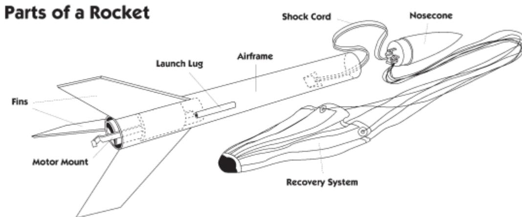
Figure 1-2 Parts of a Rocket [2] © National Association of Rocketry 2020
