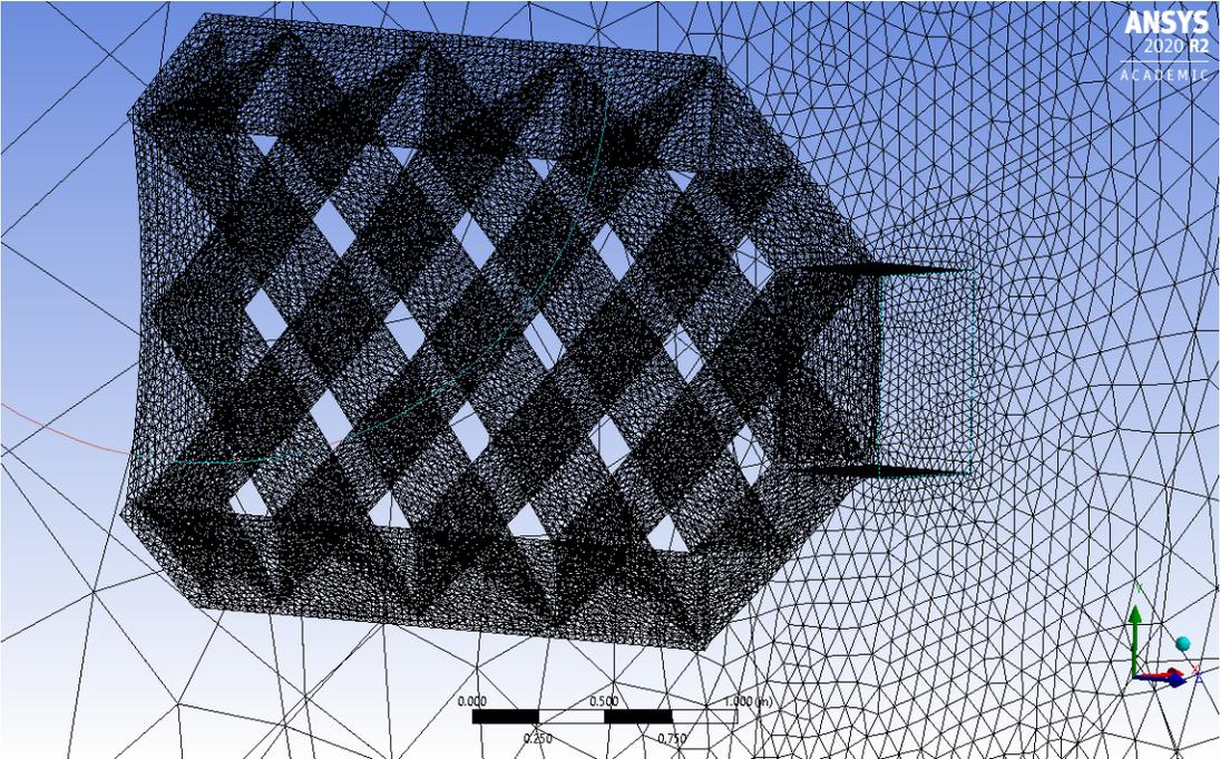
Figure 2-40 Grid Fin Domain Geometry Mesh, Detailed
