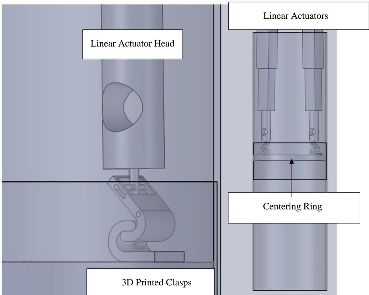
Figure 3-8 Mechanical Separation System SOLIDWORKS Model
