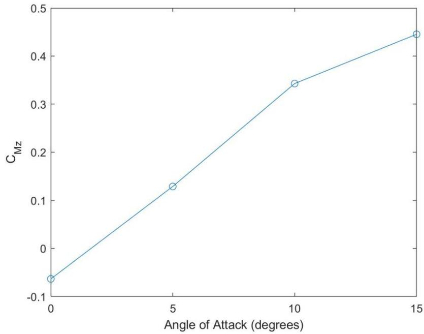
Figure 7-15 Plot of Z Moment Coefficient as a Function of Angle of Attack
