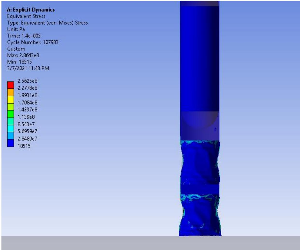
Figure 2-28 von-Mises Stress, 10m/s Impact Landing, Cross Section
