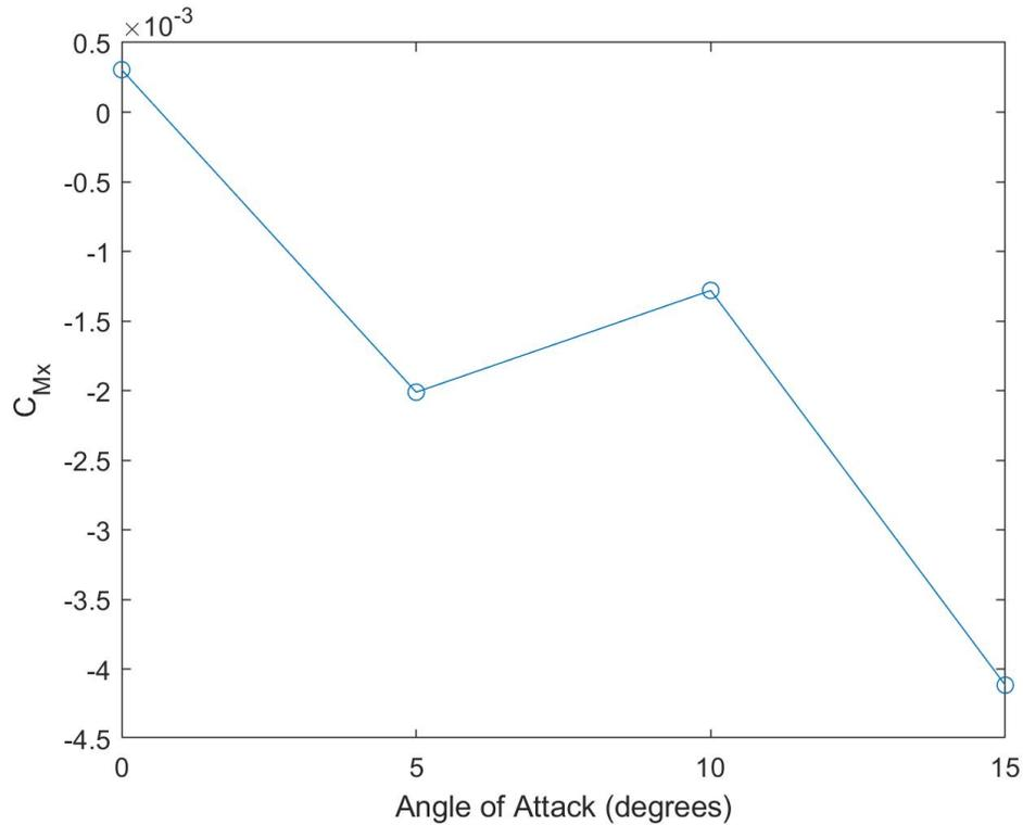
Figure 4-25 Plot of X Moment Coefficient as a Function of Angle of Attack
