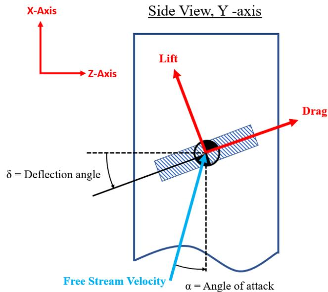
Figure 1-15 Forces on a Single Grid Fin, Y-axis Side View
