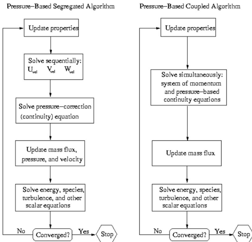
Figure 2-22 Overview of the Pressure-Based Method [76] © Ansys 2020
