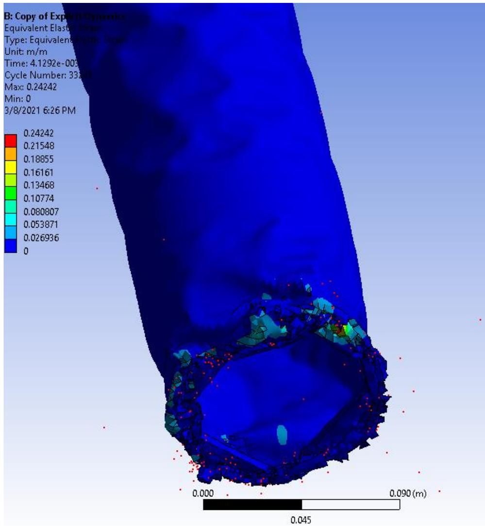
Figure 2-31 von-Mises Strain, 58m/s Impact Landing
