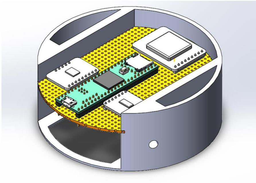
Figure 4-3 Isometric View of the Avionics Bay.
