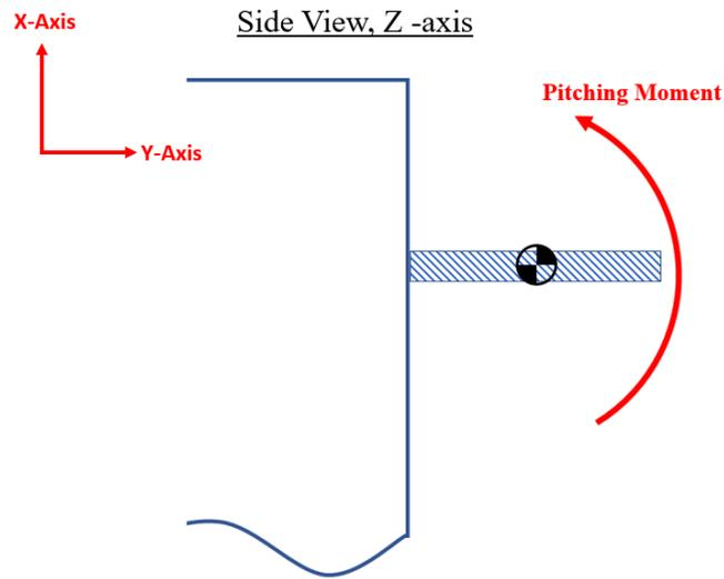
Figure 1-16 Moments on a Single Grid Fin, Z-axis Side View
