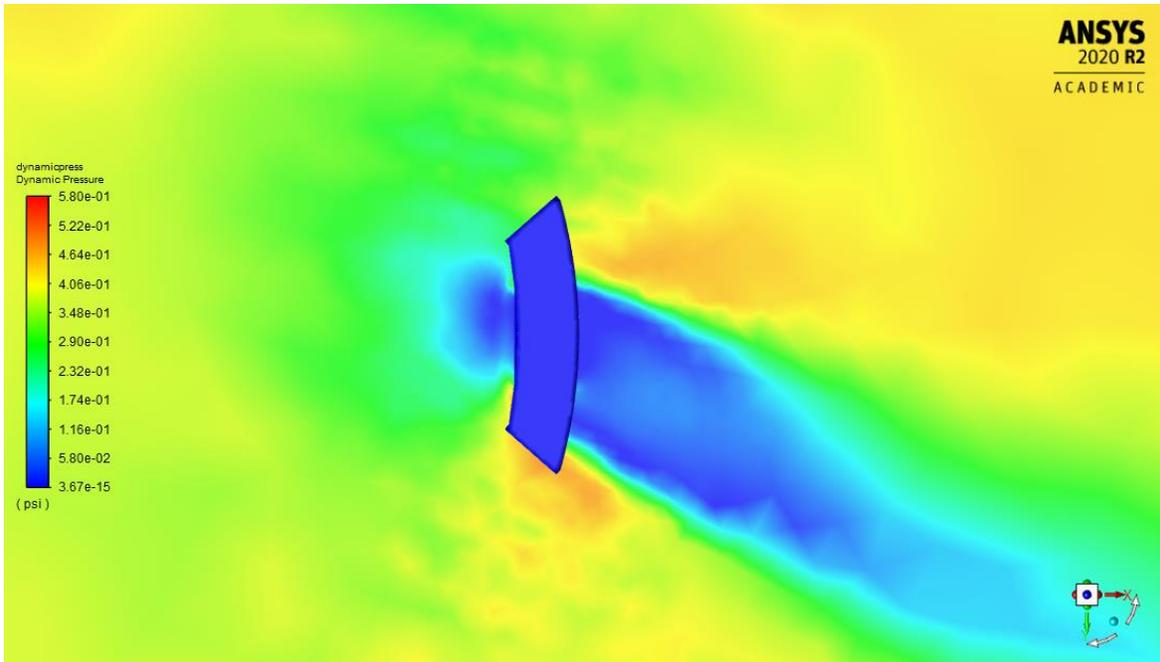
Figure 2-50 Dynamic Pressure Contour, Grid Fin  $\alpha = 20$  degrees at hinge ( $Z=0$ ) plane
