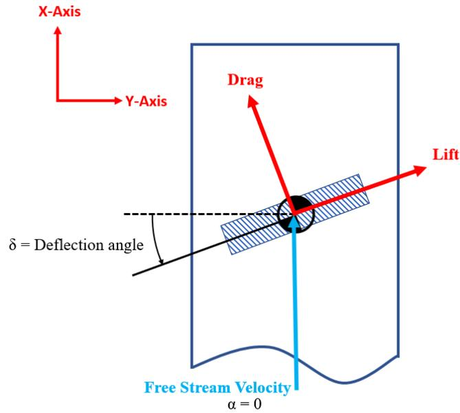
Figure 2-35 Grid Fin Components, Rocket Coordinates
