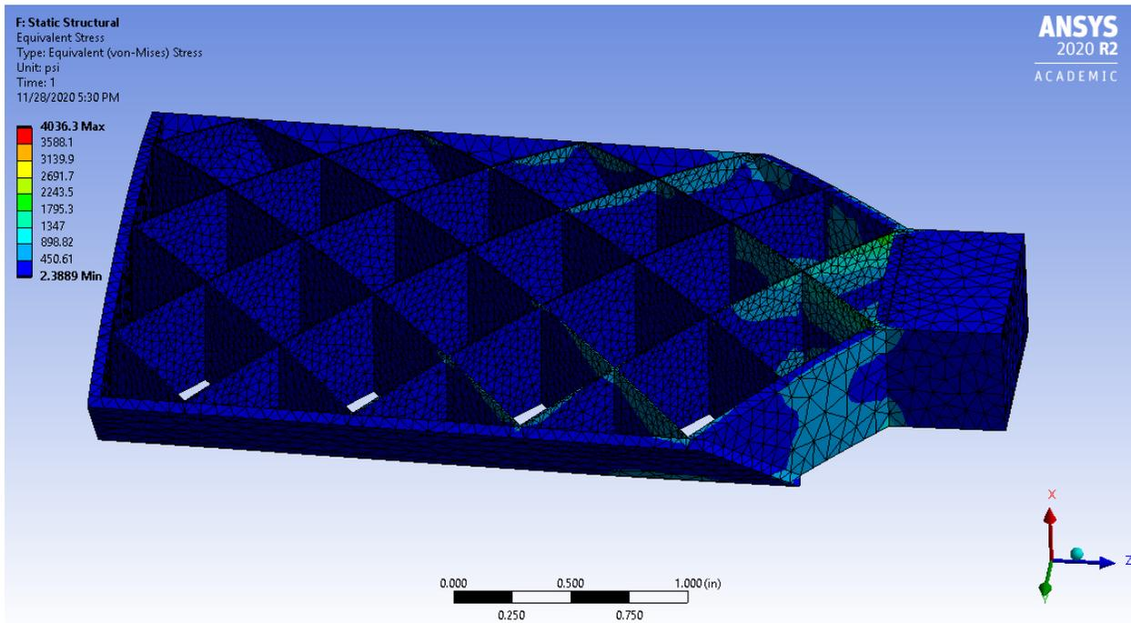
Figure 2-56 von-Mises Equivalent Stress on Grid Fin
