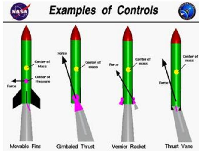
Figure 1-31 Common Methods of Attitude Control [50] © NASA 2014
