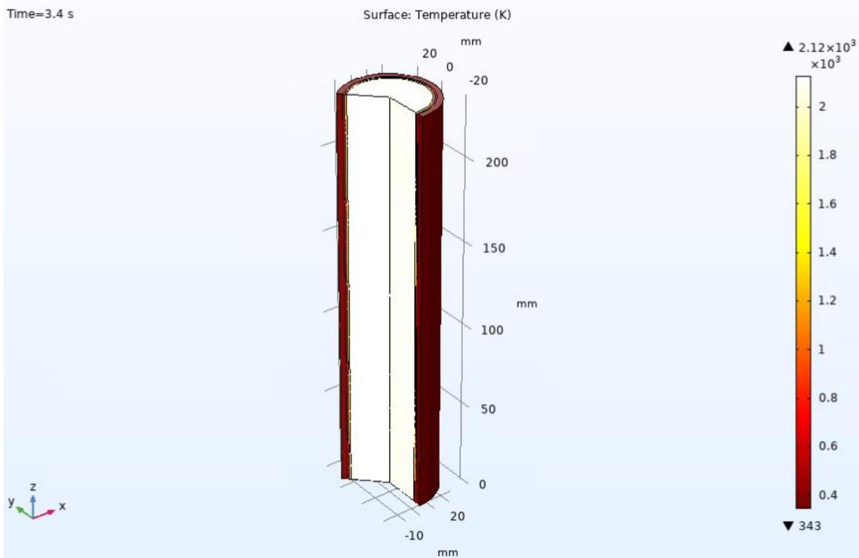
Figure 3-11 Motor temperature distribution at  $t = 3.4$  s
