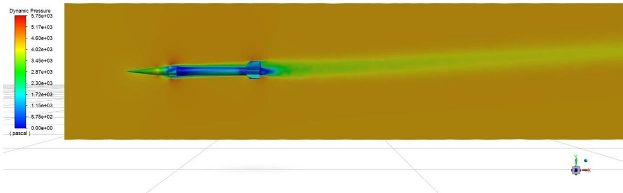
Figure 7-17 Dynamic Pressure Contour at AOA 5 deg
