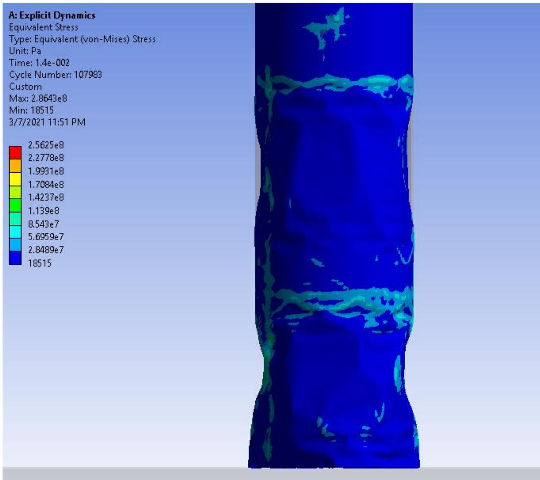
Figure 2-29 von-Mises Stress, 10m/s Impact Landing
