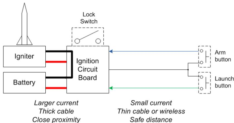
Figure 1-22 Rocket Ignition System Used on Launch Pad [36] © Robot Room 2020
