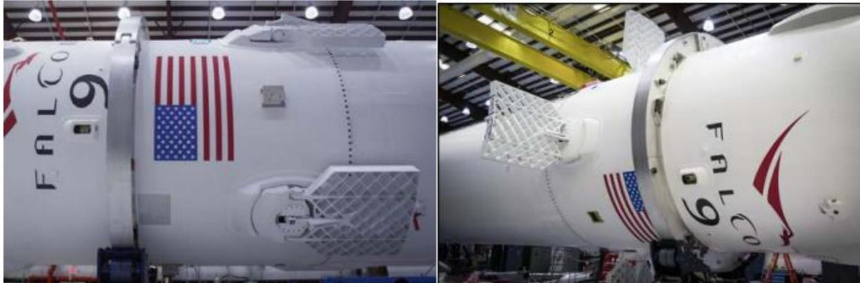
Figure 1-13 Falcon 9 Grid Fins. Left: Stowed on Ascent; Right: Deployed for Re-entry © National Academy of Sciences and SpaceX 2020
