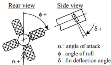
Figure 1-14 Grid Fin Model Angles [20] © ICAS 2010
