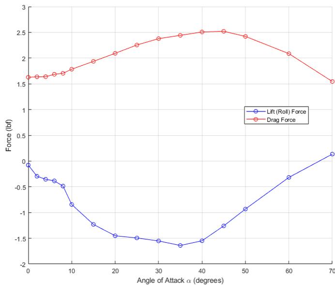
Figure 2-46 Resulting Forces on Rocket, Single Grid Fin
