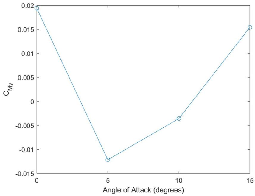
Figure 7-14 Plot of Y Moment Coefficient as a Function of Angle of Attack
