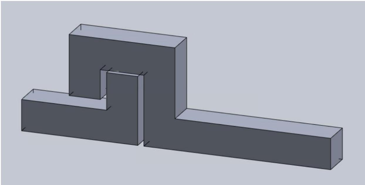
Figure 3-6 SOLIDWORKS Model of Rectangular Clasp (Overall Length of 0.25 in)
