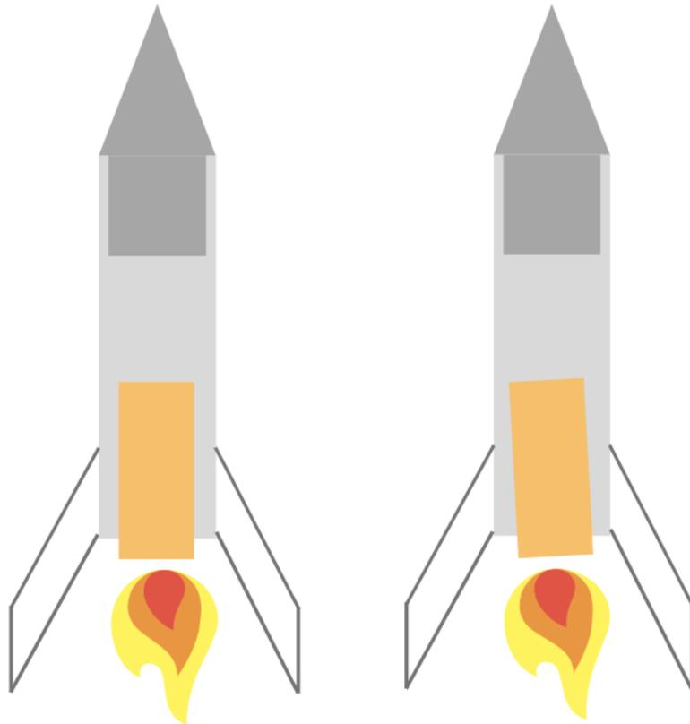
Figure 1-23 Diagram of a Straight Motor (left) Compared With an Angled Motor (right).
