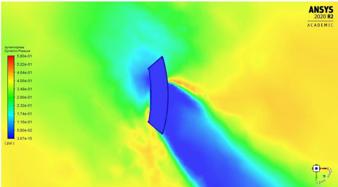
Figure 2-51 Dynamic Pressure Contour, Grid Fin  $\alpha = 45$  degrees at hinge ( $Z=0$ ) plane
