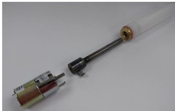
Figure 1-27 Components of the Astrojays' Mounting System © The John Hopkins University 2018
