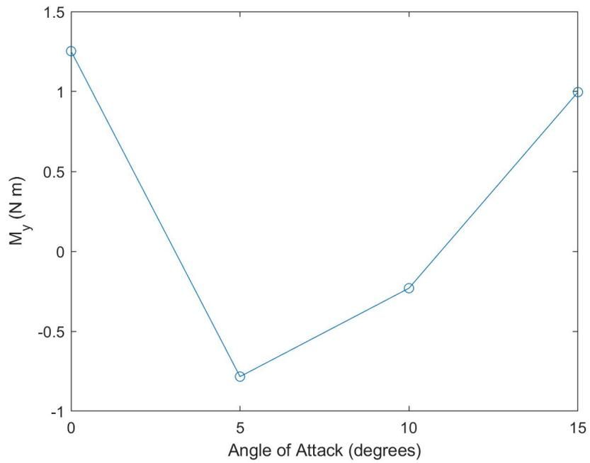
Figure 7-9 Plot of Y Moment as a Function of Angle of Attack
