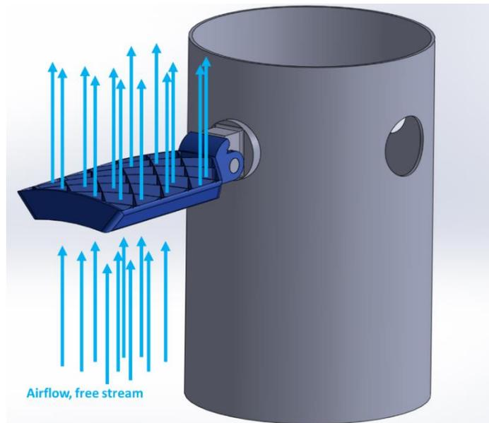
Figure 2-32 Grid Fin Airflow Diagram
