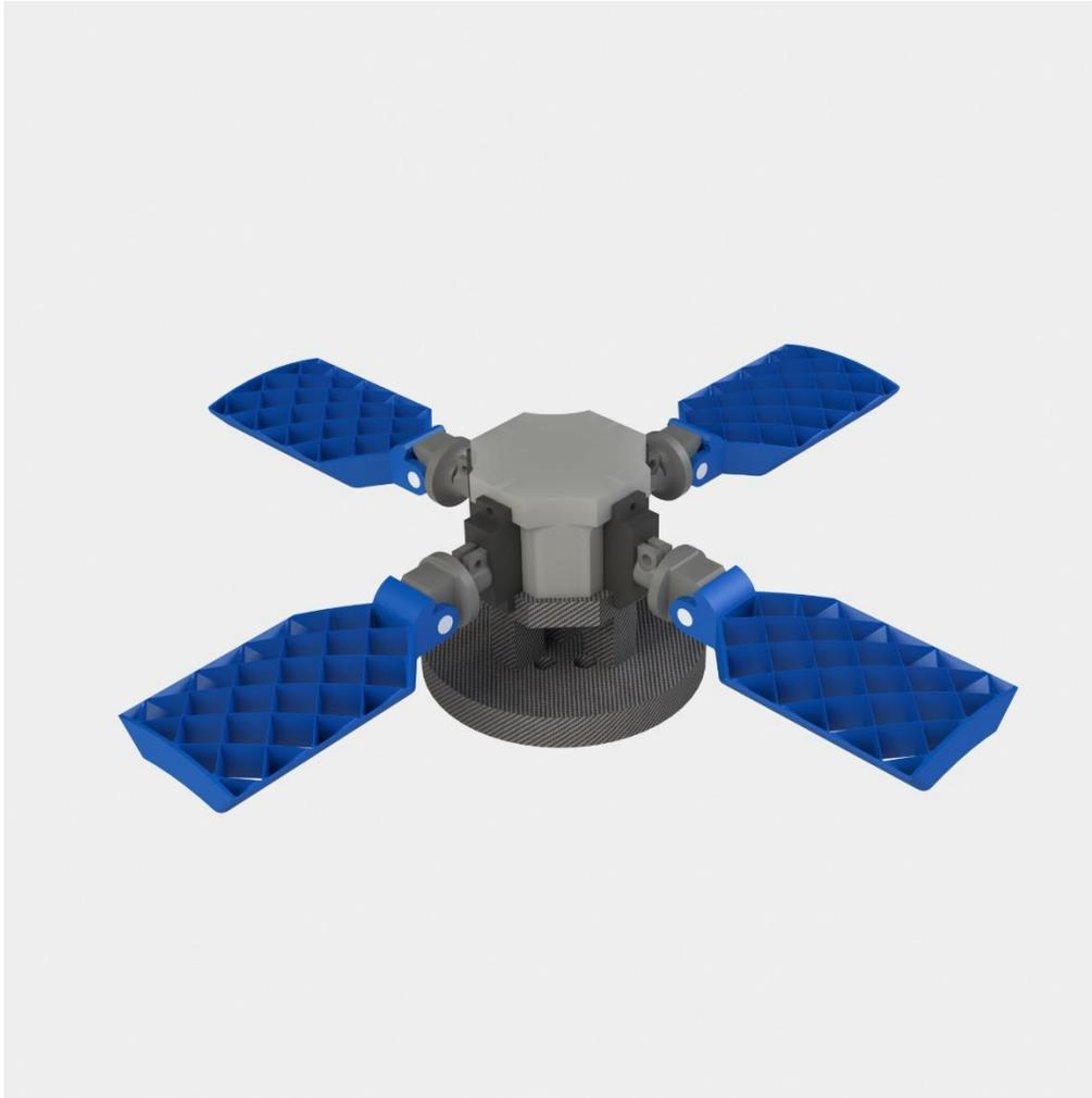
Figure 2-6 Grid Fin System 3D Render
