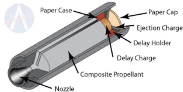
Figure 1-18 Cut-a-way View of a Composite Propellant Motor [30] © Apogee Components 2016
