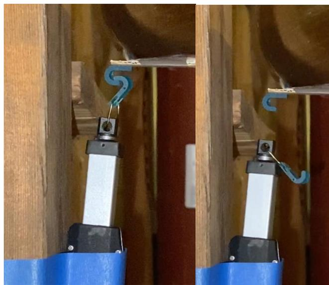
Figure 3-14 Clasp Safety Mechanism Latched and Unlatched
