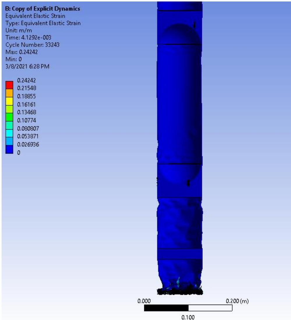
Figure 2-30 von-Mises Strain, 58m/s Impact Landing, Cross Section
