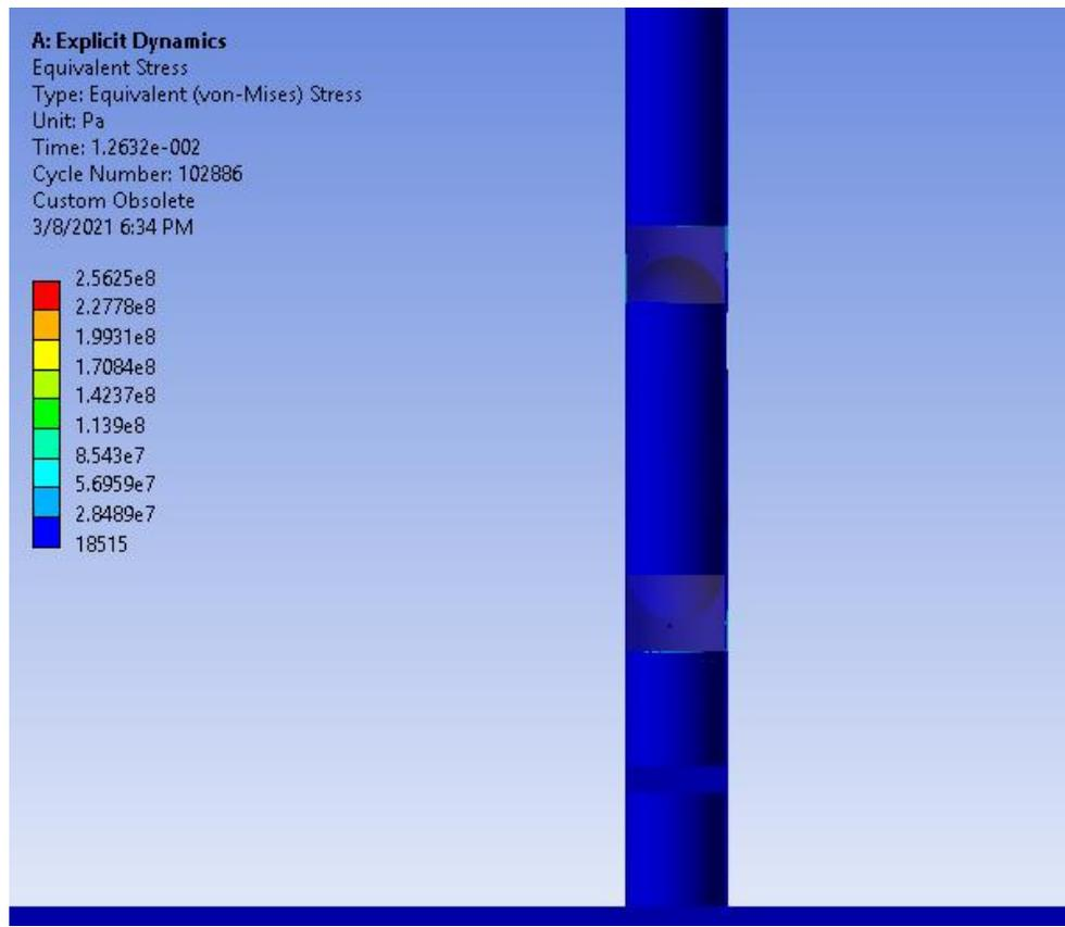
Figure 2-27 von-Mises Stress, 5m/s Impact Landing, Cross Section
