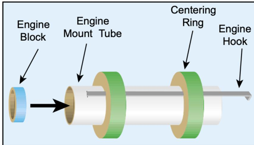
Figure 1-24 Diagram of a Low Power Motor Retention System © Apogee Components 2019
