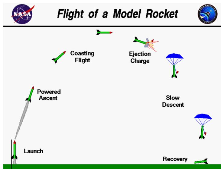
Figure 1-10 Flight of a Standard Model Rocket [1] © NASA 2020
