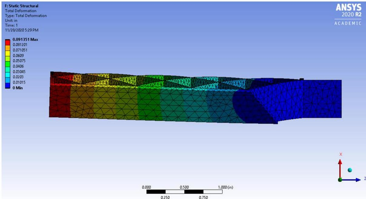
Figure 2-55 Deformation on Grid Fin (Side View)
