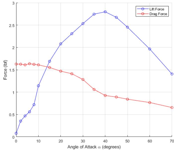
Figure 2-45 Lift and Drag Forces on Grid Fin, Fluent Results
