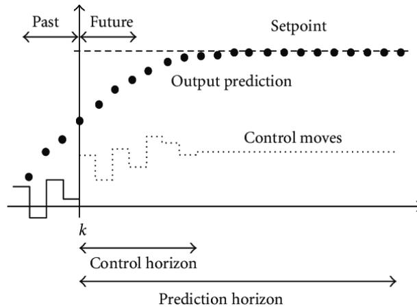
Figure 1-33 An Example of the Future State and Control Input Predictions of an MPC Controller
