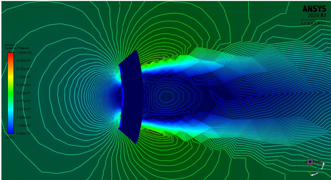
Figure 2-43 Grid Fin Dynamic Pressure Contours, Initial Fluent Run,  $\alpha = 0$
