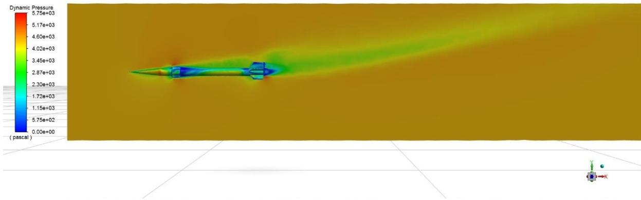
Figure 7-19 Dynamic Pressure Contour at AOA 15 deg
