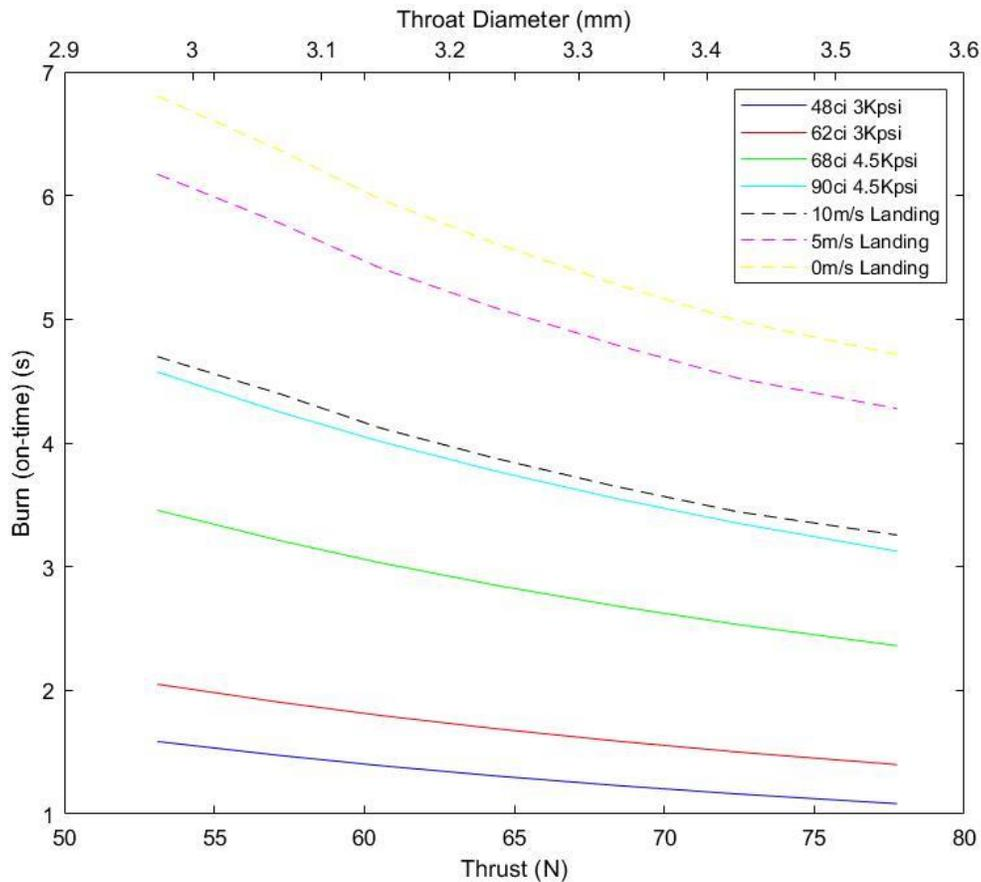
Figure 3-16 Thrust vs. Burn Time
