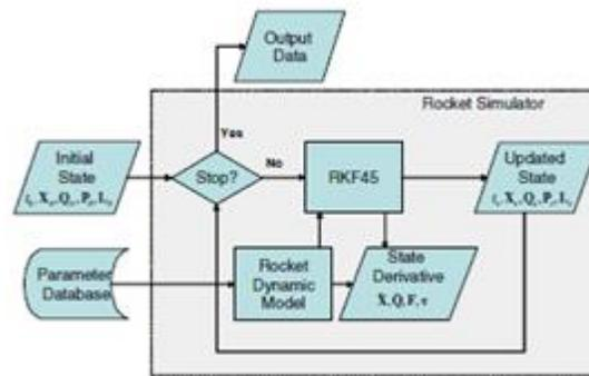
Figure 1-37 A Block Diagram of a Dynamical Simulation of a Rocket [57] © American Society of Civil Engineers 2010
