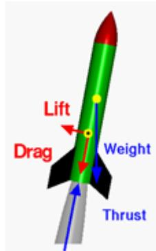
Figure 1-29 Four Forces of Rocket Flight [42] © NASA 2014
