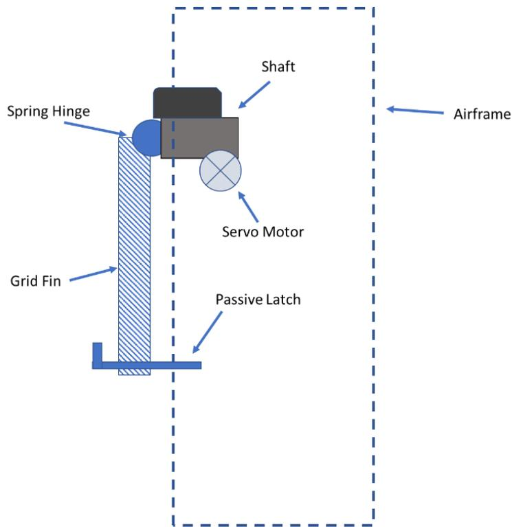
Figure 2-7 Single Grid Fin Overview, Stowed on Ascent
