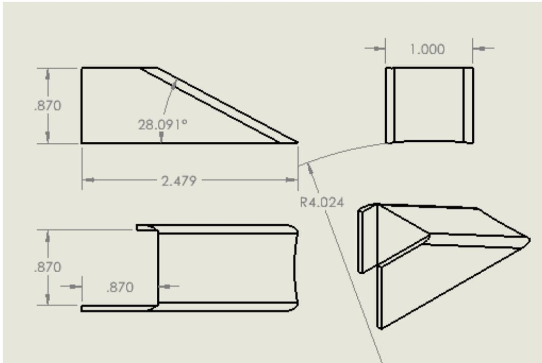
Figure 2-18 Camera Fairing Dimensions (in inches)
