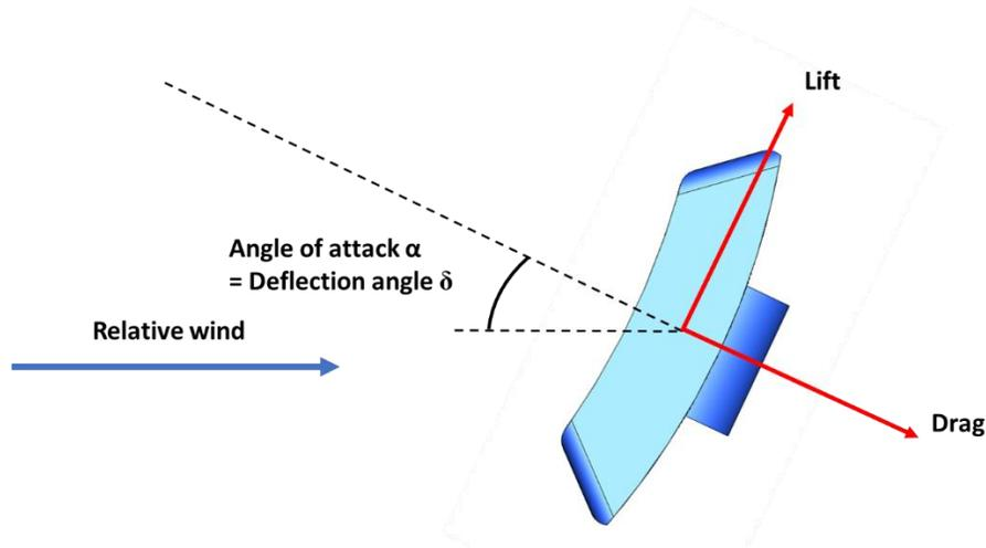
Figure 2-34 Grid Fin Lift and Drag Vectors
