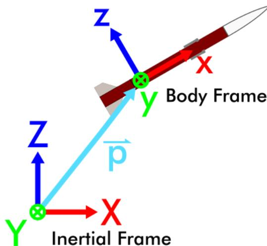
Figure 4-6 The I and B coordinate frames.
