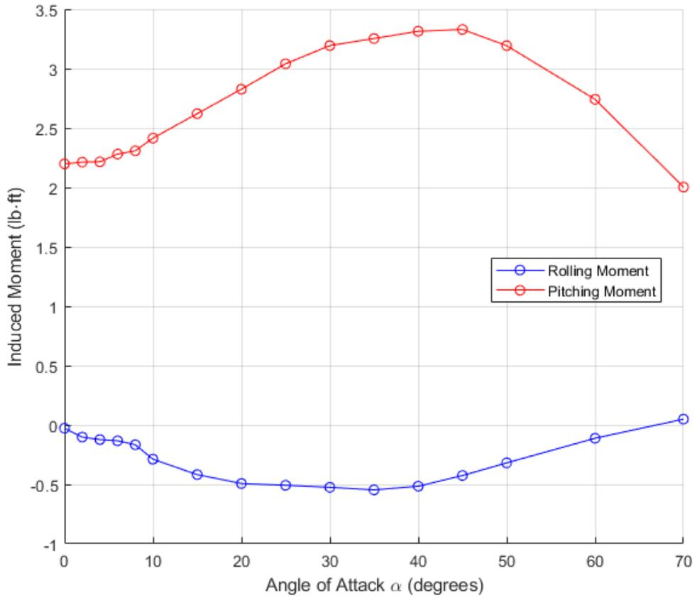
Figure 2-47 Resulting Moments on Rocket, Single Grid Fin
