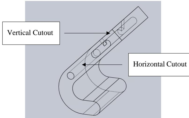
Figure 3-7 Upper Clasp Cross-Sectional Area Illustrating Cutouts for Linear Actuator
