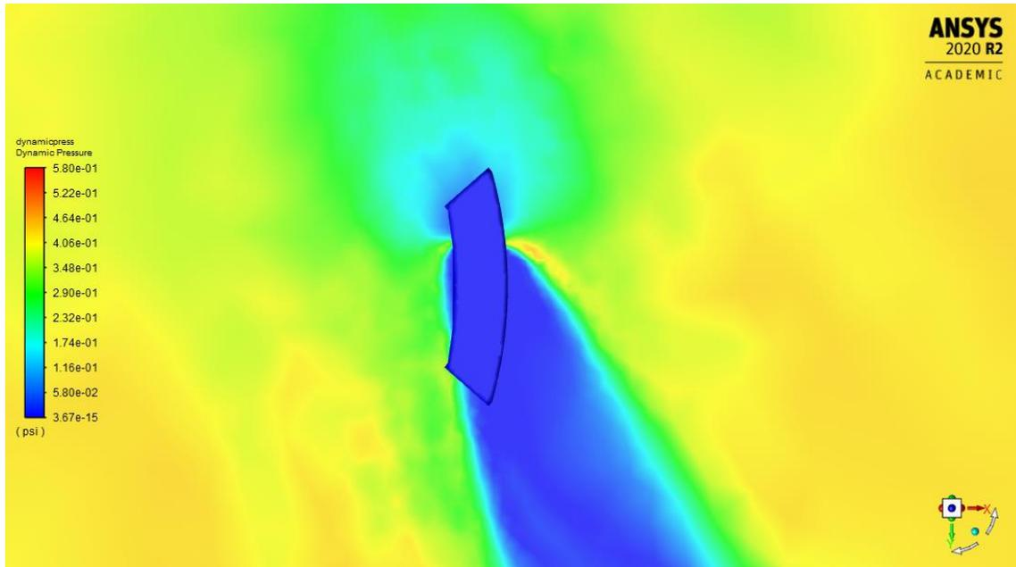
Figure 2-52 Dynamic Pressure Contour, Grid Fin  $\alpha = 70$  degrees at hinge ( $Z=0$ ) plane
