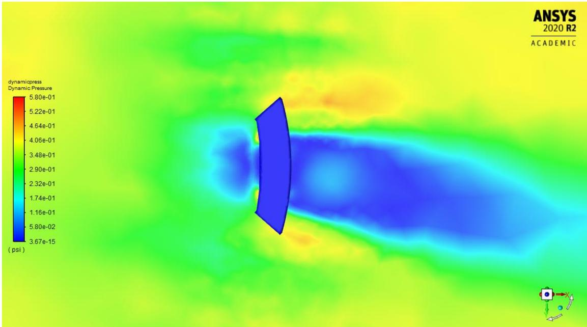
Figure 2-49 Dynamic Pressure Contour, Grid Fin  $\alpha = 6$  degrees at hinge ( $Z=0$ ) plane
