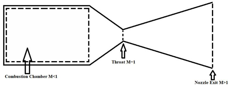
Figure 1-28 Converging Diverging Nozzle
