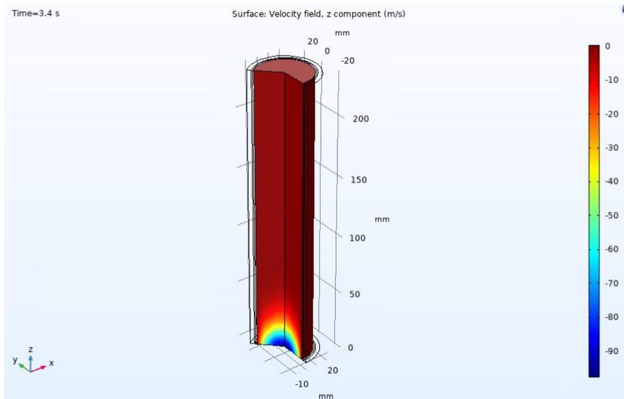
Figure 3-12 Velocity distribution in the motor at  $t = 3.4$  s
