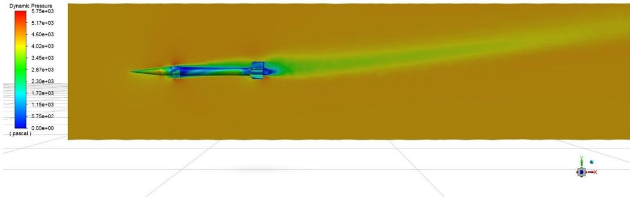
Figure 7-18 Dynamic Pressure Contour at AOA 10 deg
