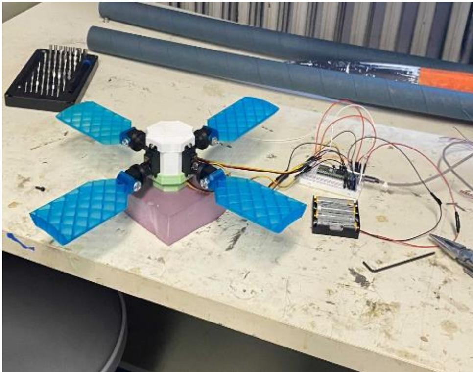
Figure 2-15 Grid Fin System, Assembled
