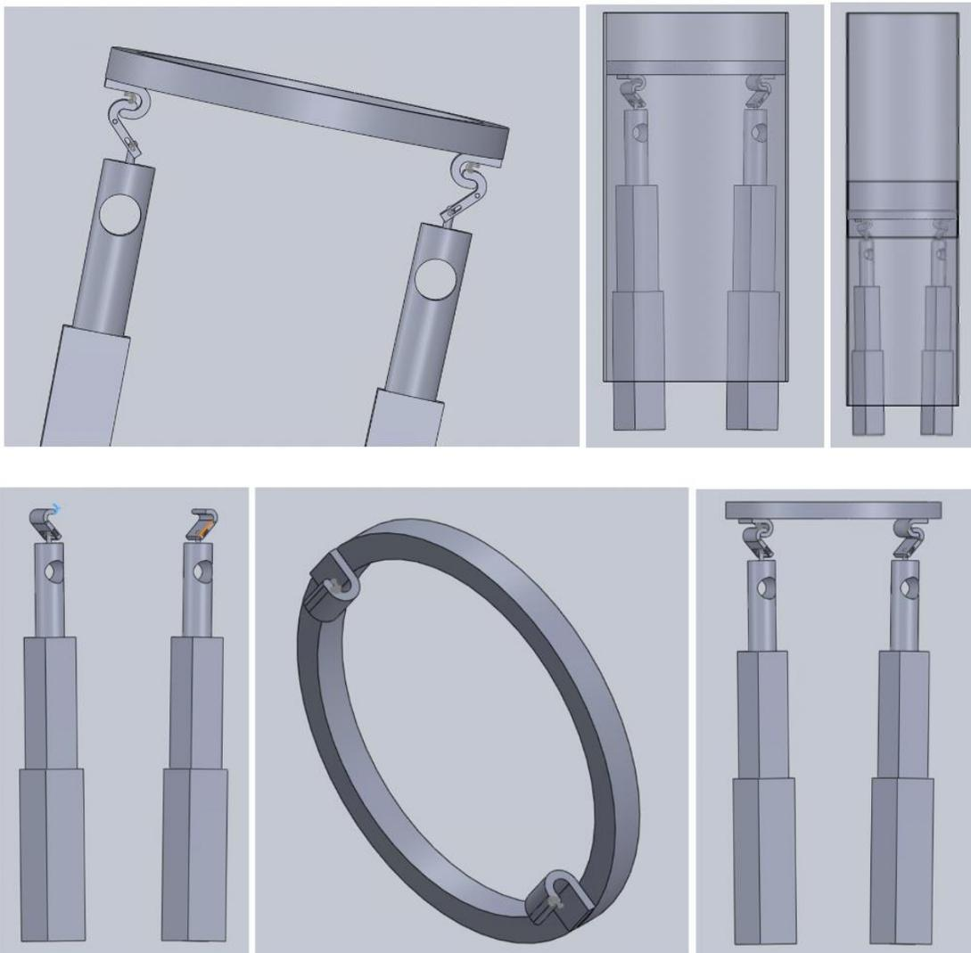
Figure 3-15 Assembly of Separation System
