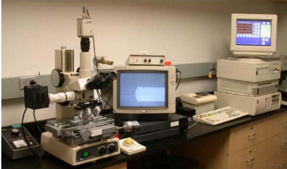
Figure 33. The measurement setup used for determining dimensions of the cantilevers.
