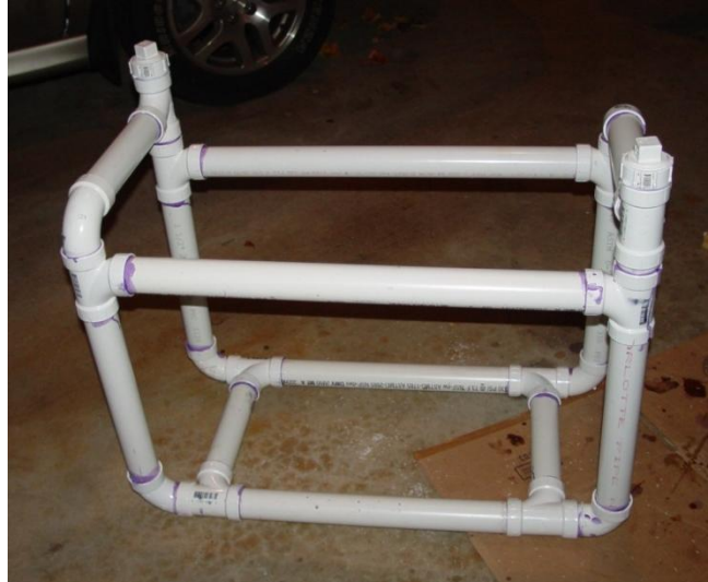
Figure 16: Final PVC piping frame for Connecticut apparatus
