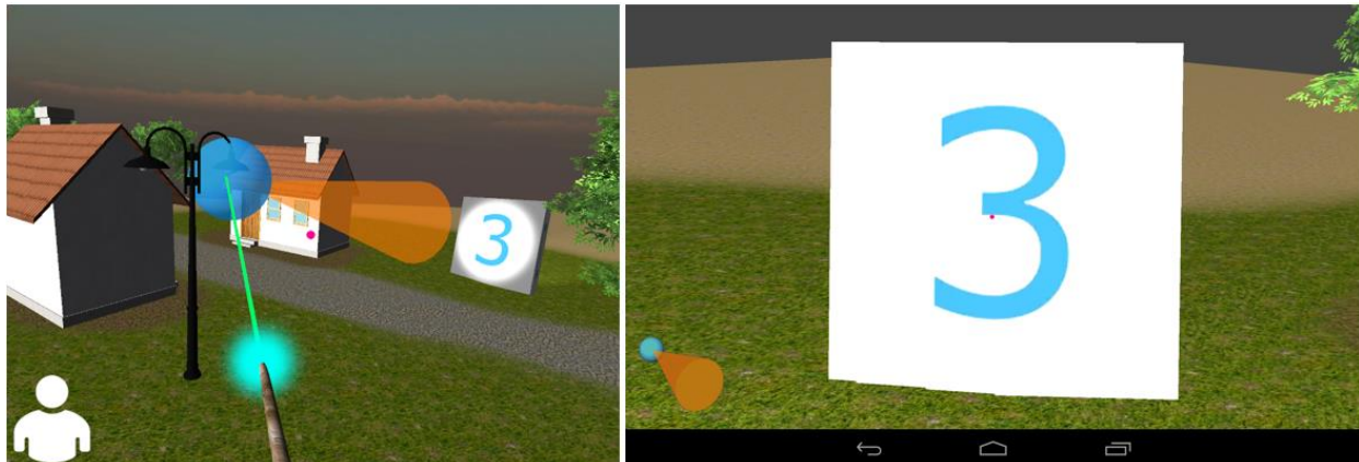
Figure 1.5: The object impersonation technique allows an immersed user to select and become an object to manipulate it from the inside, such as orienting a spotlight on a target by looking at the target from the light's own point of view. [Wang15].
