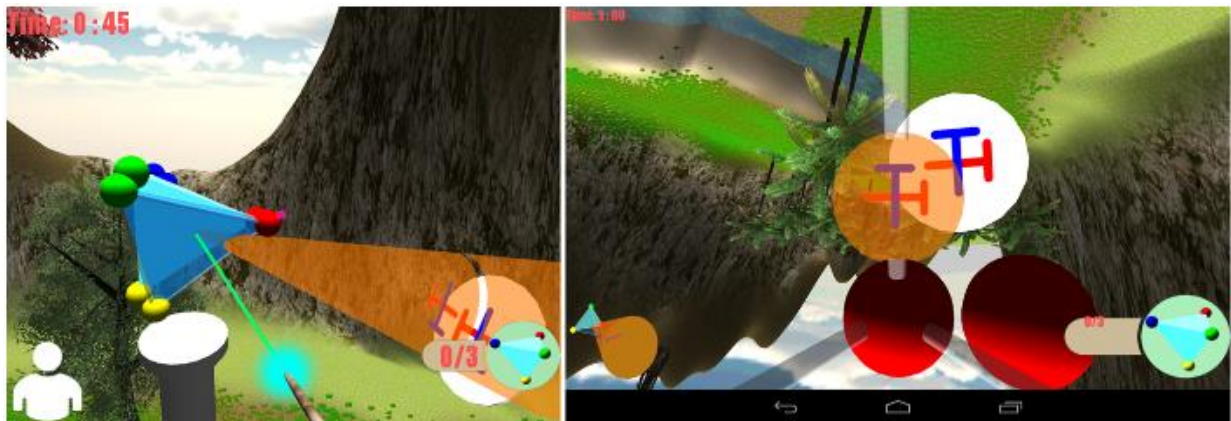
Figure 4.4: The tetrahedron alignment task is a classic 6-DOF object manipulation task. Using object impersonation, the 3-DOF rotation control can be decomposed to simpler looking and rolling actions.
