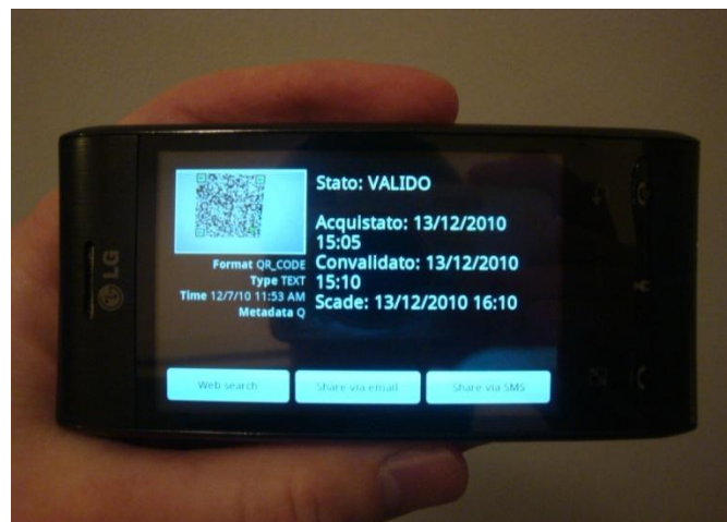
Figure 70 - An example of what the vaporetto attendant might see after scanning a ticket on the application.
