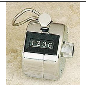
Figure 38 – A mechanical clicker used for counting pedestrians
