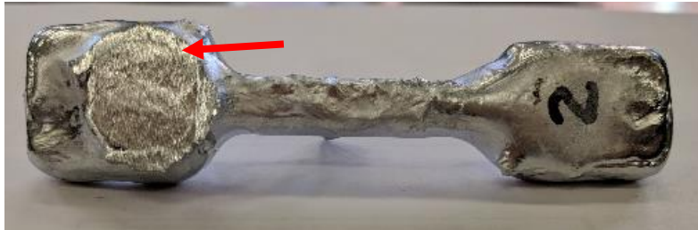
Figure 6: Aluminum tensile bar hot dipped in a zinc melt.
