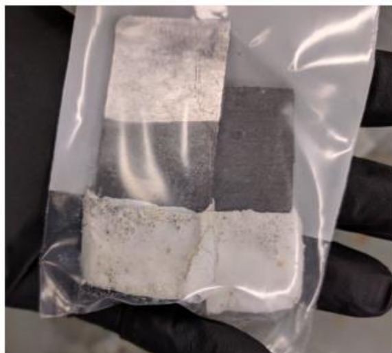
Figure 34: The result of an attempt to electroplate cerium onto A356 from a eutectic salt at 450°C for 60s. The white coating is the solidified eutectic salt.
