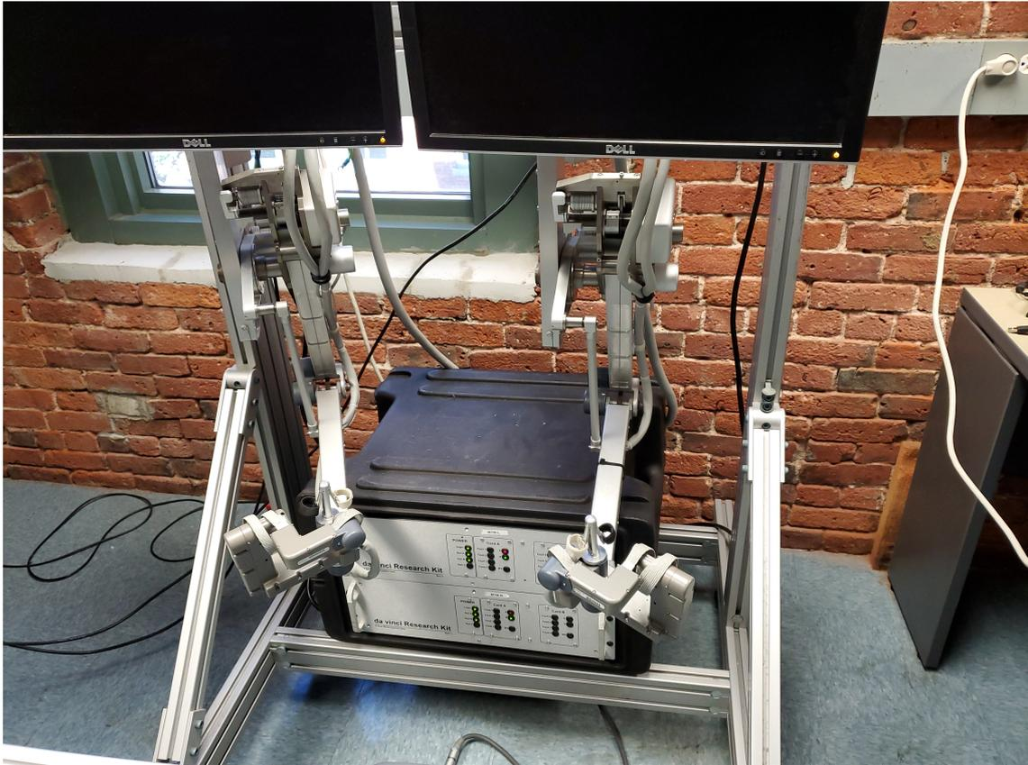
Figure 1.3: da Vinci Research Kit system Master Tool Manipulators (MTM)
