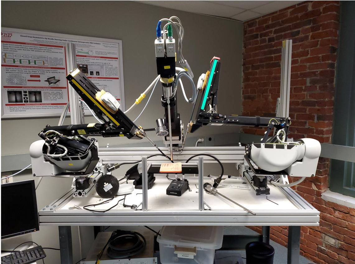
Figure 1.2: da Vinci Research Kit system with a pair of Patient Side Manipulators (PSM) and an Endoscopic Camera Manipulator (ECM)
