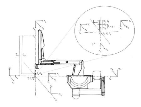
Figure 7.1: PSM DH Frame Assignments [11, 33, 39]
