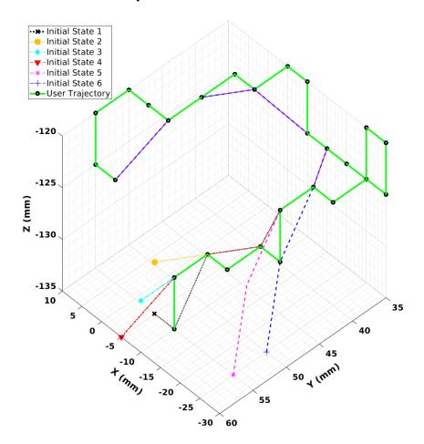
Figure 5.4: Trajectory followed by PSM after change in the initial state based on the learnt RL policy
