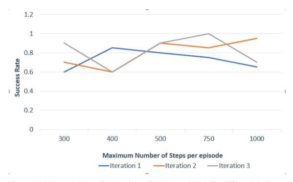
Figure 5.10: Success Rate of 3 Iterations of PSM Reach Task for different Maximum Number of Steps per Episode (Model 3). Each iteration consisted of 20 trials to reach the goal position.
