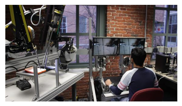
Figure 1.1: Operator using the dVRK system to perform hand-off suturing task
