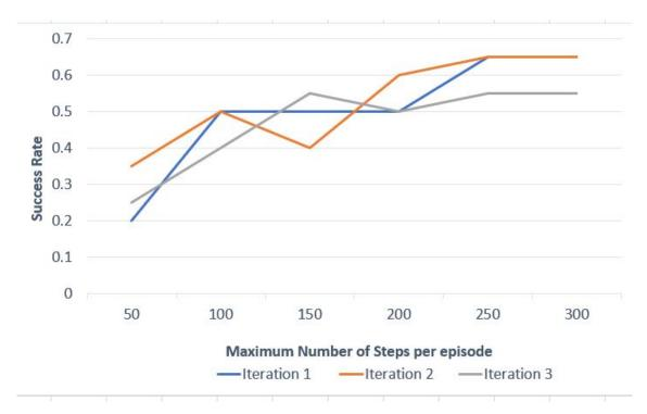
Figure 5.5: Success Rate of 3 Iterations of PSM Reach Task for different Maximum Number of Steps per Episode (Model 1). Each iteration consisted of 20 trials to reach the goal position.
