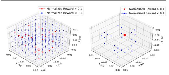
Figure 4.2: Comparison of reward functions obtained for an user using IRL with value iteration (left) and sparse reward with *Q*-learning (right). The size and color of the dots indicate the rewards received by the PSM for visiting the corresponding states in the grid world.
