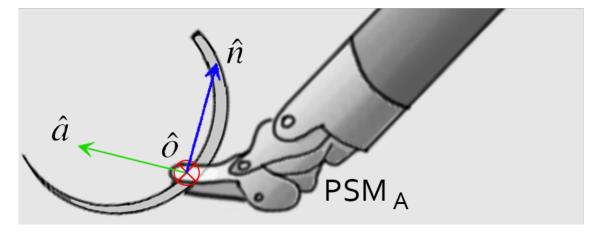
Figure 4.3: Transformations between World,  $PSM_M$ ,  $PSM_A$  and Needle frames.
