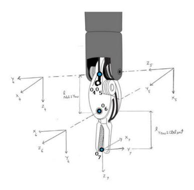
Figure 7.2: PSM Instrument DH Frame Assignments [11, 33, 39]
