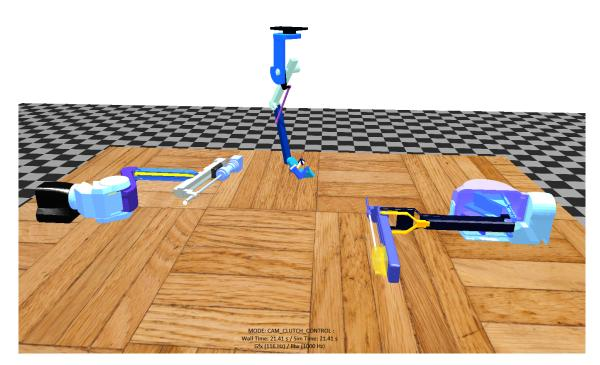
Figure 3.2: dVRK system simulated in AMBF (ECM (left), MTM (center), PSM(right))
