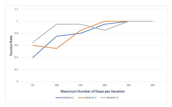
Figure 5.8: Success Rate of 3 Iterations of PSM Reach Task for different Maximum Number of Steps per Episode (Model 2). Each iteration consisted of 20 trials to reach the goal position.
