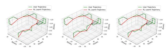
Figure 5.3: Learnt RL and discretized user trajectory for 3 different computed policies with DTW to measure similarity
