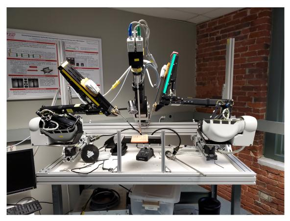
Figure 1.2: da Vinci Research Kit system with a pair of Patient Side Manipulators (PSM) and an Endoscopic Camera Manipulator (ECM)
