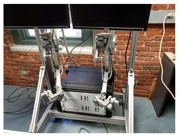
Figure 1.3: da Vinci Research Kit system Master Tool Manipulators (MTM)
