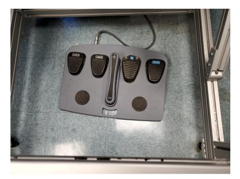
Figure 1.4: da Vinci Research Kit system User Foot Pedal
