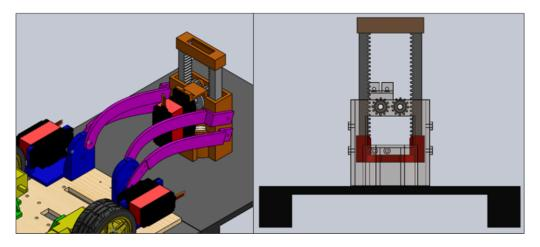
Figure 3.3: CAD models of four-bar linkage (left) and linear actuator (right)
