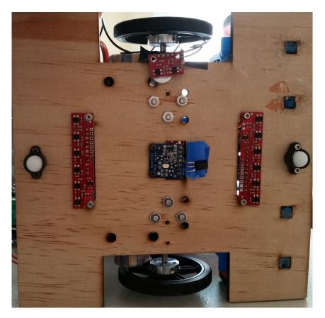
Figure 3.5: 12 light sensor setup in two arrays of 6
