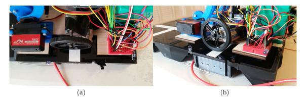
Figure 3.8: 2-way IR communication between block and robot with IR LEDs and TSOP sensor of scaffolding block shown
