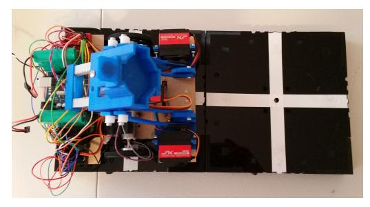
Figure 4.3: Two block inter-block navigation test
