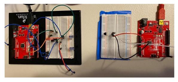
Figure 4.5: IR communication unit test setup of IR LED sending signals directly facing a TSOP38328 sensor
