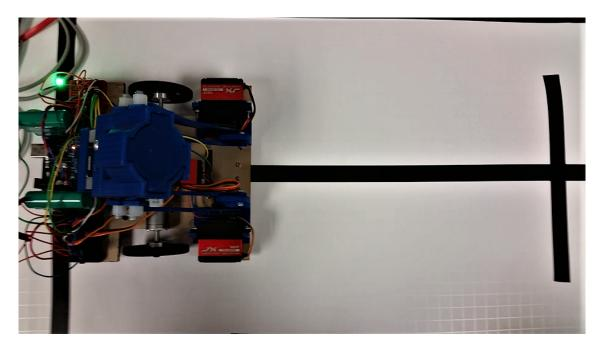
Figure 3.6: Line following test pad for developing error-correction Lookup Table
