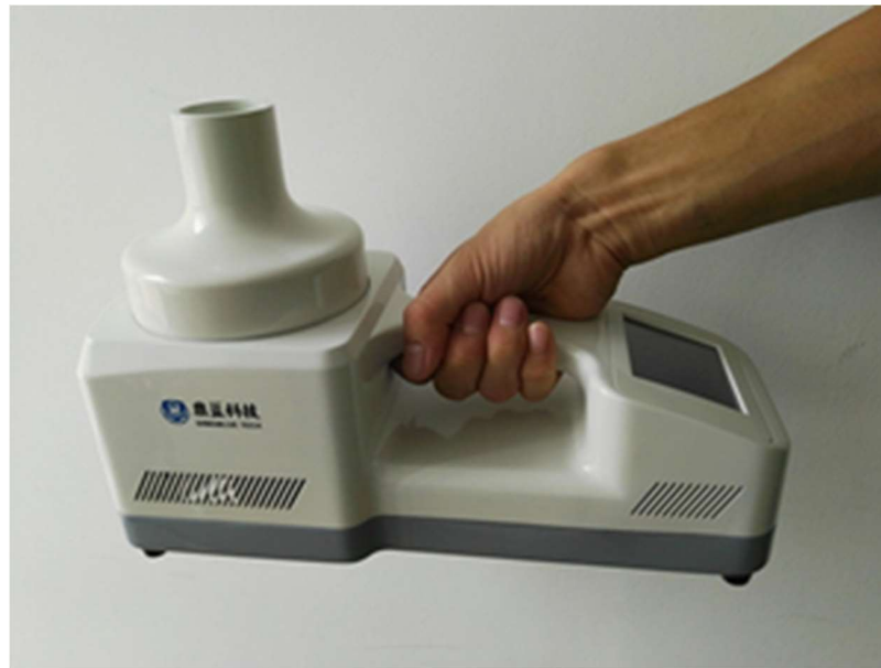
Figure E.3: The BioTrap pictured above (Beijing Dingblue Technology, 2017). The nozzle on the top left can be removed and beneath is it the sample stage on which the agar is placed. On the right is the touch screen which is where the on/off buttons and start buttons are.
