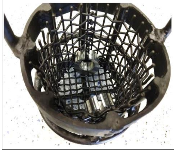
Figure 8: Setup of Navy C-ring and CHTE quench probe before heat treatment.
