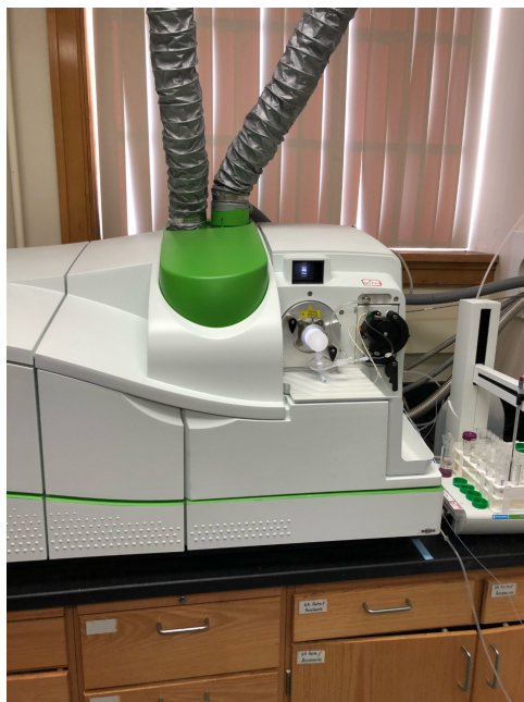
Figure 11: Inductively Couple Plasma to measure copper concentration of each sample
