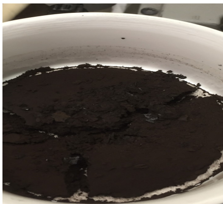
Figure 4: Hydrochar on filter paper on top of Buchner funnel after vacuum filtering
