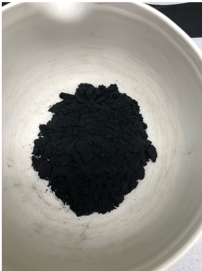
Figure 13: Vinyl sulfonic acid char after taking it out of the 65°C oven
