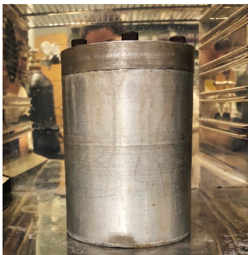
Figure 1: Autoclave in an oven that has Teflon reactor and glucose-water solution inside it
