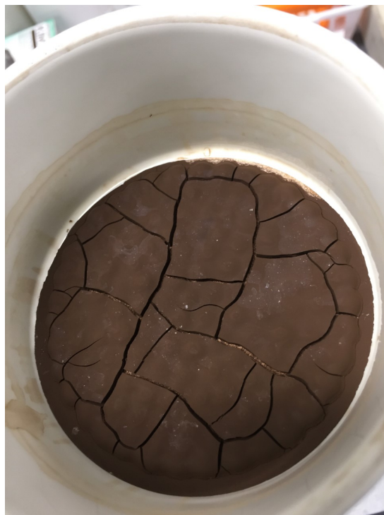
Figure 12: Acrylic acid char after vacuum filtering
