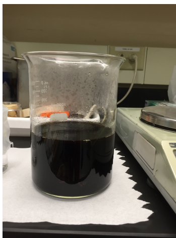
Figure 7: Hydrochar washed with potassium hydroxide solution
