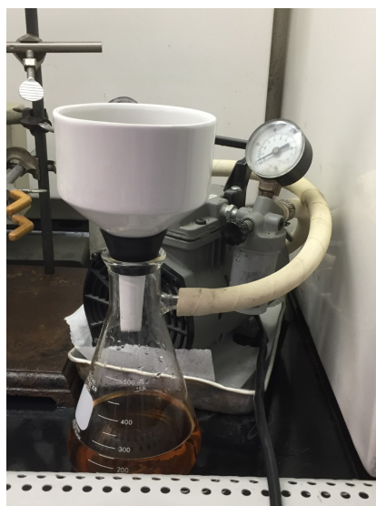
Figure 3: Vacuum filtering slurry and ethanol-water solution
