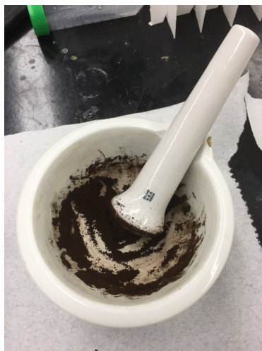
Figure 6: Hydrochar grinded up with mortar and pestle
