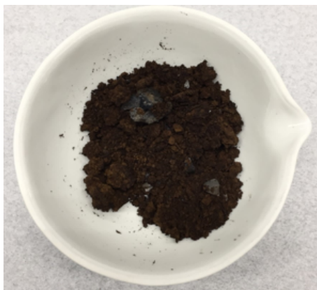
Figure 5: Hydrochar in crucible after being in oven at 65°C for 24 hours
