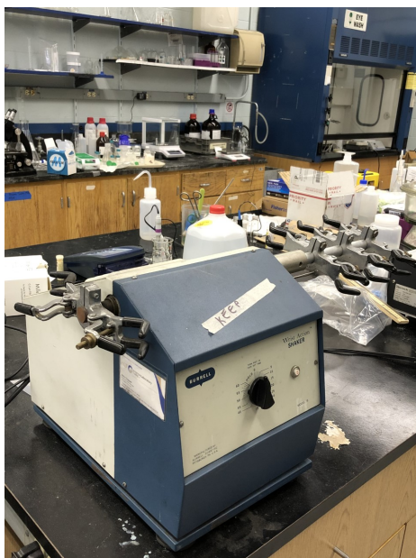
Figure 9: Shaker that shakes the samples for 24 hours
