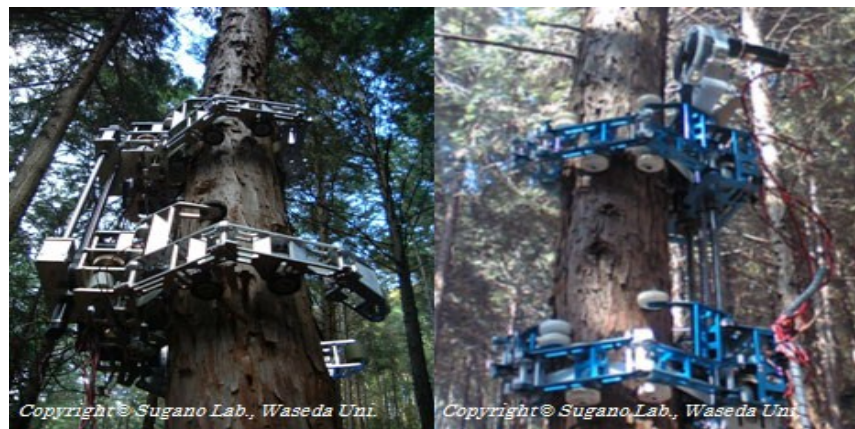
Figure 4: WOODY: "Robot Assisting Forestry Work"
