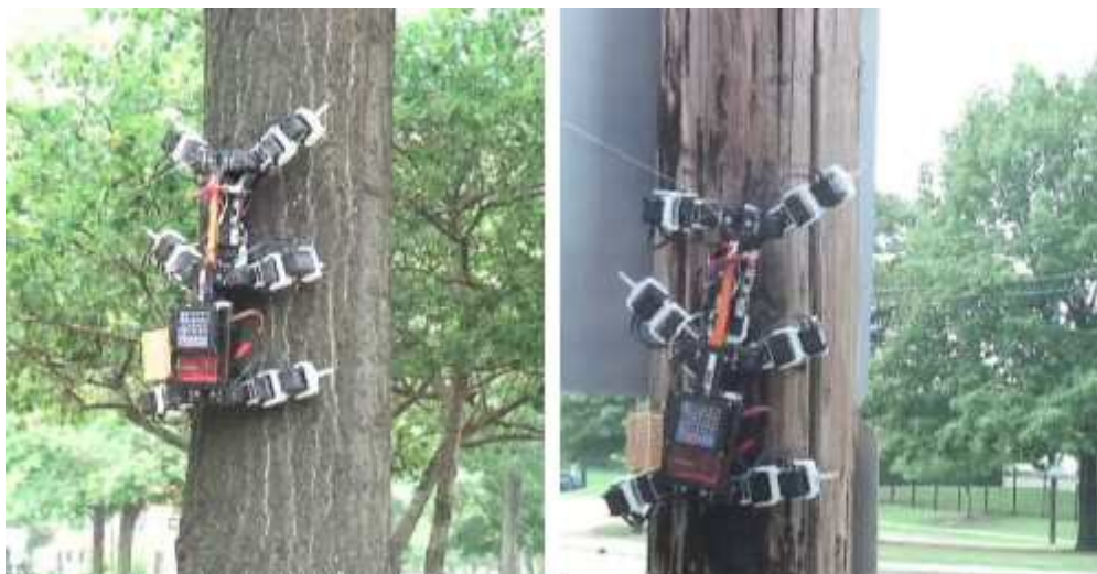
Figure 14: DIGbot climbing up a tree (left) and a telephone pole (right)
