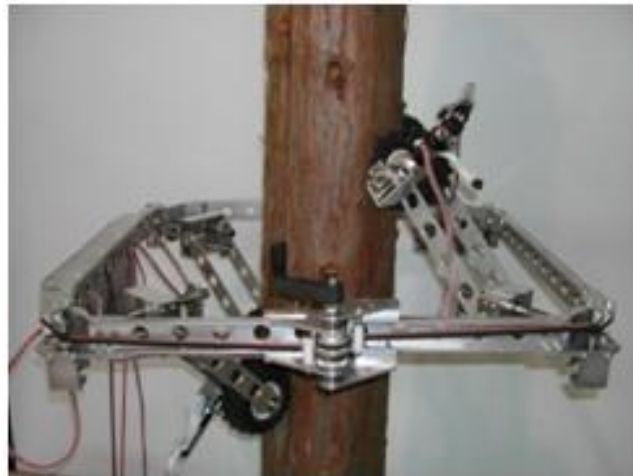
Figure 6: Kawasaki's Tree Pruning Robot at Gifu University, Japan
