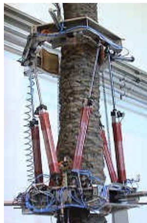
Figure 8: TREPA Robot Climbing a Tree Trunk
