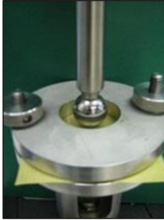
Figure 66: Ball Burst Testing Fixture (Washington University School of Medicine in St. Louis)
