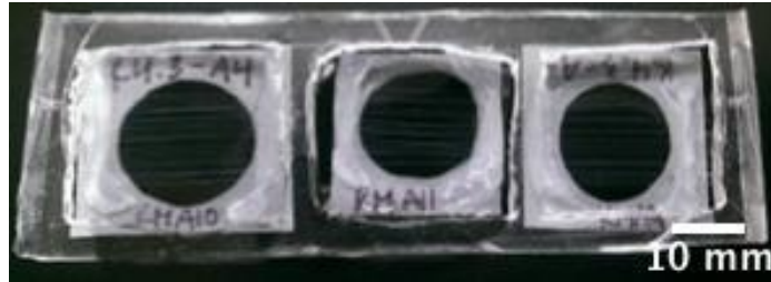
Figure 102: Composite mold with three scaffolds.
