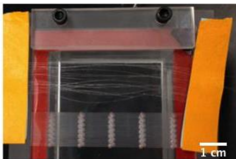
Figure 97: Removal of threads from aligned grooves.
