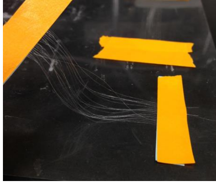
Figure 98: Transfer of aligned threads to transfer paper.
