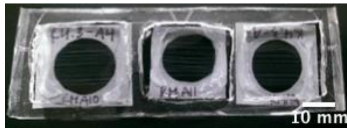
Figure 90: Picture of scaffolds in Composite Frame
