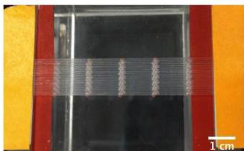
Figure 96: Tape placed on top of threads to secure in alignment.
