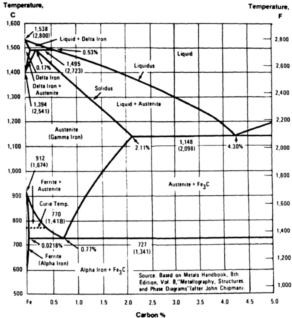
Figure 2: Fe-Fe<sub>3</sub>C equilibrium phase diagram. [7]
