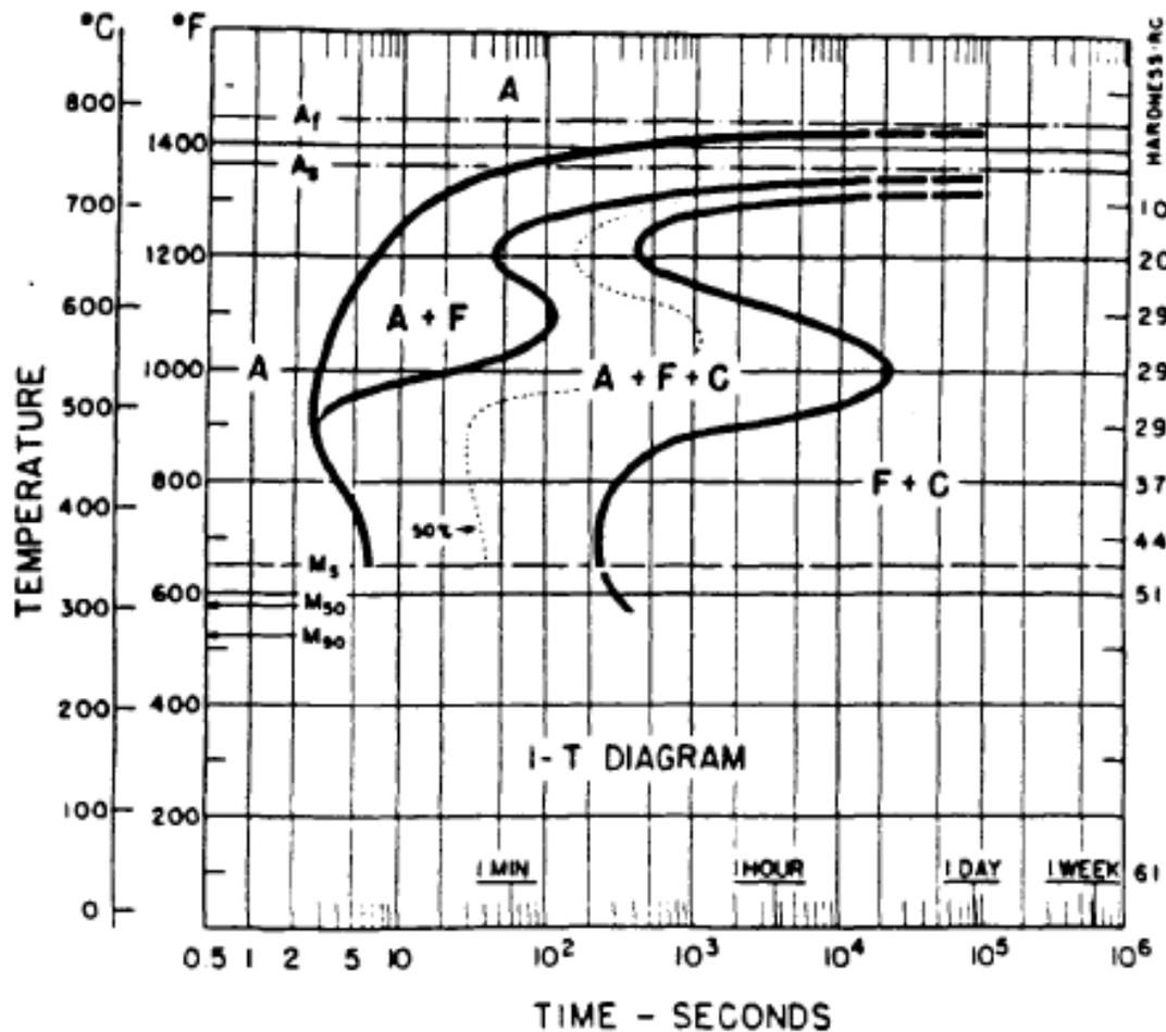
Figure 3: Isothermal transformation diagram for 4140 Steel [7]
