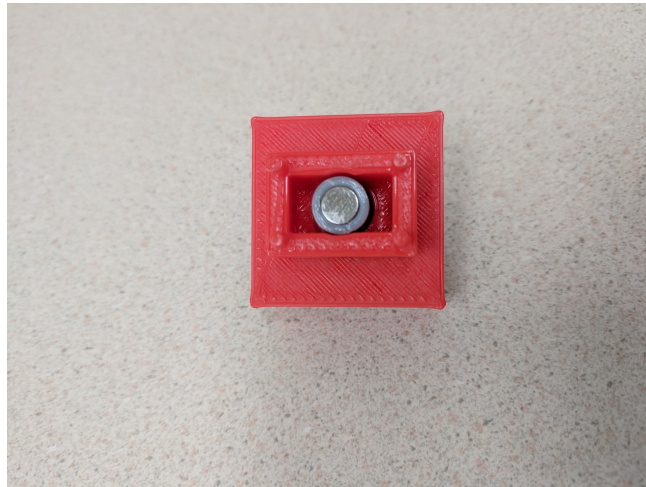
Figure 19: Second Iteration of Encoder Test Rig, Magnet View
