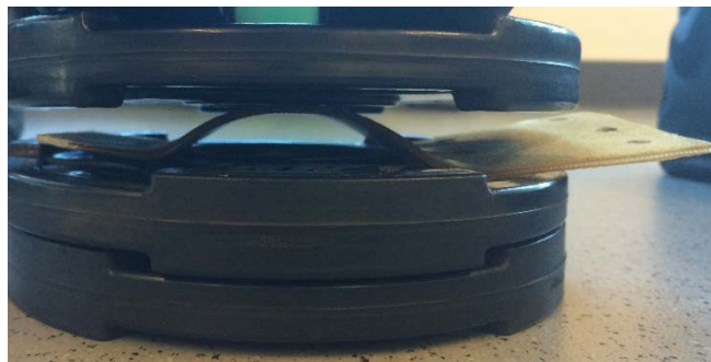
Figure 13: 8 Layer Foot with 90lb. Applied
