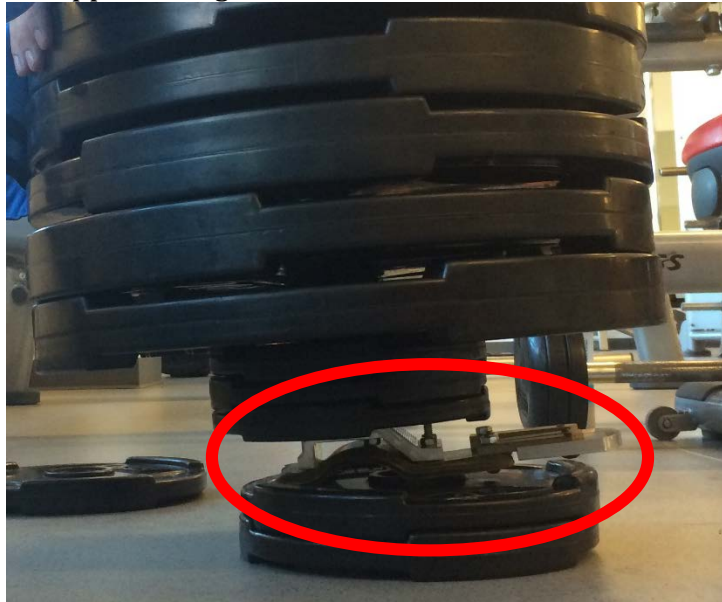
Figure 12: 40 Layer Foot with over 450lb. Applied
