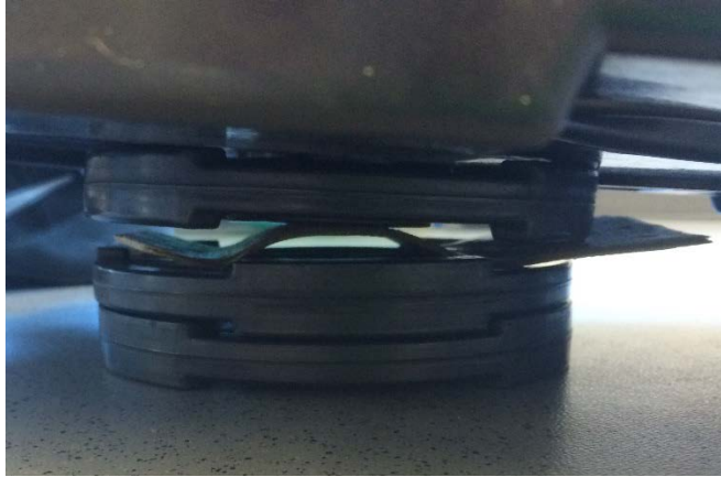
Figure 14: 8 Layer Foot with 225lb. Applied
