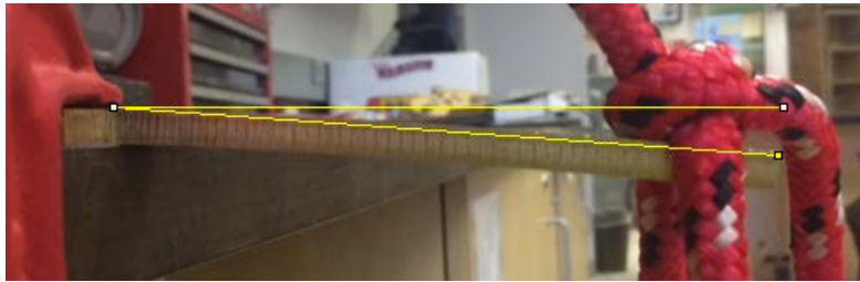
Figure 17: Thin Cantilever with 90lb. Applied
