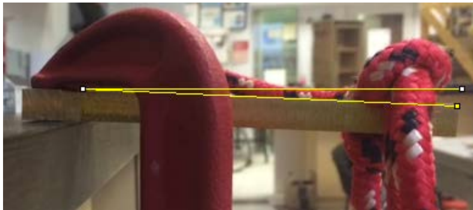
Figure 18: Thick Cantilever with 90lb. Applied
